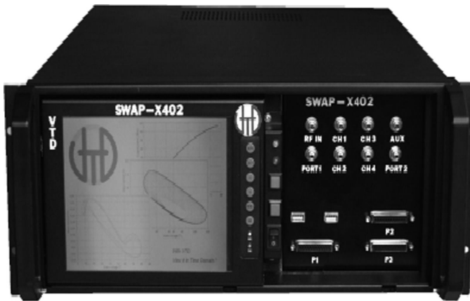
Figure 2.7 The SWAP, a new sampling-based NVNA with improved performance. (Reproduced with permission from VTD sas.)
