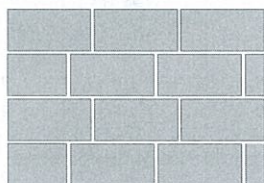
Running Bond or 1/2 Bond Standard Building Brick No Cutting Required
