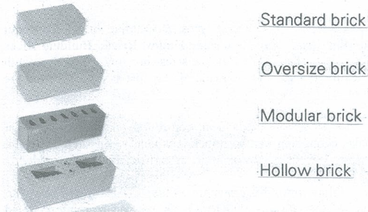
Figure 1. Building (common) brick. Standard size, available smooth or textured: Oversize, available smooth, wire cut or textured: Modular size, wire cut, smooth or textured.
