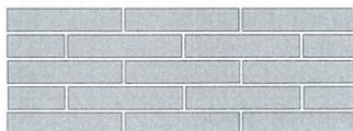
Running Bond or 1/2 Bond Norman Face Brick Oversize & Modular Building Brick Cut Corner Brick to Fit
