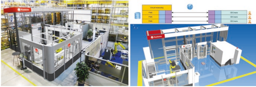
Fig. 3.1 The physical environment ( left ) and digital twin of it ( right )
