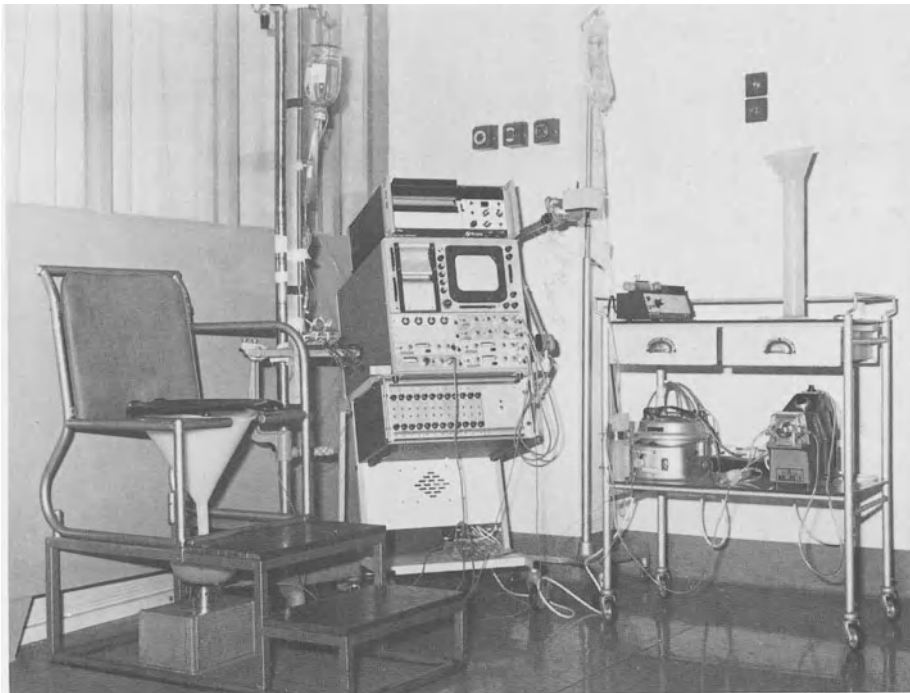
Fig. 6.3. A 12-channel urodynamic system for research studies.
