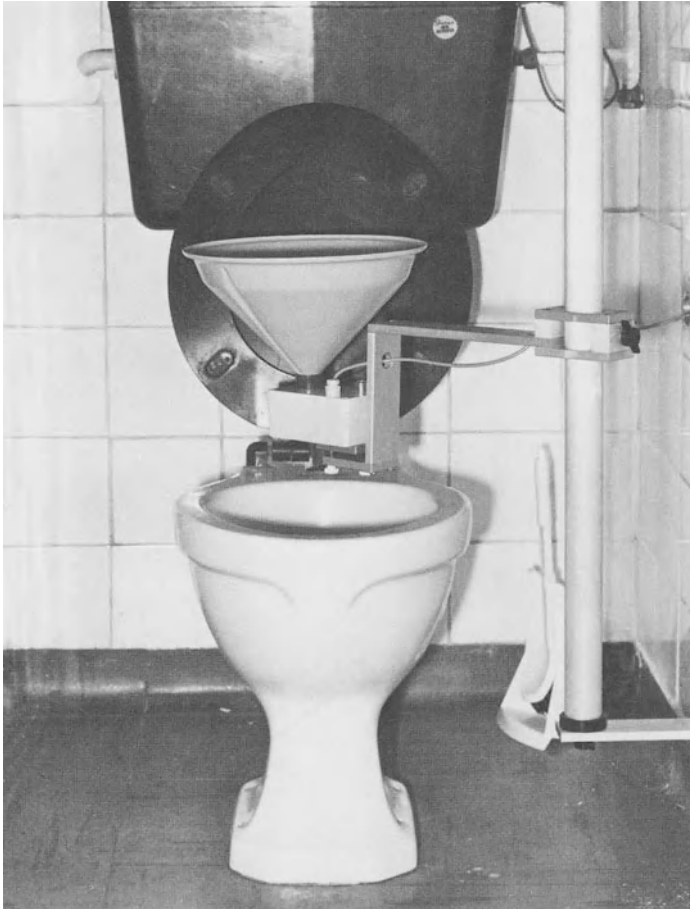
Fig. 6.4. An independent flowmeter installed in the ward toilet. This can be swung into use as necessary, the recording system being remote from the flowmeter. It can also be adjusted to go under a mobile commode. The recording system is activated when urine flows through the meter.
