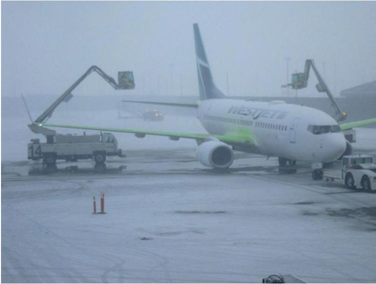
Fig. 4.1 De-icing airplanes in winter conditions (open source, Wikipedia/Steve torquay)
