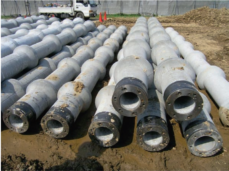
Fig. 14-33. Nodular piles with irregular surface
