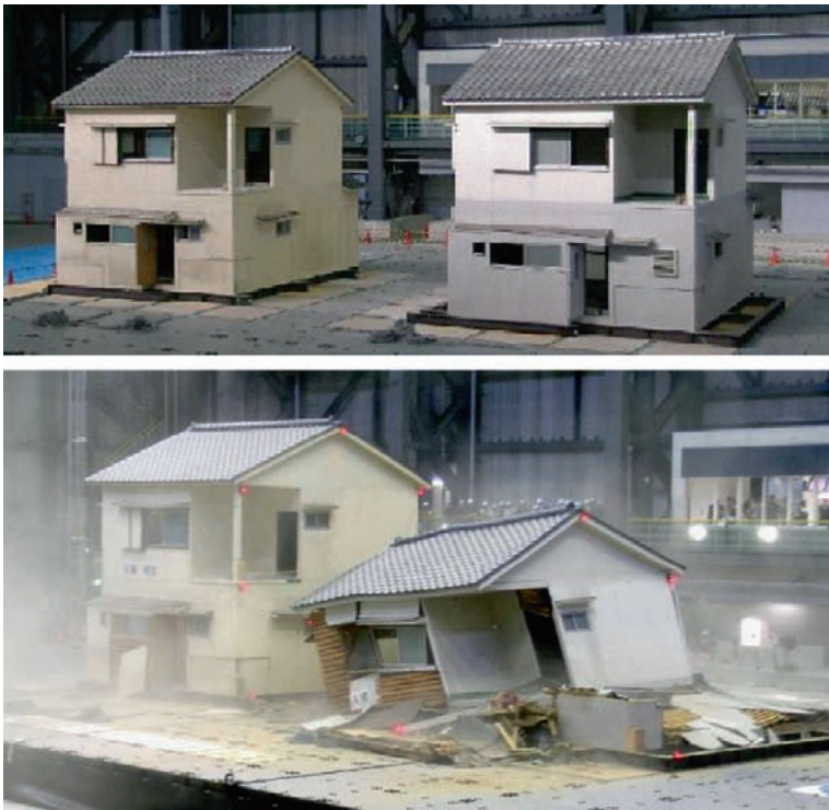
Fig. 10-11. Shaking table test of existing wooden houses (Right: not reinforced/ left: reinforced)
