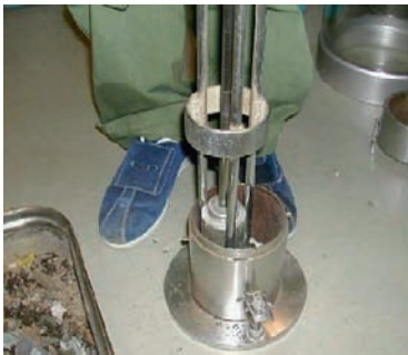
Fig. 14-19. Proctor compaction tests on organic waste
