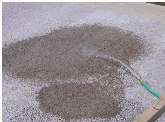
Figure 3-3 Demonstration of rapid infiltration, North Liberty, IA Source: John Kevern
