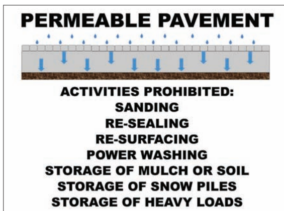
Figure 1-18 Recommended signage for maintenance staff Courtesy NCDENR
