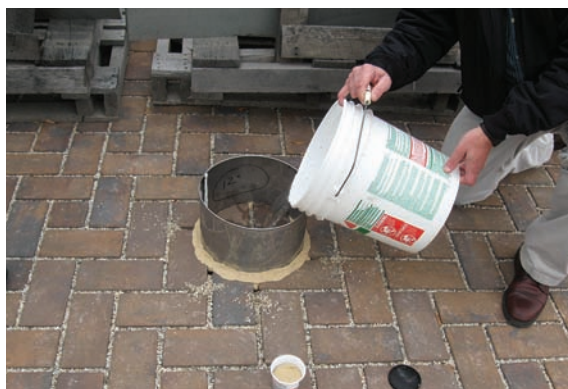
Figure 8-8 Inexpensive test apparatus for implementing ASTM C1701 and C1781 methods for assessing surface infiltration rates and cleaning needs for permeable pavements (PICP shown here)
