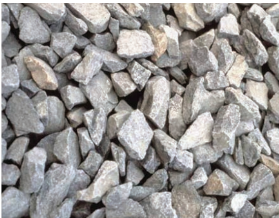
Figure 2-18 Clean, washed, crushed storage bed aggregate
