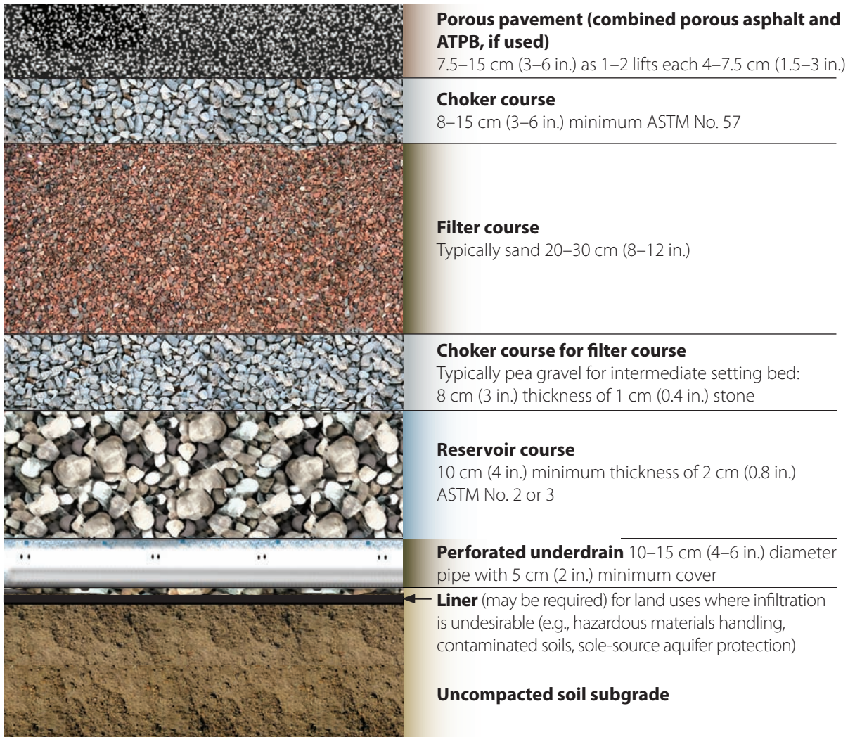
Figure 2-12 Porous asphalt section with filter course and capillary barrier for frost protection
