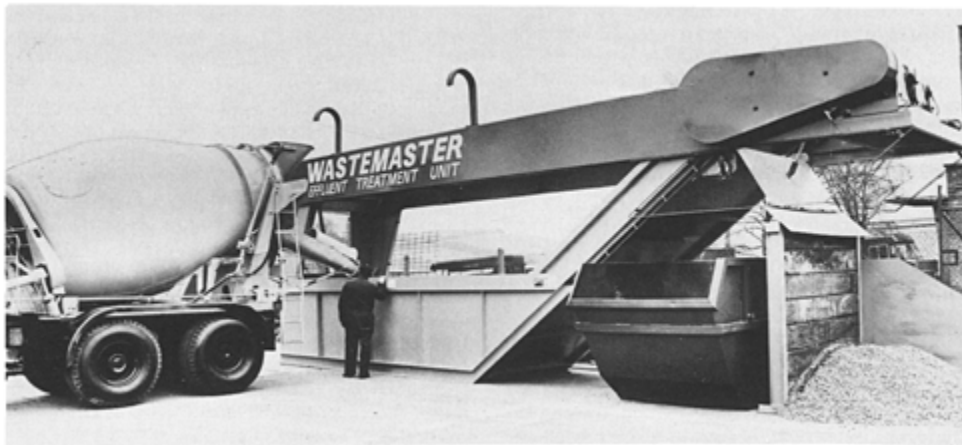
The effluent treatment unit which recycles the cleaning water forms a useful addition to the readymixed plant—four vehicles can be washed at a time and the aggregate re-used (except for quality concrete) (Batching Plant Limited)
