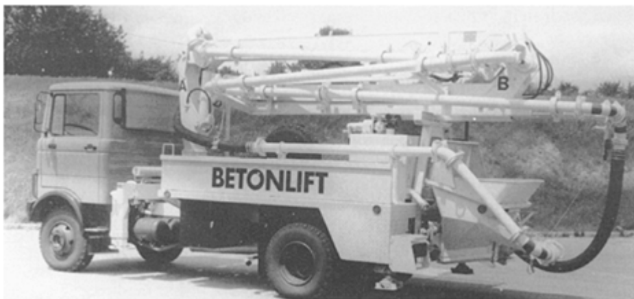
The plant which has revolutionised concrete placing—this typical piece of equipment can place more than 35 m 3 /hour through its 16 m long placing boom (Putzmeister)
