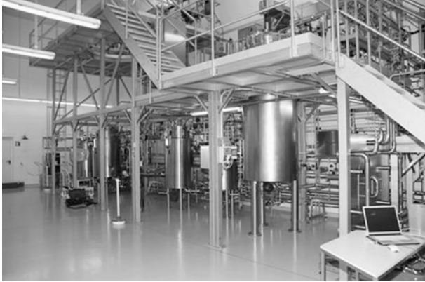
FIGURE 3.6 cGMP bioreactor cascade for plant cell suspension-based therapeutics production at Phyton Biotech.
