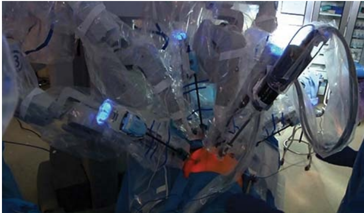
FIGURE 33-4 da Vinci SI docked for completion proctectomy with instruments in place.
