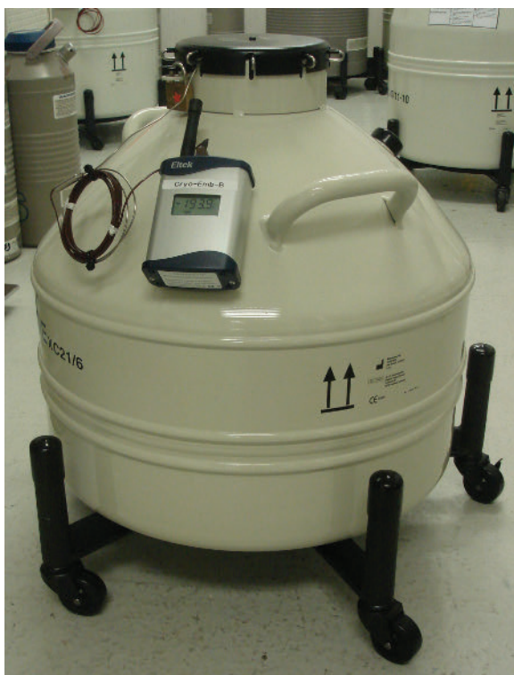
Figure 21.2 Sperm storage tank with a temperature probe which connects wirelessly to the laboratory monitoring system.
