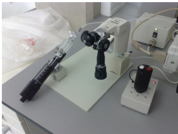
Figure 26.1 Controls on the left-hand side of the system. From left, injector control syringe, fine control unit for holding pipette and coarse control for holding pipette.
