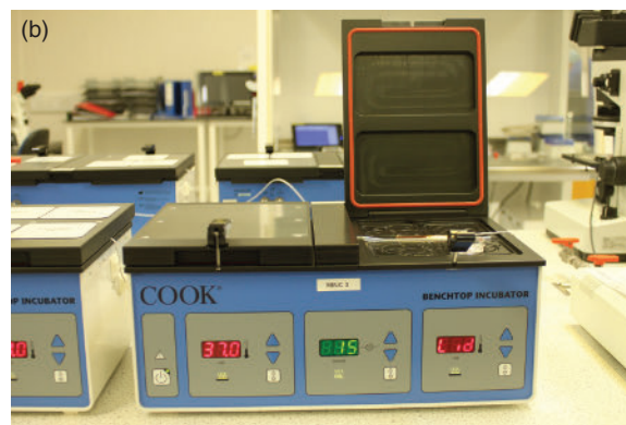
Figure 27.2 (a) Front loading, conventional type of incubator with individual inner doors. (b) Top loading, mini incubator showing small chamber for direct heat transfer.
