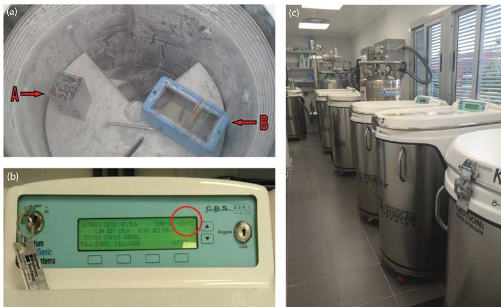
Figure 24.2 (a) Working area of the vapor tank showing a storage canister (A arrow) and the vitrification rack (B arrow) at the time of storing oocytes. (b) Display showing the temperature while manipulating the oocytes ( -184^{\circ}\text{C} ). (c) Storage room.
