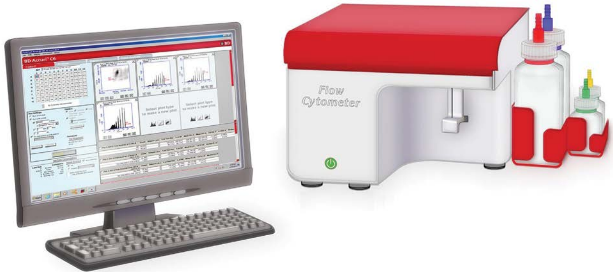
Figure 6.4 BD Accuri C6 flow cytometer.
