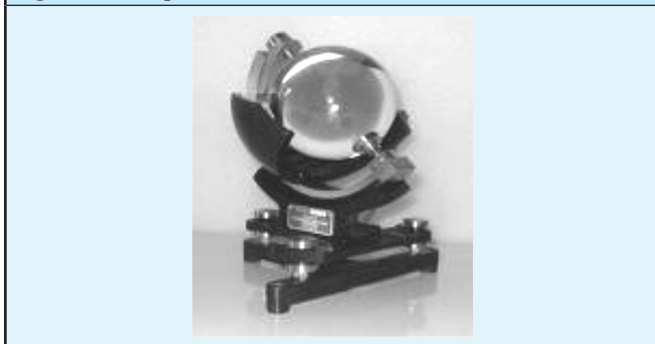
Fig. - 2 : Campbell-Stokes sunshine recorder
