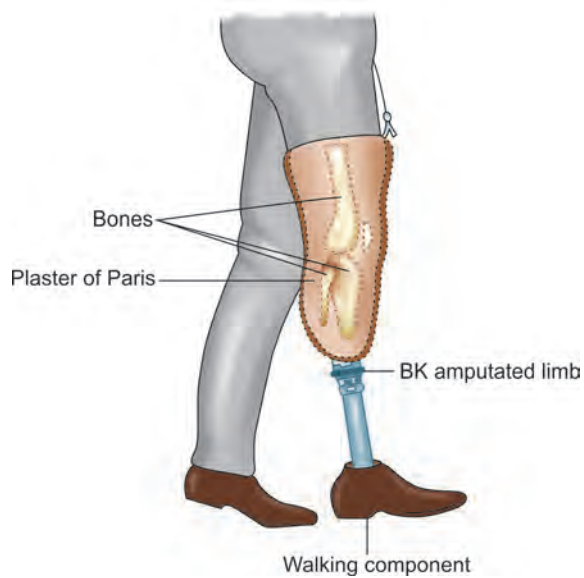
Fig. 1.579: Pylon is plaster cast with walking component used for immediate mobilisation after below-knee amputation.
