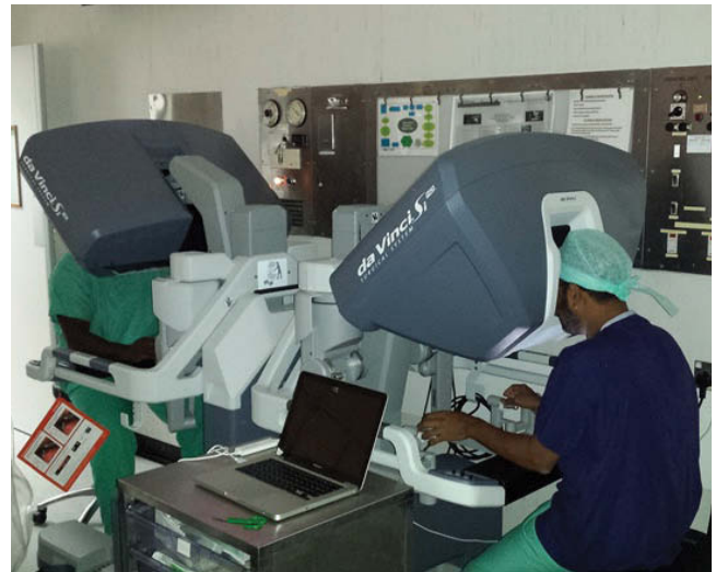
Figure 29.3 Photograph shows robotic surgery in progress, with dual surgical consoles. The two console surgeons share the same view and can swap control of the instruments, which facilitates training and allows rapid acquisition of skills.
