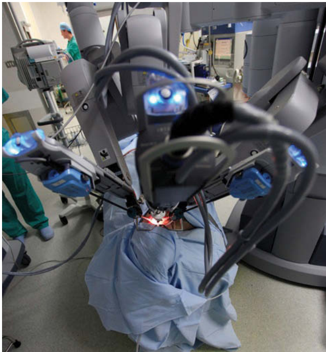
Figure 29.1 A bird's eye view of the da Vinci Si system docked in the mouth prior to TORS.
