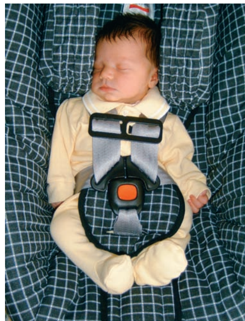
● Figure 26–13 Infant car restraint for use from birth to about 24 months of age.
