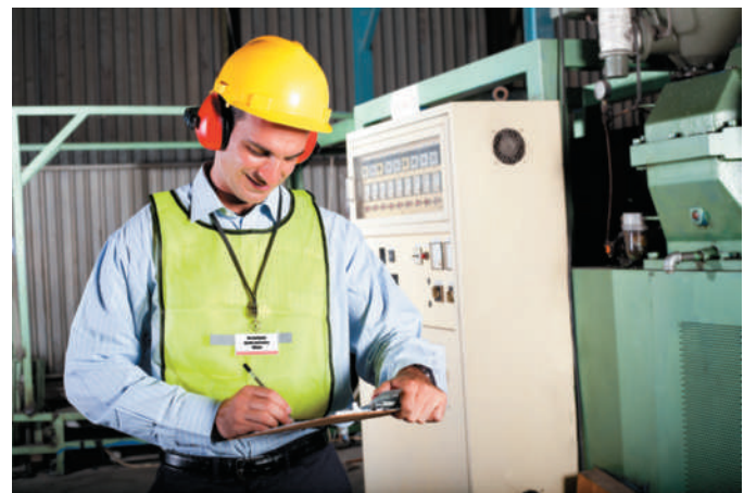
Use of hearing protection in high-noise areas can prevent hearing loss. (Michaeljung/Fotolia)
