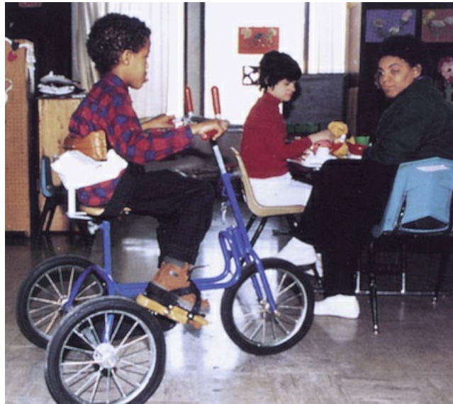
FIG 17-4 A modified tricycle with block pedals, self-adhesive straps for support, and a modified seat and handle bars can help a child with disabilities gain mobility.
