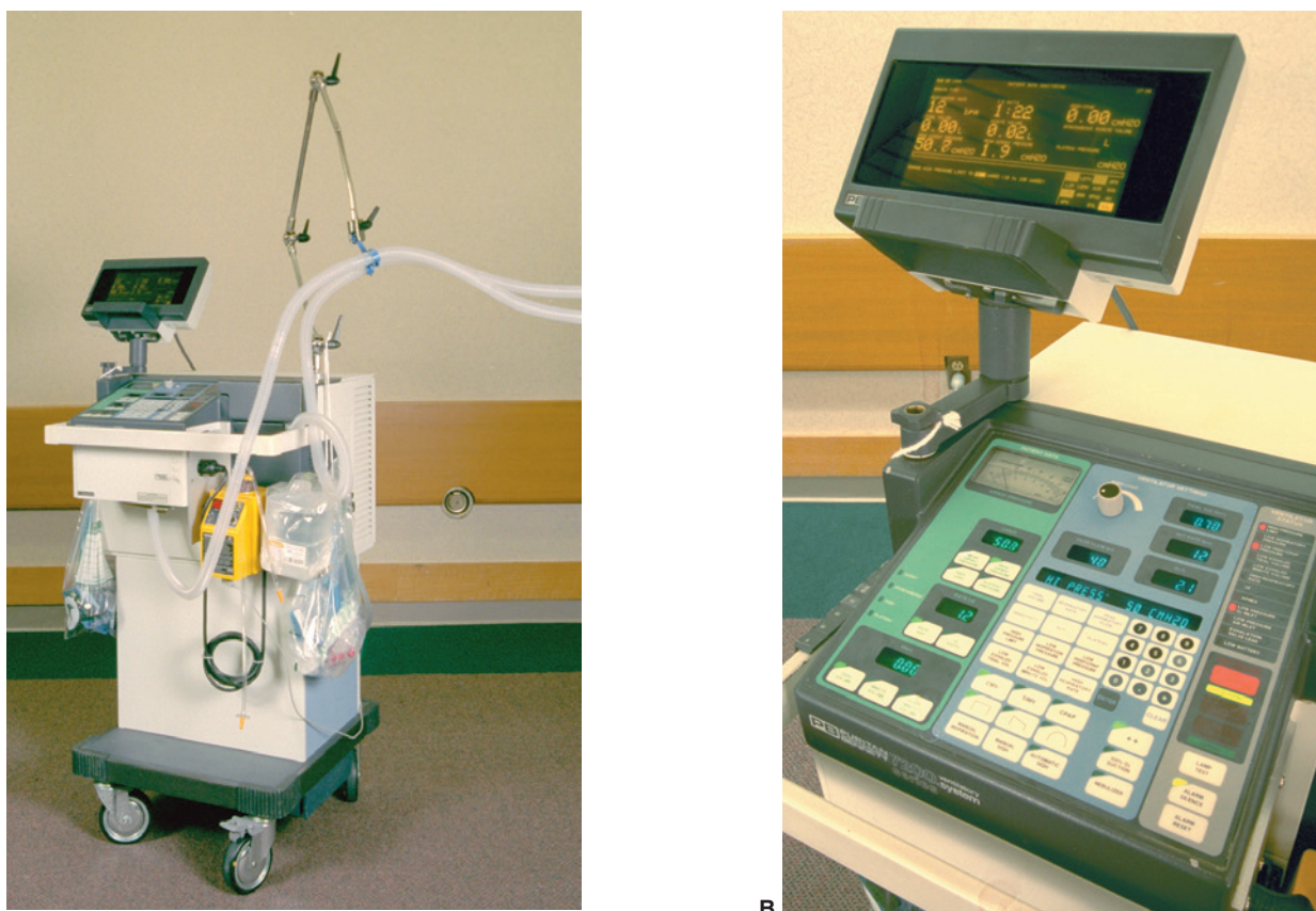
FIGURE 36.14 ■ A , Positive-pressure ventilator. B , Control panel used to set the mode, rate, limits and percentage of oxygen delivered
