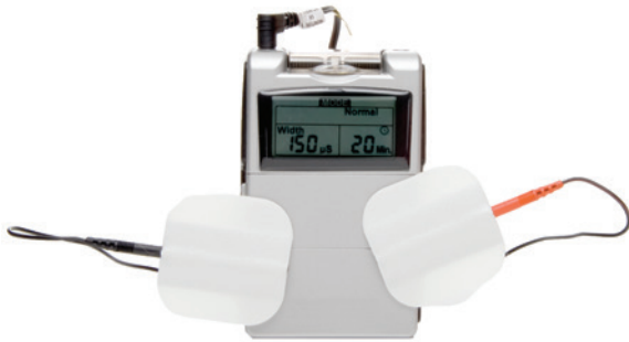
FIGURE 8.5 ■ The TENS unit is believed to assist in pain management in the ways described in the gate-control theory. Electrodes that deliver low-voltage electrical stimuli are placed directly on the person over painful areas
