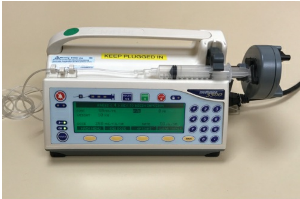
Figure 38.7 An infusion pump and calibrated infusion chamber are safety features used with children's intravenous infusions.
