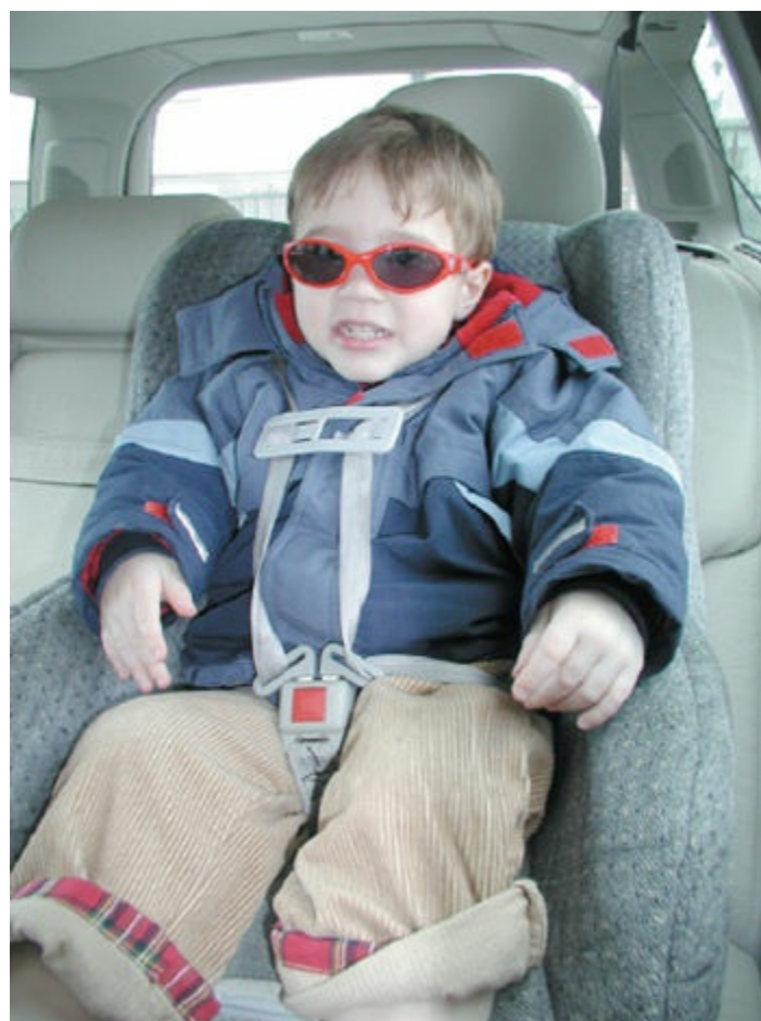
Figure 30.5 Toddlers should use a car seat with a five-point restraint while riding in an automobile until they are 2 years of age.
