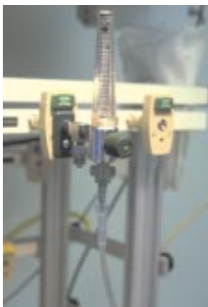
Figure 7-1-2B In-line oxygen and flow meter
