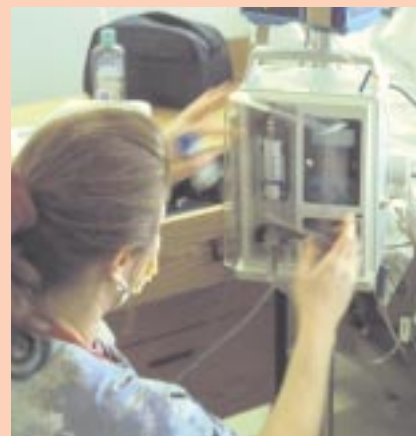
Figure 5-21-5 Check for any leaking or damage to the system, and close the door to the chamber.
