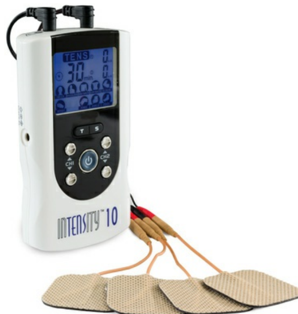
FIG. 4-5 TENS unit used in the home by the patient. (Courtesy Compass Health Brands, Middleburg Heights, Ohio.)
