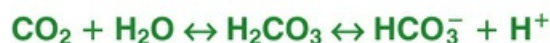
FIG. 12-7 The carbonic anhydrase equation showing that the concentration of carbon dioxide is directly related to the concentration of hydrogen ions.
