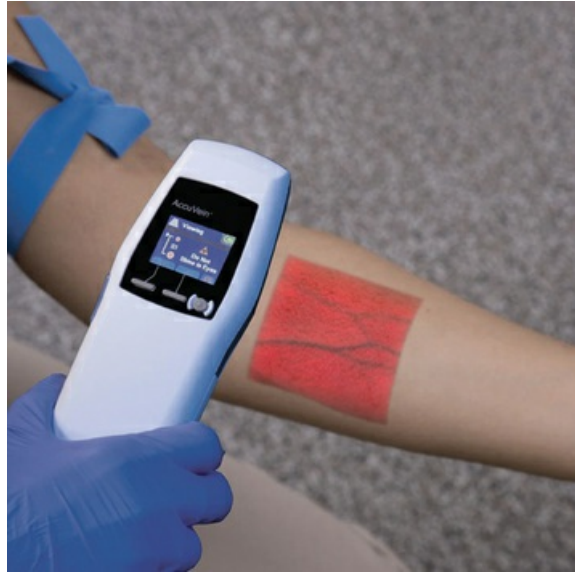
FIG. 13-3 The AccuVein AV300 is a vein illumination device that helps health care professionals locate veins for blood draw, IV infusion, and blood donation by projecting a pattern of light on the patient's skin to reveal the position of underlying veins on the skin's surface. The device uses red and infrared light, which the hemoglobin in blood absorbs to detect the position of the vein. (Courtesy AccuVein, LLC.)
