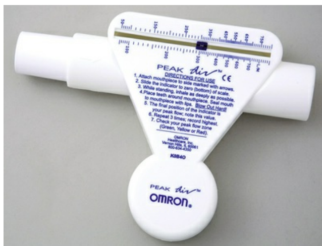
FIG. 30-4 Typical peak flow meter. This model will show faster exhalation rates in green , reduced exhalation rates in yellow , and seriously reduced exhalation rates in red . (From Aehlert, B. [2011]. Paramedic practice today: Above and beyond . St. Louis: Mosby.)
