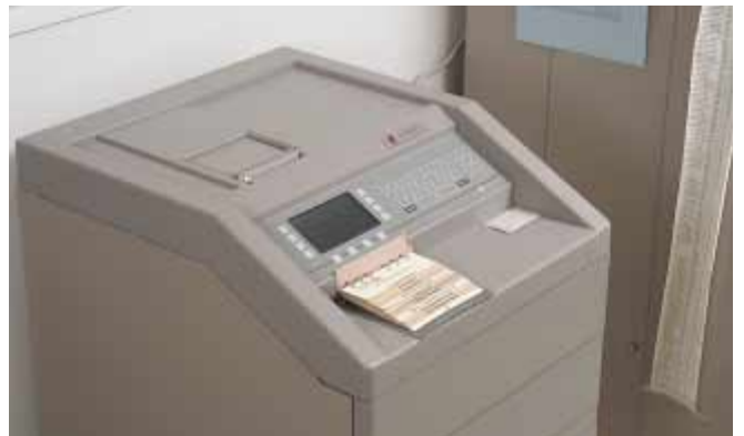
Figure 29-6 Computer-controlled Dispensing System
