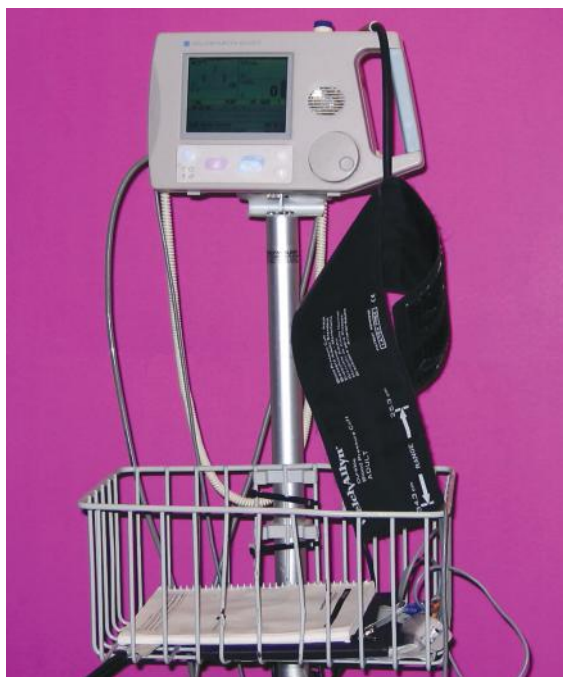
Fig 11.6b Electronic sphygmomanometer. (From Wilkinson and Treas [2011]. Fundamentals of nursing , Vol. 1, 2nd ed. Philadelphia: F. A. Davis Company, with permission.)
