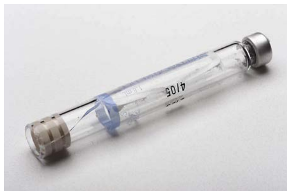
• Fig. 7.12 Cracked glass on dental cartridge.
