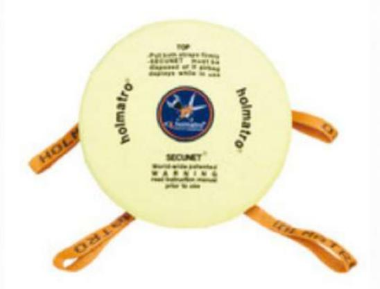
Airbag covers are placed over un-deployed airbags. An airbag may deploy unexpectedly during a rescue even if the battery has been disconnected and cause serious harm to the patient or rescuer.
