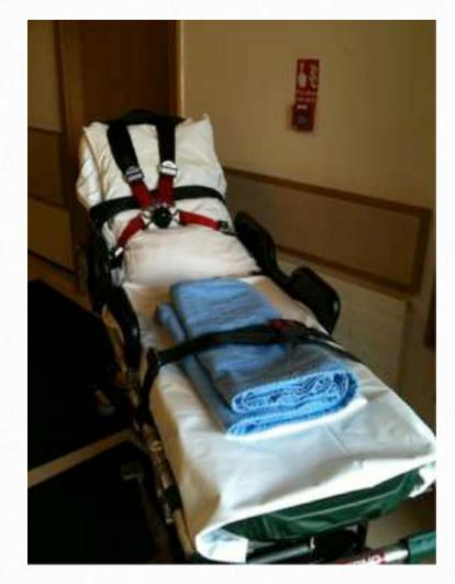
An ambulance trolley with a Ferno® 5 point safety harness seatbelt. These seatbelts are tested to 10G in 6 directions.
