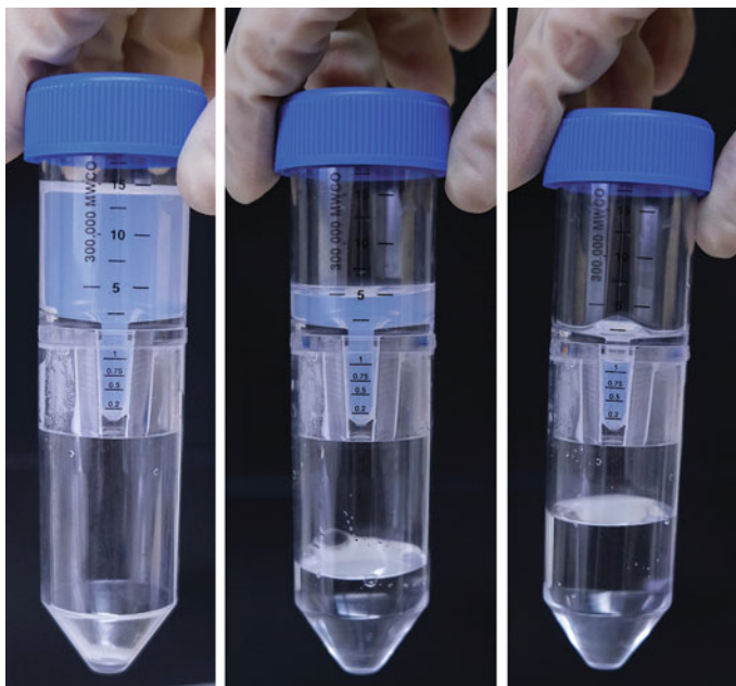
Fig. 2 130 nm glucan nanoparticle centrifugation using Vivaspin 20 centrifugal concentrator (MWCO 300KD): the nanoparticle suspension is being concentrated in the upper part of the tube (white suspension), while the bottom contains the filtrate (with no color associated)
