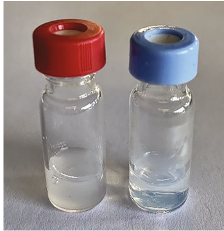
Fig. 5 The non-extruded (red cap) liposome solution is cloudier than the extruded solution (blue cap)
