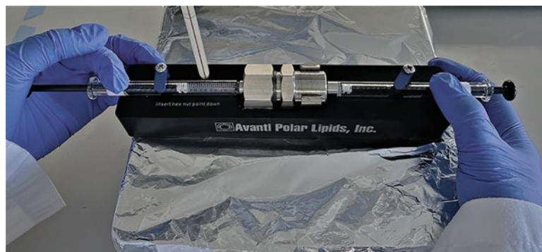
Fig. 4 The correct position to perform the extrusion when pushing the plunger of the loaded syringe
