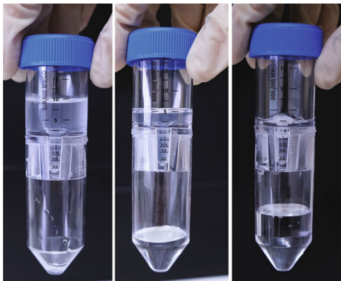
Fig. 4 350 nm glucan nanoparticle centrifugation using Vivaspin 20 centrifugal concentrator (MWCO 300KD): the nanoparticle suspension is being concentrated in the upper part of the tube (transparent suspension), while the bottom contains the filtrate
