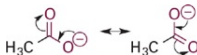
Figure 5.10 Resonance structures of acetate anion showing equal distribution of negative charge on the two oxygen atoms.
