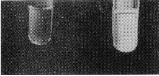
Fig. 24 The liquid crystal is radiant between crossed polarizers (right), whereas an isotropic solution (left) appears black.
