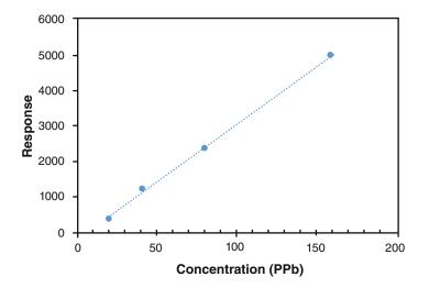
Fig. 2 Malathion linearity over the concentration range of 20-160 ppb
