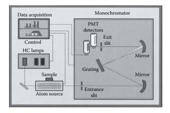
**FIGURE 6.32** The AtomSource glow discharge atomizer incorporated into an analyzer for solid metals and metal alloys (the pulsar system). (Courtesy of Teledyne Leeman Labs, Inc., Hudson, NH (www.teledyneleemanlabs.com].)
