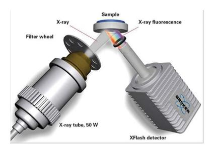
**FIGURE 8.15** Schematic 3D view of a direct excitation EDXRF system. (© 2020 Bruker, Inc. [www.bruker.com]. Used with permission.)
