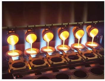
**FIGURE 1.5** (a) Platinum crucibles and molds used for fusion, along with some finished glassy sample disks, used for XRF analyses. (b) An automated fusion machine pouring multiple molten samples into platinum molds. (Courtesy of XRF Scientific, Perth, Australia, www.xrfscientific.com. Used with permission.)
