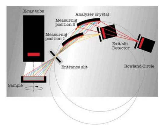
**FIGURE 8.43** Rowland circle type monochromator schematic with a Johansson curved crystal used as a scanning channel. (© 2020 Bruker, Inc. [www.bruker.com]. Used with permission.)
