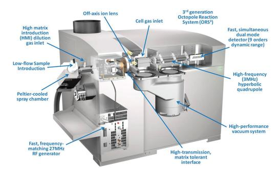
**FIGURE 9.32** Cutaway view of the single quadrupole 7700-series benchtop ICP-MS from Agilent Technologies. The hyperbolic quadrupole is shown between the reaction cell and the detector. The sample introduction system and ICP torch are on the left of the diagram. (© 2018 Agilent Technologies [www.agilent.com/chem]. All rights reserved. Used with permission.)
