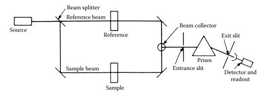
FIGURE 2.27 Schematic diagram of a double-beam optical system.
