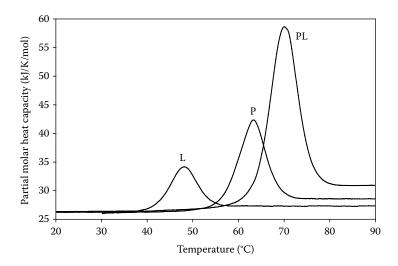
**FIGURE 14.38** Simulated DSC data showing the higher temperature stability of a tightly-associated protein/ligand complex (PL) compared with the free protein (P) and ligand (L). (Courtesy of TA instruments, New Castle, DE. www.tainstruments.com.)
