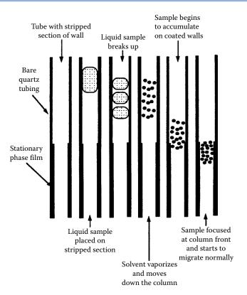
**FIGURE 11.11** Illustration of on-column injection with a retention gap. (Cazes, used with permission.)
