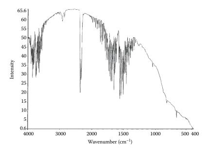
**FIGURE 4.14** A background spectrum of air, showing the absorption bands due to water vapor and carbon dioxide. (Collected on a paragon 1000 FTIR spectrometer, ©2020 PerkinElmer, inc. All rights reserved. Printed with permission.)
