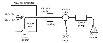
**FIGURE 9.14** Schematic of continuous flow FAB-MS operated in the flow-injection mode.
