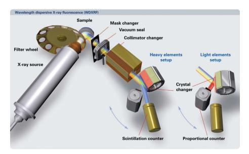
**FIGURE 8.32** Schematic commercial WDXRF system showing the position of a collimator mask changer, as well as the layout of X-ray tube, filter wheel, sample, collimator, analyzing crystal changer, and detector. (© 2020 Bruker, Inc. [www.bruker.com]. Used with permission.)
