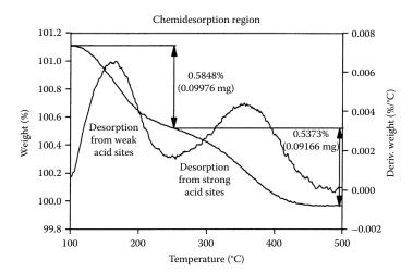
**FIGURE 14.13** TGA and DTG thermal curves showing desorption of basic compounds from the acidic sites of a zeolite catalyst. Losses from weakly acidic sites can be distinguished from strongly acidic sites using the DTG curve, despite the fact that the overall mass loss is only about 1 %. The mass scale is on the left *y*-axis. (Courtesy of TA instruments, New Castle, from thermal analysis applications brief TA-231. www.tainstruments.com.)
