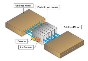
Figure 1. Illustration of Folded Flight Path technology.
