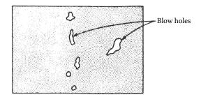
FIGURE 8.60 Schematic X-ray absorption photograph of a mechanical weld.
