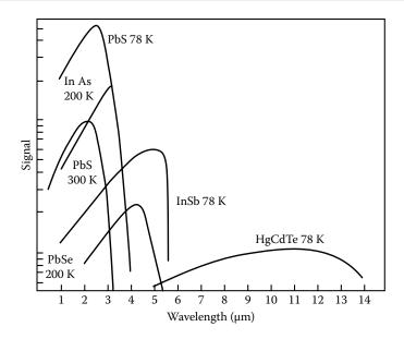
**FIGURE 4.15** Spectral response of various semiconductor detectors. The operating temperature in kelvin is given next to the material.
