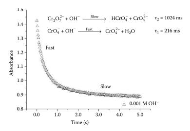
**FIGURE 3.37** Measurement of the fast and slow steps in the oxidation of dichromate ion by spectroscopy using a rapid mix accessory. (© Thermo Fisher Scientific [www.thermofisher.com]. Used with permission.)
