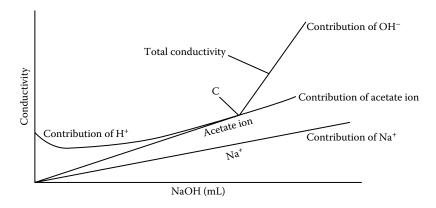
**FIGURE 13.24** Solution conductivity during an acetic acid (CH<sub>3</sub>COOH)–NaOH titration. Point C is the neutralization point.
