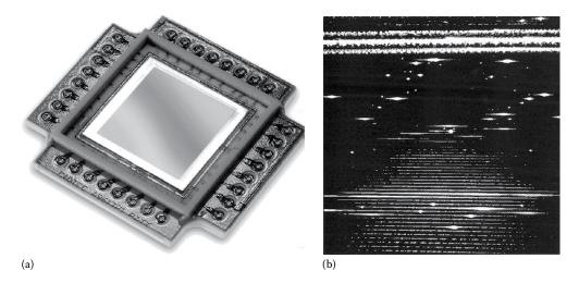
**FIGURE 7.17** (a) Photograph of a CID. This solid-state array detector captures an electronic image of the complete emission spectrum. (b) The Echellogram of a sample of zinc oxide collected by a CID detector from a DC arc source. (© Thermo Fisher Scientific [www.thermofisher.com]. Used with permission.)
