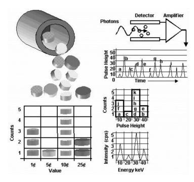
**FIGURE 8.26** Schematic of the pulse processing of a multichannel analyzer. Left side: the "coins" (photons) are separated by denomination and binned. Right side, second from the bottom: the number of coins gives a "stack height" (counts). The typical EDXRF output is the lower right plot of intensity (counts per second) versus energy.
