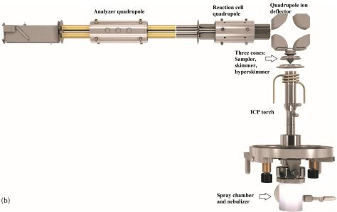
**FIGURE 9.52** (a) Schematic diagram of an ICP-MS system with a quadrupole mass analyzer. (b) NexION 300 ICP-MS showing its three quadrupoles, three cones and the ICP torch, and sample introduction system. (© 1993-2020 PerkinElmer, inc. All rights reserved. Printed with permission. [www.perkinelmer.com].)
