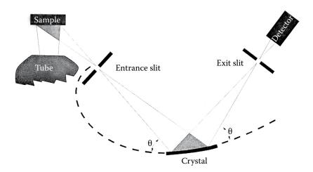
**FIGURE 8.35** Schematic of the optical path in a curved crystal spectrometer. (Courtesy of Malvern Panalytical Inc., Almelo, the Netherlands [www.malvernpanalytical.com]. Used with permission.)
