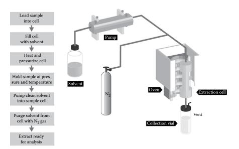
**FIGURE 1.6** Accelerated solvent extraction technique. (© Thermo Fisher Scientific (www.thermofisher.com). Used with permission.)
