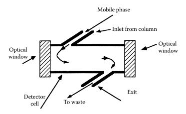
**FIGURE 12.14** Diagram of HPLC UV/VIS detector flow cell. (Scott, used with permission.)
