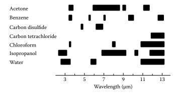
**FIGURE 4.18** IR absorption characteristics of some common solvents. Regions of strong IR absorbance in 0.1 mm cells (except water, 0.01 mm cell) are shown as shaded areas. Longer cell paths will broaden the regions of absorption and in some cases introduce new regions where absorption is significant. (Reprinted from Aikens et al. By permission from Waveland Press, Inc. Long Grove, IL, 1984. All rights reserved.)
