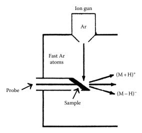
**FIGURE 9.13** Schematic FAB ionization source. The sample, dissolved in solvent, is spread on a thin film on the end of a metal probe and bombarded by fast-moving argon atoms. Both positive and negative ions are produced.
