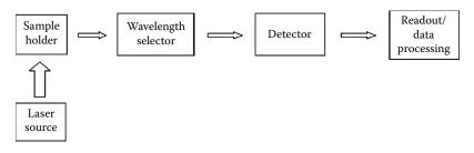
**FIGURE 4.40** Idealized layout of a Raman spectrometer.
