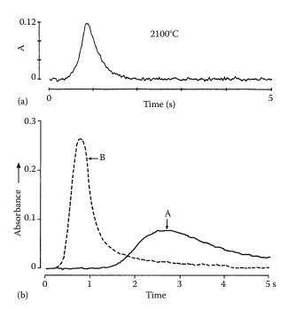
**FIGURE 6.19** (a) An ideal Gaussian-shaped atomization signal from a graphite furnace. (b) Atomization signals for molybdenum in a graphite furnace atomizer. (a) is the signal resulting from an uncoated graphite tube atomizer. (b) is the signal from a graphite tube coated with pyrolytic graphite. (© 1993-2020 PerkinElmer, inc. All rights reserved. Printed with permission. [www.perkinelmer.com].)
