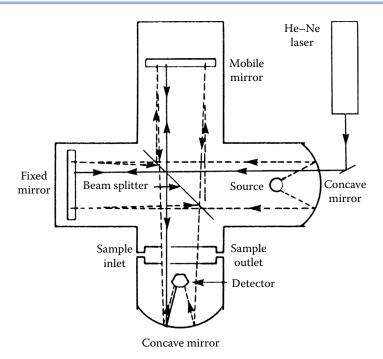
**FIGURE 2.30** Schematic of a Michelson interferometer-based FTIR spectrometer.
