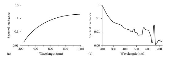
**FIGURE 3.14** (a) Emission spectrum of a commercial tungsten-halogen lamp. (b) Emission spectrum of a commercial deuterium arc lamp. (© 2020 Agilent Technologies, Inc. [www.agilent.com]).
