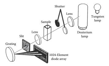
**FIGURE 3.25** Optical diagram of a diode array spectrophotometer, showing both UV and visible light sources and a 1024 element PDA detector. (© 2020 Agilent Technologies, Inc. [www.agilent.com]).
