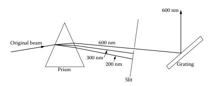
FIGURE 2.18 Prism used as an order sorter for a grating monochromator.
