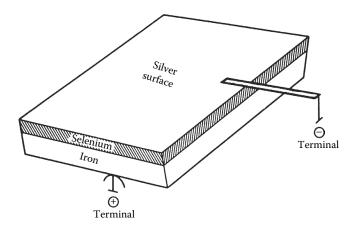
FIGURE 3.17 Barrier layer cell.
