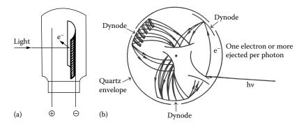
**FIGURE 3.18** (a) A vacuum phototube. (b) Schematic of a PMT, looking down through the tube. Impinging photons pass through the quartz envelope and liberate electrons from the light-sensitive cathode. The electrons are accelerated to the first dynode, where each electron liberates several electrons on impact. The process is repeated at the other dynodes, resulting in a cascade of electrons for every photon hitting the PMT.
