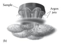
**FIGURE 6.31** (a) The AtomSource glow discharge atomizer for conductive solid samples. (b) Schematic of the sputtered atom cloud produced by bombardment of the sample surface by ionized argon. (Courtesy of Teledyne Leeman Labs, Inc., Hudson, NH (www.teledyneleemanlabs.com].)
