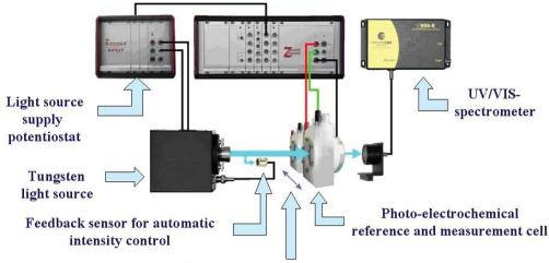
Actuator for automatic change between reference and measurement cell
