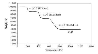
**FIGURE 14.6** TGA thermal curve of calcium oxalate monohydrate,  $CaC_2O_4 \cdot H_2O$ .
