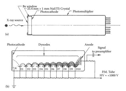
**FIGURE 8.40** Schematic NaI(TI) scintillation detector. **(a)** The assembled detector. **(b)** Schematic representation of the photomultiplier and its circuitry. (Courtesy of ORTEC [Ametek], www.ortec-online.com from Jenkins et al., 1981, Used with permission.)
