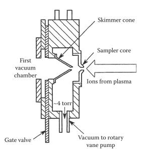
**FIGURE 9.53** Close-up of an ICP-MS interface, showing the sampler and skimmer cones. (© 1993-2020 PerkinElmer, inc. All rights reserved. Printed with permission. [www.perkinelmer.com].)
