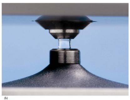
**FIGURE 3.33** (a) 0.5 μL sample pipetted onto the measurement surface of the NanoDrop™ 2000c. (b) Cuvette-less sample column formed between the pedestals by closing the cover. (© Thermo Fisher Scientific [www.thermofisher.com]. Used with permission.)
