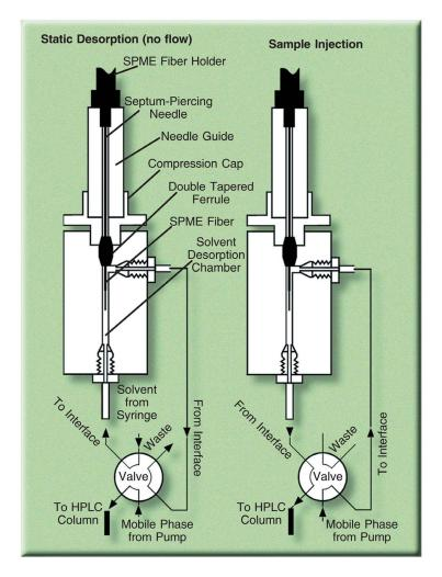
**FIGURE 1.11** A SPME-HPLC interface. (Used with permission from Sigma-Aldrich, a part of MilliporeSigma. www.sigmaaldritch.Com. Copyright 2020 Sigma-Aldrich Co. LLC. All rights reserved.)
