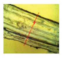
**FIGURE 4.25** Micrograph of a polymer laminate, showing two broad layers and a narrow middle layer. The sample was mounted in a NaCl compression cell and spectra were collected automatically in 2  $\mu$ m steps along the line indicated. A Centaur $\mu$ s analytical FTIR microscope system was used for the automatic data collection and results. (© Thermo Fisher Scientific [www.thermofisher.com]. Used with permission.)
