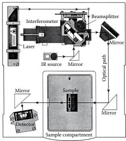
**FIGURE 4.10** (Top) Schematic diagram of a Michelson interferometer. ZPD stands for zero path-length difference (i.e., the fixed mirror and moving mirror are equidistant from the beam splitter). (From Coates, used with permission). (Bottom) A simple commercial FTIR spectrometer layout showing the He-Ne laser, optics, the source, interferometer, sample, and detector. (© Thermo Fisher Scientific [www.thermofisher.com]. Used with permission.)
