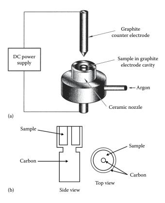
**FIGURE 7.6 (a)** Diagram of a direct current arc source. The solid sample is packed into the cupped end of the lower graphite electrode. The graphite counterelectrode is also shown. (From Hareland, used with permission.) **(b)** A schematic of the lower electrode used to hold the sample.
