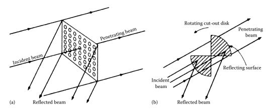
**FIGURE 2.28** (a) Plate beam splitter. (b) Rotating disk beam splitter (or *chopper*).
