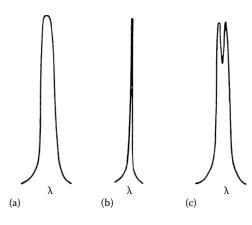
FIGURE 6.28 Distortion of spectral line shape in an HCL due to self-reversal. (a) Shape of the spectral line emitted by the HCL. (b) Shape of the spectral energy band absorbed by cool atoms inside the HCL. (c) Shape of the net signal emerging from an HCL, showing self-absorption of the center of the emission band.
