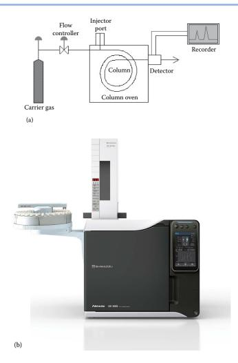
**FIGURE 10.2** (a) A schematic gas chromatography instrument, showing carrier gas, column, oven, injection port and detector. (b) A modern GC instrument with autosampler, the Shimadzu GC-2030. [(b) Courtesy of Shimadzu Corporation, Kyoto, Japan, www.ssi.shimadzu.com.] Details of the instrumentation will be discussed in Chapter 11.
