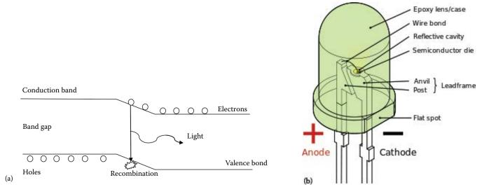
FIGURE 3.15 (a) Light production by recombination of an electron and hole in an LED. (b) Schematic of an LED.
