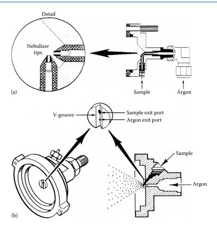
**FIGURE 7.31** (a) A cross-flow nebulizer, with a close-up of the nebulizer tips. (b) A V-groove nebulizer. (© 1999-2020 PerkinElmer, inc. All rights reserved. Printed with permission. [www.perkinelmer.com].)
