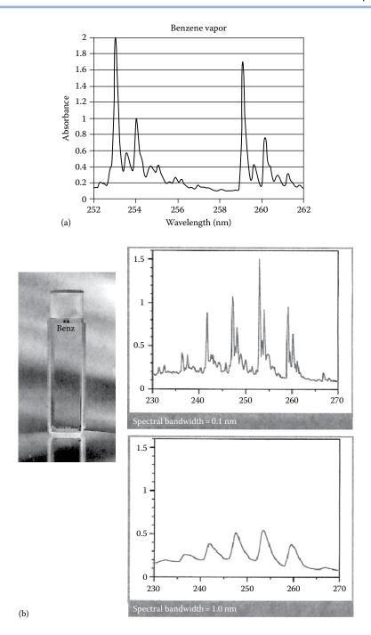
**FIGURE 2.21** (a) Spectrum of benzene vapor. (b) Spectra of benzene vapor taken at two different bandwidths for testing resolution of a grating-based instrument. (Courtesy of Starna Cells, Inc. Atascadero, CA [www.starnacells.com].)
