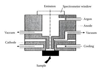
**FIGURE 7.43** A DC GD source. A flat conducting sample serves as part of the cathode. (Courtesy of HORIBA Scientific. © 2020 HORIBA Scientific [www.horiba.com/scientific]. All rights reserved.)
