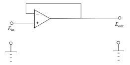
**FIGURE 13.13** Schematic of an operational amplifier (called an op-amp) with voltage feedback (the voltage follower).
