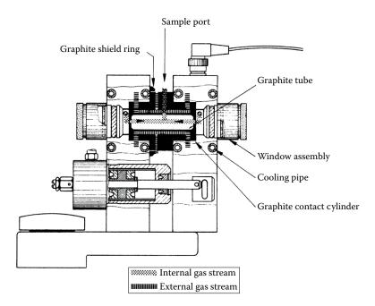
**FIGURE 6.11** Graphite furnace atomizer. This is a longitudinally heated furnace design. The graphite tube is shown in greater detail in figure 6.21. (© 1993-2020 PerkinElmer, inc. All rights reserved. Printed with permission. [www.perkinelmer.com].)
