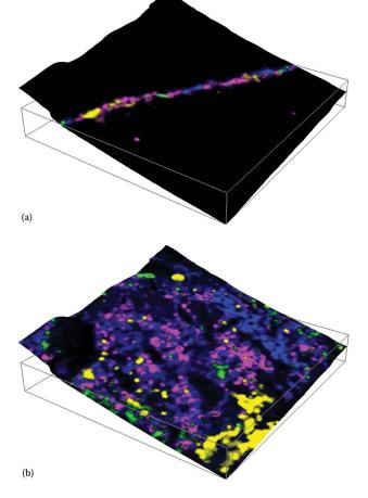
**FIGURE 4.61** (a) Field of view of a Confocal Raman Imaging measurement without correcting for the topography. (b) True Surface Raman image as a result of the height profile overlaid with the topography-traced confocal Raman image. (Courtesy of Frances Westall, CNRS Orleans, France and WITec GmbH, Ulm, Germany. www.WITec.de. Used with permission.)
