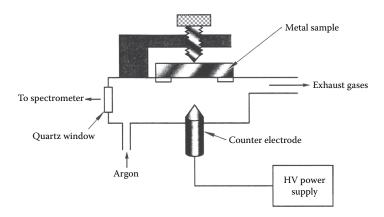
**FIGURE 7.10** A schematic spark source, showing a flat metal sample as the cathode and a tungsten counterelectrode as anode. (From Hareland, used with permission.)
