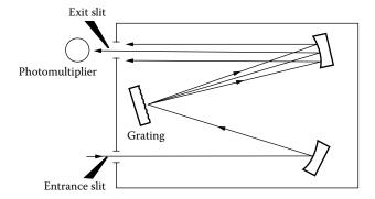
**FIGURE 6.13** Typical grating monochromator layout. (© 1993-2020 PerkinElmer, inc. All rights reserved. Printed with permission. [www.perkinelmer.com].)
