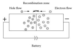
**FIGURE 3.22** A p-n junction under forward bias. The positive battery terminal is connected to the p side.
