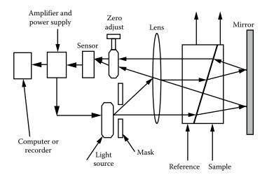
**FIGURE 12.11** Schematic diagram of differential refractive index detector. (Katz et al., Used with permission.)
