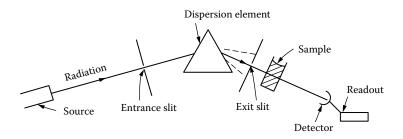
**FIGURE 2.13** Schematic diagram of a single-beam absorption spectrometer.
