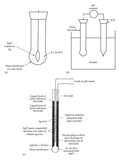
**FIGURE 13.7** (a) A schematic glass electrode for pH measurement. (b) A complete pH measurement cell, with the glass indicator electrode and an external saturated calomel reference electrode. (c) A commercial combination pH electrode, with built-in internal Ag/AgCl reference electrode.
