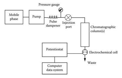
**FIGURE 12.16** A schematic of an HPLC system with electrochemical detection.
