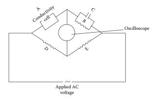
FIGURE 13.22 Wheatstone bridge arrangement for conductometric analysis.
