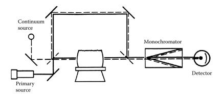
**FIGURE 6.26** Continuum background corrector in a double-beam AAS system. (© 1993-2020 PerkinElmer, inc. All rights reserved. Printed with permission. [www.perkinelmer.com].)
