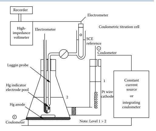
**FIGURE 13.21** Apparatus for coulometric titration with potentiometric endpoint detection.
