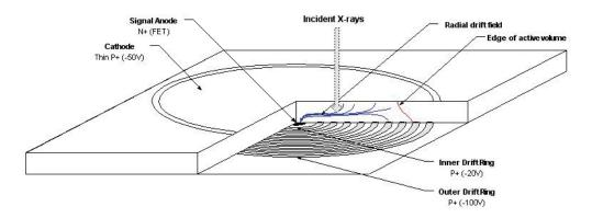
**FIGURE 8.25** Schematic of a silicon drift detector. (Courtesy of Amptek, Inc. www.amptek. com.)
