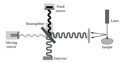
**FIGURE 4.42** Schematic of an FT-Raman spectrometer. (Reprinted from Weesner and Longmire, with permission from Advanstar Communications, Inc.)
