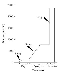
**FIGURE 6.18** Typical temperature program for a graphite furnace atomizer. (© 1993-2020 PerkinElmer, inc. All rights reserved. Printed with permission. [www.perkinelmer.com].)
