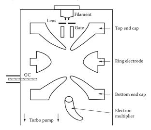
**FIGURE 9.34** Cross-section of a quadrupole ion trap mass spectrometer. This schematic shows a gas phase sample introduced from a GC and ionized inside the trap by electrons from the filament. (From Niessen and Van Der Greef, used with permission.)
