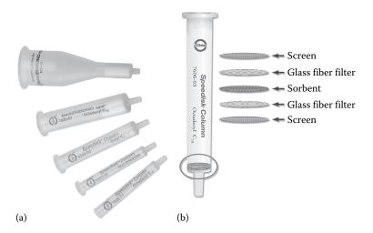
**FIGURE 1.8 (a)** Commercial plastic syringe-type cartridges and **(b)** Schematic of sorbent packing. (Permission to reprint from Avantor Performance Materials, Inc., Center Valley, PA. www.avantormaterials.com.)
