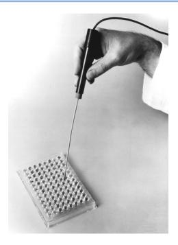
**FIGURE 13.8** A commercial microelectrode for pH measurements in volumes as small as  $10 \, \mu L$ . The electrode has a solid-state pH sensor and a flexible polypropylene stem, making it extremely rugged and suitable for use in the field. This electrode can be used to determine pH in single droplets of water on leaves of plants or blades of grass to study acid rain deposition. (Courtesy of Lazar Research Laboratories, Inc., Los Angeles, CA [www.lazarlab.com].)
