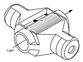
**FIGURE 6.12** A graphite tube for a transversely heated furnace. (© 1993-2020 PerkinElmer, inc. All rights reserved. Printed with permission. [www.perkinelmer.com].)
