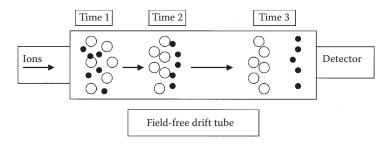
**FIGURE 9.25** A pulse of ions of two different m/z values enters the field free drift tube of a TOF mass spectrometer at time one. The large white circles have m/z > than the small dark circles. As they travel down the tube, the lighter ions move faster, and by time three, have been separated from the heavier ions.
