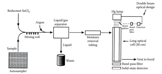
FIGURE 6.33 Automated cold vapor mercury analyzer. Mercury in the sample is reduced to Hg. The Hg vapor is separated from the solution by a gas-liquid separator and carried to the optical cell. The Hg vapor absorbs the 253.7 nm emission line from the Hg lamp and the amount of atomic absorption is measured using a solid-state detector. (Courtesy of Teledyne Leeman Labs, Inc., Hudson, NH [www.teledyneleemanlabs.com].)
