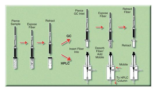
**FIGURE 1.10** Schematic of the SPME process. (Used with permission from Sigma-Aldrich, a part of MilliporeSigma. www.sigmaaldritch.com. Copyright 2020 Sigma-Aldrich Co. LLC. All rights reserved.)
