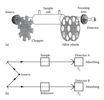
**FIGURE 4.30** (a) Schematic of a two-filter wheel, multiwavelength filter photometer. (From Coates, used with permission.) (b) Schematic of a positive-filter nondispersive IR system.
