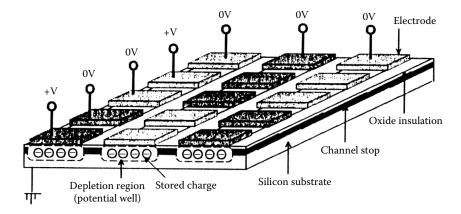
**FIGURE 7.18** Schematic of a CCD. In this CCD, three electrodes define a pixel. (Courtesy of Horiba, Inc. © 2020 HORIBA Scientific [www.horiba.com/scientific]. All rights reserved.)
