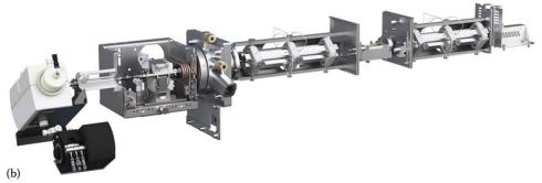
**FIGURE 9.57 (a)** The Agilent technologies 8800 ICP-QQQ. **(b)** The interior of the 8800 ICP-QQQ. From the left, sample introduction, the ICP torch box (note the cooling coils for the torch), Q1, the ORS<sup>3</sup> octopole collision/reaction cell, Q2 and finally the electron multiplier detector. (© 2020 Agilent Technologies [www.agilent.com/chem]. All rights reserved. Used with permission.)
