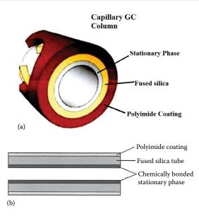
**FIGURE 10.7** (a) Schematic cross section of a capillary column. (b) Schematic of a fused silica open tubular column for chromatography.
