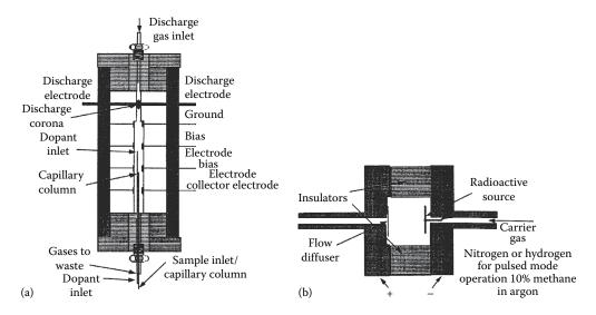
**FIGURE 11.21** Diagrams of two types of electron capture detectors (ECD). **(a)** ECD for use with pulsed electrode potential and **(b)** ECD for use with constant electrode potential. (Cazes, used with permission.)
