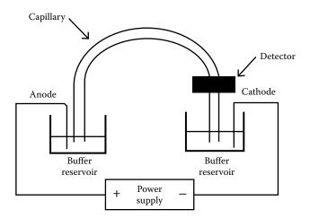
**FIGURE 12.38** Schematic of capillary zone electrophoresis apparatus. (Cazes, used with permission.)
