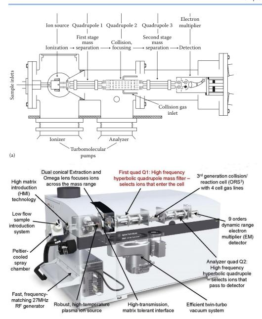
**FIGURE 9.33 (a)** A commercial quadrupole tandem MS/MS instrument for organic MS. (© Thermo Fisher Scientific [www.thermofisher.com]. Used with permission.) **(b)** The 8800 ICP-QQQ with two hyperbolic quadrupoles separated by an octopole cell for ICP-MS/MS. (© 2020 Agilent technologies [www.agilent.com/chem]. All rights reserved. Used with permission.)
