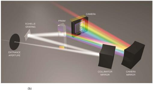
**FIGURE 7.14** A schematic diagram of an Echelle spectrometer. Two dispersive devices are used. **(a)** The prism disperses light in the vertical plane; The grating disperses the vertically dispersed light in the horizontal plane. The physical arrangement of the grating and prism can be reversed as in **(b)** or two gratings may be used. (Courtesy of SPECTRO, a unit of the materials analysis division of AMETEK, Inc., www.spectro.com, used with permission.)
