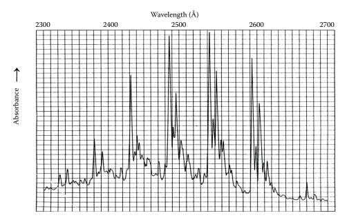
**FIGURE 3.11** Gas phase absorption spectrum of benzene. (From Jaffé and Orchin. Reprinted with the permission of the late professor M. Orchin.)
