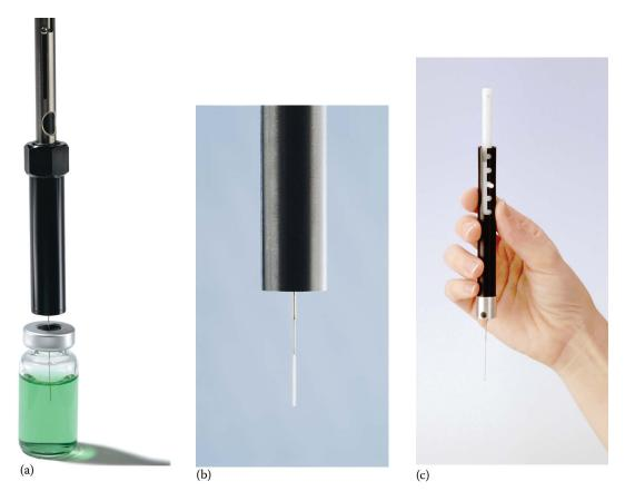
**FIGURE 1.9** (a) Commercial SPME unit with the coated fiber (b) Inserted into a sample vial. (c) An SPME probe the size of a ballpoint pen. (Used with permission from Sigma-Aldrich, a part of MilliporeSigma. www.sigmaaldritch.Com. Copyright 2020 Sigma-Aldrich Co. LLC. All rights reserved.)
