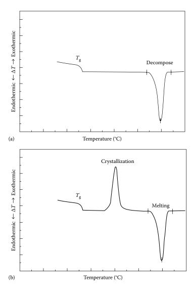
**FIGURE 14.18** Schematic DTA thermal curves for the totally amorphous polymer structure and the semicrystalline polymer structure shown in figure 14.17. Both show  $T_g$ ; only the semicrystalline polymer has a crystallization exotherm.
