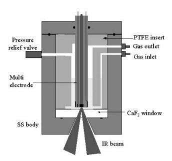
**FIGURE 13.42** A schematic cell for IR-SEC studies. Note the IR-transparent CaF<sub>2</sub> window. (Courtesy of Professor Stephen P. Best, University of Melbourne, Australia.)
