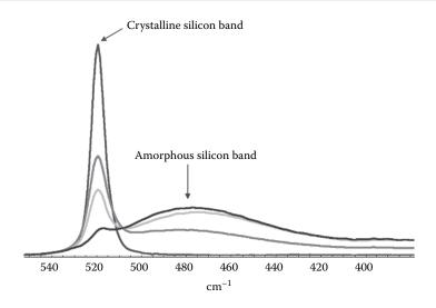
FIGURE 4.57 Raman spectra of silicon samples ranging from pure crystalline to primarily amorphous silicon. The spectra show a sharp band at 521 cm<sup>-1</sup> from crystalline silicon and a much broader band centered at approximately 480 cm<sup>-1</sup> from amorphous silicon. (From Deschaines et al., © Thermo Fisher Scientific [www.thermofisher.com]. Used with permission.)
