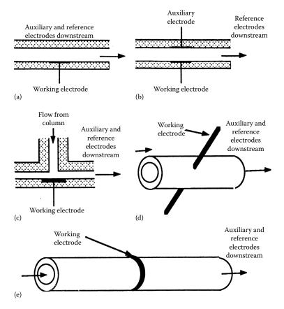
**FIGURE 12.17** Five HPLC electrochemical detector three-electrode arrangements. (Scott, used with permission.)
