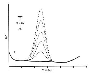
FIGURE 13.34 Effect of standard additions on a differential pulse polarogram.
