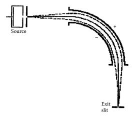
**FIGURE 9.19** A cylindrical electrostatic-sector energy filter. (From Ewing, used with permission.)
