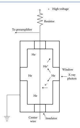
**FIGURE 8.36** Schematic diagram of a gas-filled X-ray detector tube. He filler gas is ionized by X-ray photons to produce He<sup>+</sup> ions and electrons, e<sup>-</sup>. the electrons move to the positively charged center wire and are detected. (Modified from Parsons, used with permission.)
