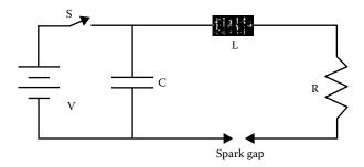
**FIGURE 7.8** Schematic spark excitation source. S is a switch, C is a capacitor, L is an inductor, R is a resistor, and V is a voltage source. (From Thomsen, used with permission from ASM International\*.)
