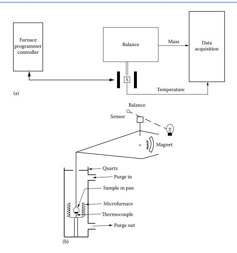
**FIGURE 14.3** (a) Block diagram of a TGA system. S represents the sample pan hanging from the balance arm in position in the furnace (represented by the solid bars on each side). (b) Schematic of a commercial TGA, showing the purge gas inlet and outlet and the thermocouple position beneath the sample pan. (b: © 2020 PerkinElmer, inc. All rights reserved. Printed with permission. [www.perkinelmer.com].)
