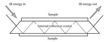
**FIGURE 4.21** Schematic ATR sampling accessory. The internal reflection crystal permits multiple reflections. At each reflection, a small amount of IR energy penetrates the sample and absorption occurs at the vibrational frequencies for the sample. (Courtesy of Pattacini Associates, LLC, Danbury, CT.)
