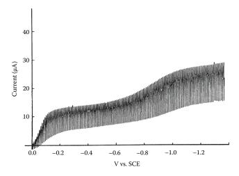
**FIGURE 13.29** Polarogram of dissolved oxygen in an electrolyte, 1 M KNO<sub>3</sub> (scan rate 5 mV/s, 2 s drop time).
