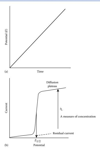
FIGURE 13.26 (a) Linear potential excitation and (b) the resulting polarographic wave.
