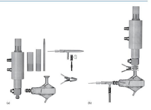
**FIGURE 7.33 (a)** The components of a liquid sample introduction system for ICP: glass concentric nebulizer, demountable three-piece quartz torch, torch body, and glass cyclonic spray chamber. **(b)** The components assembled for use. This torch design is typical of that used in Horiba Scientific ICP instruments. (Courtesy of Glass Expansion Pty, Ltd., Australia [www.geicp.com].)
