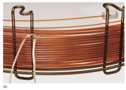
**FIGURE 10.8** (a) A commercial glass capillary column for gas chromatography. (b) Close-up of a fused silica capillary column. (Both courtesy of Restek corporation, Bellefonte, PA., www.restek. com. Used with permission.)
