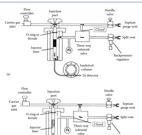
**FIGURE 11.7** Diagram of GC flows for split and splitless injections: **(a)** split mode; **(b)** splitless mode. (Adapted with permission of Restek Corporation, Bellefonte, PA, www.restek.com.)
