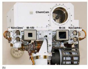
**FIGURE 7.53 (a)** Artist's conception of the mars rover curiosity, showing the raised mast head. **(b)** Close-up of the actual mast head with the ChemCam. (Image credits: Courtesy of NASA/JPL-Caltech/LANL.)
