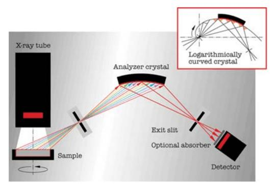
**FIGURE 8.42** Monochromator schematic with a logarithmic spiral curved crystal. (© 2020 Bruker, Inc. [www.bruker.com]. Used with permission.)
