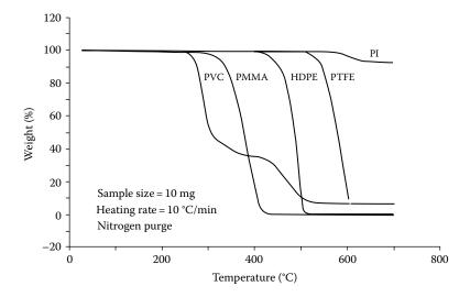
**FIGURE 14.10** TGA thermal curves showing the decomposition temperatures of some common polymers: PVC, polyvinylchloride; PMMA, polymethylmethacrylate; HDPE, high-density polyethylene; PTFE, polytetrafluoroethylene; PI, polyimide. (Courtesy of TA instruments, New Castle, www.tainstruments.com.)
