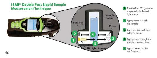
**FIGURE 3.35** (a) The i-LAB® visible hand held analyzing spectrometer measuring a solid sample. (b) Schematic of the i-LAB® liquid sample measurement technique. (Courtesy of Microspectral Analysis, LLC, Wilton, ME [www.microspectralanalysis.com]. All rights reserved.)
