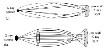
**FIGURE 8.45** (a) Schematic of a mono-capillary X-ray optic for producing micro-beams of X-rays. (b) Schematic of poly-capillary X-ray optics for producing micro-beams of X-rays. (©2020 HORIBA Scientific, Itd. [www.horiba.com]. All rights reserved.)
