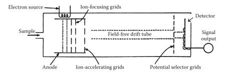
**FIGURE 9.26** Schematic TOF mass spectrometer.
