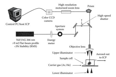
**FIGURE 7.34** A commercial laser ablation system for solid samples, the CETAC technologies LSX-500. (Courtesy of Teledyne CETAC Technologies, Omaha, NE [www.cetac.com].)
