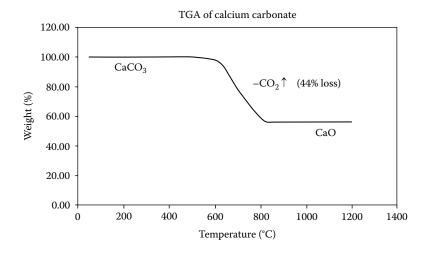
**FIGURE 14.1** TGA thermal curve for pure anhydrous calcium carbonate,  $CaCO_3$ . The loss in mass is due to the loss of  $CO_2(g)$  and the compound remaining is  $CaO_3$ .
