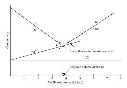
**FIGURE 13.23** Solution conductivity during an HCl-NaOH titration. Point C is the neutralization point.
