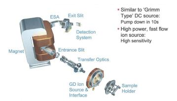
**FIGURE 9.21** Reverse Nier-Johnson geometry of the Thermo Scientific element MS with a GD source. (© Thermo Fisher Scientific [www.thermofisher.com]. Used with permission.)
