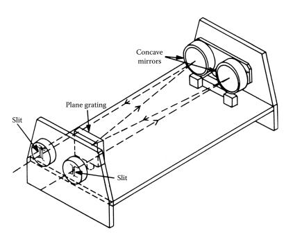
**FIGURE 2.25** A grating monochromator showing the optical slits. The entrance slit is on the right and the exit slit on the left. (Dean, J.A. and Rains, T.C., Eds., *Flame Emission and Absorption Spectrometry*, Vol. 2, Marcel Dekker, Inc., New York, 1971. Used with permission.)
