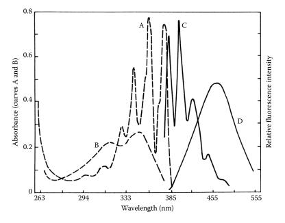
**FIGURE 3.52** Excitation and fluorescence spectra of anthracene and quinine: curve a, anthracene excitation; curve b, quinine excitation; curve c, anthracene fluorescence; curve d, quinine fluorescence. (From Guilbault, used with permission.)
