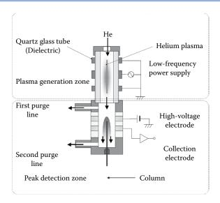
**FIGURE 11.24** Design of the dielectric barrier discharge ionization detector (BID). (Used with permission from Shimadzu corporation, Kyoto, Japan; www.shimadzu.com.)
