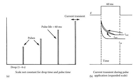
**FIGURE 13.31** (a) Waveform for normal pulse polarography and (b) current transient response (not to scale).
