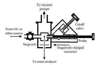
The sample is placed into the cavity or quartz insert (called a crucible) in the tip of the probe. When not in use, the cutoff valve is closed and gas samples can be introduced by opening the stopcock shown. The black dot at the center of the square shows the point at which the electron beam impacts the sample. (From Ewing, used with permission.)
