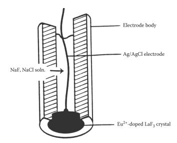
**FIGURE 13.9** A commercial solid-state fluoride ISE. The ion-sensitive area is a solid crystal of LaF<sub>3</sub> doped with EuF<sub>2</sub>. The filling solution contains NaF and NaCl. The electrical connection is made by an Ag/AgCl electrode. (© Thermo Fisher Scientific [www.thermofisher.com]. Used with permission.)
