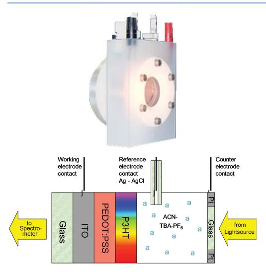
**FIGURE 13.39** A photo of the ZAHNER PECC-2 cell (left side) and a schematic diagram of a model system for an organic solar cell film sample with electrode positions shown on the right side. The schematic is not to scale. (Courtesy of C.-A. Schiller, ZAHNER-Elektrik GmbH & Co. KG. \*ZAHNER-Elektrik GmbH & Co. KG, Kronach, Germany [www.zahner.de].)
