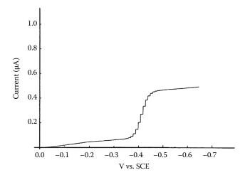
**FIGURE 13.30** Normal pulse polarogram of Pb<sup>2+</sup> ions (5 ppm) in 1 M KNO<sub>3</sub> (scan rate 5 mV/s, 2 s drop time).
