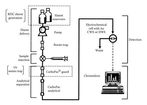
**FIGURE 12.18** Schematic diagram of HPAE-PAD system. (© Thermo Fisher Scientific (www. thermofisher.com). Used with permission.)
