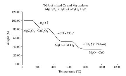
**FIGURE 14.8** TGA thermal curve of a mixture of calcium oxalate monohydrate and magnesium oxalate dihydrate. The last weight loss is due to the loss of CO<sub>2</sub> only from calcium oxalate monohydrate. Therefore, the composition of the mixture can be determined, even though the other steps have combined mass losses from both compounds.
