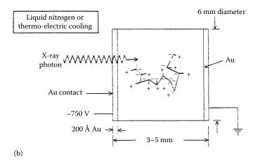
**FIGURE 8.23** The Si(Li) semiconductor detector. **(a)** Schematic shows the n-type Si region on one end of the Si crystal, a central charge depleted intrinsic region and p-type Si on the other end. **(b)** The actual detector has 200 Å layers of gold as electric contacts on each end of the crystal. An X-ray photon striking the intrinsic region generates electron-hole pairs within the diode. (b: © Thermo Fisher Scientific [www.thermofisher.com]. Used with permission.)
