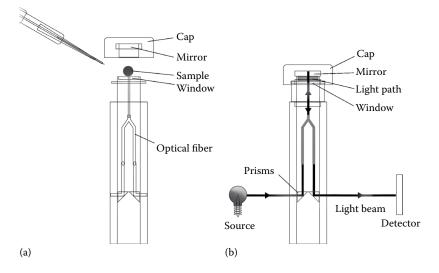
**FIGURE 3.31** Left: sample is pipetted onto the cell window. Right: the cap compresses the sample into a fixed pathlength. (Graphic courtesy of Hellma Analytics [www.hellmausa.com].)
