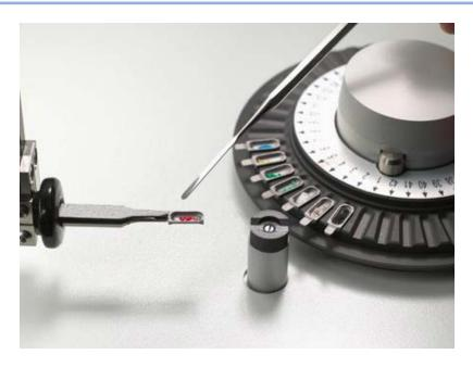
**FIGURE 6.30** The SS600° solids autosampler for direct solids analysis by graphite furnace AAS. (©2020 Analytik Jena, [www.analytik-jena.de]. Used with permission.)
