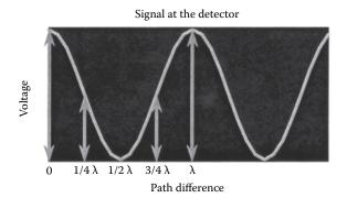
**FIGURE 4.11** (Top) A simplified schematic showing the generation of an interferogram from monochromatic light by displacement of the moving mirror. (Modified from Coates, used with permission). (Bottom) An enlarged view of the signal at the detector as a function of path difference between the moving and fixed mirrors for monochromatic light of wavelength  $\lambda$ . (© Thermo Fisher Scientific [www.thermofisher.com]. Used with permission.)
