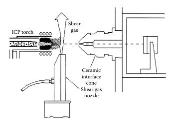
**FIGURE 7.29** Axial (end-on) ICP torch position showing how the shear gas cuts off the cool plasma tail plume. Light emitted from the plasma passes through the ceramic interface into the spectrometer on the right side of the diagram (not shown). (© 1999-2020 PerkinElmer, Inc. All rights reserved. Printed with permission. [www.perkinelmer.com].)
