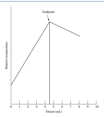
**FIGURE 14.33** Representative thermometric titration plot. The endpoint is denoted by an abrupt change in the slope of the curve. The thermometric titration plot for HCl (a strong acid) with NaOH would look virtually identical to the thermometric titration plot for boric acid (a very weak acid) with NaOH because the  $\Delta H$  of reaction is almost the same for both acids.
