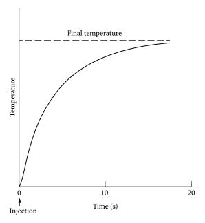
**FIGURE 14.34** DIE titration plot. An excess of reactant B is added rapidly. The amount of analyte a is calculated from the final temperature.
