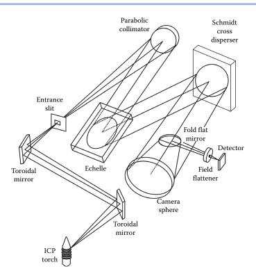
**FIGURE 2.23** An echelle spectrometer optical layout. The echelle grating disperses the light to a second wavelength selector, called a cross-disperser. (©1997-2020 PerkinElmer, Inc. All rights reserved. Printed with permission. www.perkinelmer.com.)
