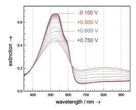
**FIGURE 13.40** Spectra series for the model solar cell layer system from the previous figure. The plots are of extinction versus wavelength at a series of cell voltages. (Courtesy of C.-A. Schiller, ZAHNER-Elektrik GmbH & Co. KG. \*ZAHNER-Elektrik GmbH & Co. KG, Kronach, Germany [www.zahner.de].)
