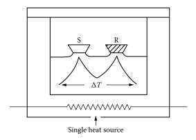
**FIGURE 14.16** Schematic DTA instrument. (© 2020 PerkinElmer, inc. All rights reserved. Printed with permission. [www.perkinelmer.com].)
