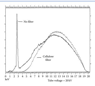
**FIGURE 8.18** The use of a filter to remove unwanted radiation from entering the spectrometer is demonstrated. A cellulose filter placed between a Rh X-ray tube and the sample removes the Rh  $L_{\alpha}$  line at 2.69 keV and allows only the continuum radiation to excite the sample. (© Thermo Fisher Scientific [www.thermofisher.com]. Used with permission.)
