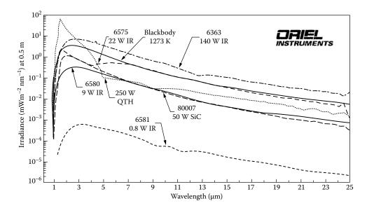
**FIGURE 4.7** Spectral output of a variety of commercial IR radiation sources, including a silicon carbide source (dashed line marked SiC) and an NIR quartz tungsten-halogen lamp (the dotted line marked QTH). A blackbody curve at 1273 K is included for comparison. (Courtesy of Newport corporation, Irvine, CA [www.newport.com].)
