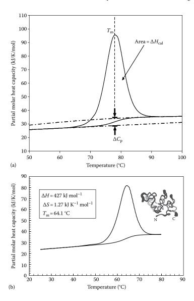
**FIGURE 14.35** (a) A schematic DSC scan, showing how  $T_m$ ,  $\Delta H$  and  $\Delta C_p$  are obtained. (b) A temperature scan, converted to partial molar heat capacity for 1 mg/mL<sup>-1</sup> hen egg white lysozyme (shown in the upper right corner) in 0.2 M glycine buffer, pH 2.7. Data obtained at a scan rate of 1 °C/min in a nano DSC. (Courtesy of TA instruments, New Castle, DE. www.tainstruments. com.)
