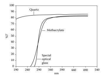
**FIGURE 3.27** Transparencies of materials used to make sample cells for UV/VIS spectroscopy.
