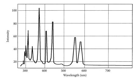
**FIGURE 3.50** Spectral output of a mercury arc lamp, used as a source in fluorometers. (From Froelich and Guilbault, used with permission.)
