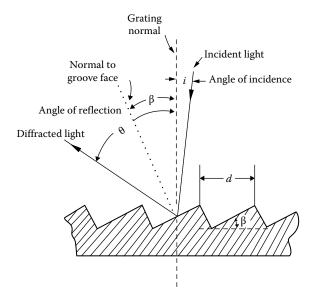
**FIGURE 2.16** Cross-section diagram of a diffraction grating showing diffraction of a single beam of light. Symbols: i = angle of incidence,  $\theta =$  angle of diffraction (or reflectance),  $\beta =$  blaze angle of the grating, d = grating spacing. (Modified from Dean and Rains, used with permission.)
