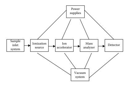
**FIGURE 9.4** Block diagram of a mass spectrometer.
