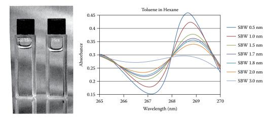
**FIGURE 2.22** Spectral bandwidth measurements using a sealed cell containing 0.02 % toluene in hexane and a hexane blank cell. (Courtesy of Starna Cells, Inc. Atascadero, CA [www.starnacells.com].)
