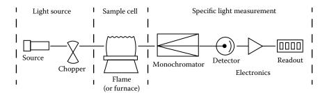
**FIGURE 6.9** Basic AAS system. (© 1993-2020 PerkinElmer, inc. All rights reserved. Printed with permission. [www.perkinelmer.com].)
