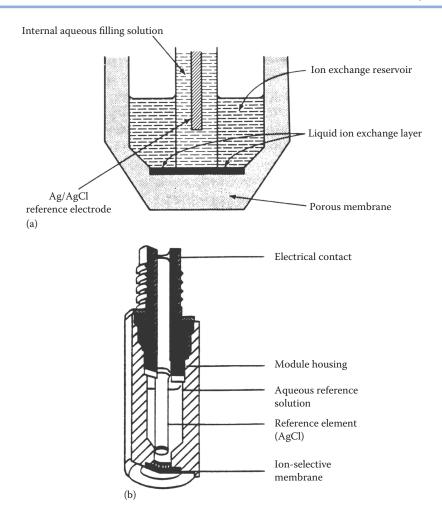
**FIGURE 13.10** (a) A liquid membrane ISE. (b) An ISE with ion exchange material in a solid polymer membrane. The sensed ion is exchanged across the membrane, creating the potential. This type of ISE is available for Ca<sup>2+</sup>, K<sup>+</sup>, nitrate ion, and nitrite ion determinations. (b: © Thermo Fisher Scientific [www.thermofisher.com]. Used with permission.)
