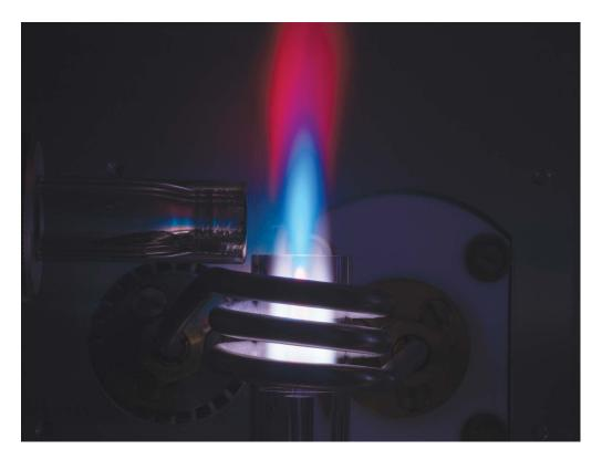
**FIGURE 7.25** Argon ICP torch in operation. The analytical zone is the blue region above the coils. Compare with Figure 7.24. (Courtesy of SPECTRO, a unit of the materials analysis division of AMETEK, Inc., www.spectro.com. Used with permission.)
