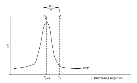
FIGURE 13.33 Waveform obtained in differential pulse polarography.
