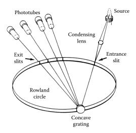
**FIGURE 7.12** A Rowland circle polychromator. This configuration is called a Paschen-Runge mount. The source shown is an inductively coupled plasma, but any of the electrical excitation sources can be substituted. Multiple photomultiplier detectors are placed at the appropriate positions on the circumference of the circle to measure dispersed wavelengths or a CCD detector can be used. (© 1999-2020 PerkinElmer, inc. All rights reserved. Printed with permission. [www.perkinelmer.com].)
