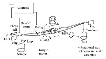
**FIGURE 14.4** (a) Electrobalance for a TGA. As the sample weight changes, the balance arm tips, resulting in a change in the amount of light reaching the photocell. This generates a current to restore the arm position; the current is proportional to the change in weight of the sample. (© Thermo Fisher Scientific [www.thermofisher.com]. Used with permission.)
