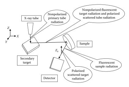
**FIGURE 8.16** Schematic drawing of a 3D beam of a secondary target EDXRF system. (Modified from a diagram provided by Bruno Vrebos, courtesy of Malvern Panalytical Inc., Almelo, the Netherlands [www.malvernpanalytical.com]. Used with permission.)
