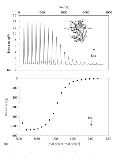
**FIGURE 14.39** (a) Simulated raw incremental titration data for an ITC experiment. Each peak corresponds to the heat produced upon injection of a fixed amount of titrant at specific time intervals. (b) Simulated binding analysis. Area under each peak in (a) is integrated and fit to a binding model to permit calculation of affinity, enthalpy and stoichiometry for the interaction. (Courtesy of TA instruments, New Castle, DE. www.tainstruments.com.)
