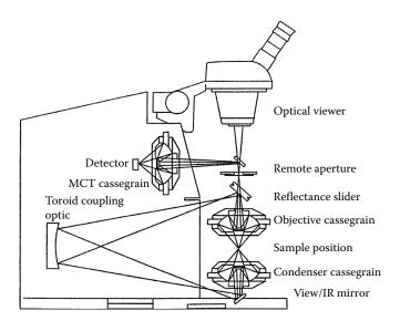
**FIGURE 4.24** IR microscope schematic with the detector integrated into the microscope. The microscope is usually coupled to a light port on the side of the FTIR spectrometer. The FTIR spectrometer supplies a modulated, collimated beam of light to the microscope. (© 2020 PerkinElmer, inc. All rights reserved. Printed with permission. www.perkinelmer.com.)
