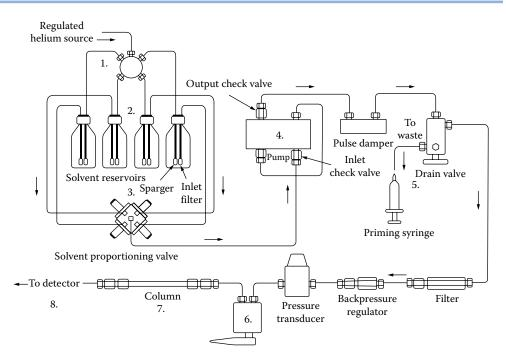
**FIGURE 12.8** Diagram of conventional HPLC instrument. (© 2020 Perkin Elmer, Inc. All rights reserved. Printed with permission. [www.perkinelmer.com].)
