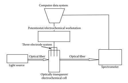
**FIGURE 13.37** Schematic basic spectroelectrochemistry instrument.
