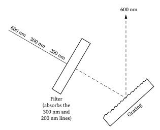
**FIGURE 2.19** A filter is used as an order sorter to prevent higher-order wavelengths from reaching the grating.
