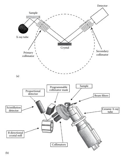
**FIGURE 8.30 (a)** Schematic of the optical path in a wavelength-dispersive sequential spectrometer, showing the positions of the collimators. **(b)** Schematic layout of a commercial sequential WDXRF system. (Courtesy of Malvern Panalytical Inc., Almelo, the Netherlands [www.malvernpanalytical.com]. Used with permission.)
