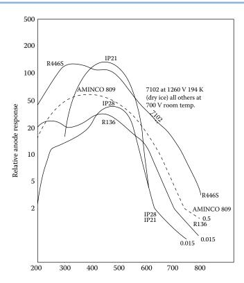
**FIGURE 3.19** Response curves for various commercial PMTs. Note the variable response among different models and the sharp drop-off in response outside the useable range.
