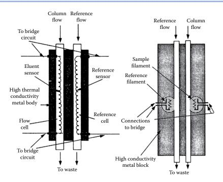
**FIGURE 11.19** Diagrams of two types of thermal conductivity detectors (TCD). (Cazes, used with permission.)
