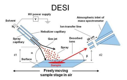
**FIGURE 9.15** Prosolia DESI omni spray ion source geometry and operation diagram. The family of different (manual, 1D and 2D) ion sources can be used on MS equipment from Agilent, Thermo, Waters, ABSciex, Bruker, and LECO. (Used with permission from Prosolia, inc., www.prosolia.com.)
