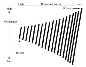
**FIGURE 2.24** Illustration of the two-dimensional (2D) array of dispersed light produced by an echelle spectrometer. (©1997-2020 PerkinElmer, Inc. All rights reserved. Printed with permission. www.perkinelmer.com.)
