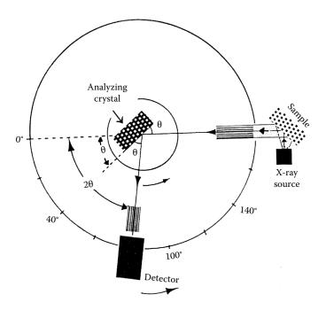
**FIGURE 8.34** Goniometer layout for a sequential XRF spectrometer.
