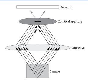
**FIGURE 4.51** A simplified illustration of confocal microscopy. A spectrum is collected only from the area of the sample denoted by the middle arrow; only that light exits the confocal aperture. Information from all other sample areas is blocked. Raising or lowering the sample will allow the detector to collect Raman scatter from levels in the sample lower or higher than the area in the middle. (Reprinted from Weesner and Longmire, with permission from Advanstar Communications, Inc.)
