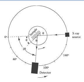
**FIGURE 8.66** Schematic layout of a single-crystal XRD.
