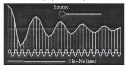
**FIGURE 4.13** Schematic diagram showing how the interferogram is digitized by sampling it at discrete points based on the He-Ne laser signal, shown at the bottom. Each vertical line represents a sampling point. (© Thermo Fisher Scientific [www.thermofisher.com]. Used with permission.)
