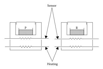
**FIGURE 14.20** Schematic of a power-compensated DSC. (© 2020 PerkinElmer, inc. All rights reserved. Printed with permission. [www.perkinelmer.com].)
