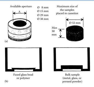
**FIGURE 8.20** (a) Sample cassette for bulk solid samples. (b) Position of a bulk solid in the face-down configuration used in many spectrometers. (© Thermo Fisher Scientific [www.thermofisher.com]. Used with permission.)
