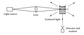
**FIGURE 3.40** Schematic optical system for nephelometry.
