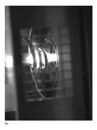
**FIGURE 9.16** (a) Argon ICP torch used as an ionization source for ICPMS. (From Ewing, used with permission.) (b) Photo of the plasma in a SPECTRO MS system (described in section 9.2.3). (Courtesy of SPECTRO analytical instruments, inc., AMETEK\* materials analysis division [www.spectro.com, www.ametek.com]. Used with permission.)
