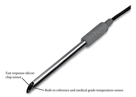
**FIGURE 13.12** A commercial ISFET pH probe, with a silicon chip pH sensor, a built-in reference electrode, and a built-in temperature sensor. This pH probe is housed in a stainless steel body with a slanted tip for easy insertion into meat or other soft solid samples. (Courtesy of IQ Scientific Instruments, Inc., Carlsbad, CA., www.phmeters.com.)
