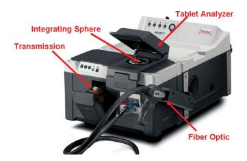
**FIGURE 4.34** Antaris II <sup>™</sup> FT-NIR analyzer, Thermo Scientific, equipped with a fiber optic probe for remote measurement, transmission, and integrating sphere and a tablet analyzer for direct analysis of pharmaceuticals. (© Thermo Fisher Scientific [www.thermofisher.com]. Used with permission.)
