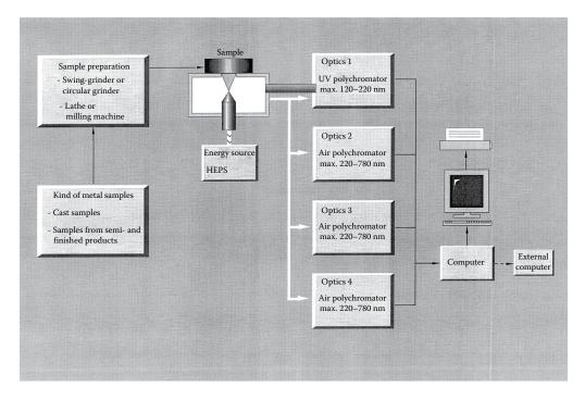
**FIGURE 7.13** Schematic diagram of the SPECTROLAB spark emission spectrometer system. (Courtesy of SPECTRO Analytical Instruments GmbH, a division of AMETEK, Inc. www.spectro.com, www.ametek.com.)
