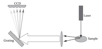
**FIGURE 4.41** Schematic of a dispersive Raman spectrometer. (Reprinted from Weesner and Longmire, with permission from Advanstar Communications, Inc.)
