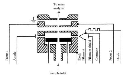
**FIGURE 9.6** Cross-section of an El source. The filament and anode define the electron beam. The ions are formed in the space above the two repellers (the solid color blocks). A positive charge on the repellers together with a negative potential on the focus electrodes cause positive ions to be accelerated upward in the diagram, into the mass analyzer. (Modified from Ewing, used with permission.)
