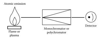
**FIGURE 7.2** Schematic atomic emission spectrometer. (© 1999-2020 PerkinElmer, inc. All rights reserved. Printed with permission. [www.perkinelmer.com].)
