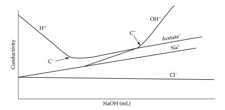
**FIGURE 13.25** Solution conductivity during titration of a mixture of HCl and CH<sub>3</sub>COOH with NaOH. Here C' and C" designate the respective endpoints. HCl is titrated first and then the weaker acetic acid is neutralized.
