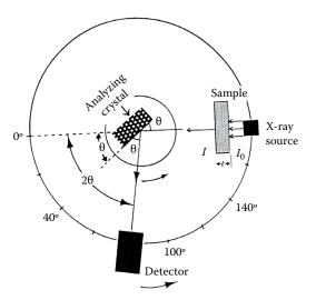
**FIGURE 8.57** X-ray absorption. The sample is placed between the X-ray tube and the detector. The intensity of the source is  $I_0$ . the intensity of light reaching the detector after passing through a sample of thickness t is l. l will be less than  $l_0$  if absorption occurs.
