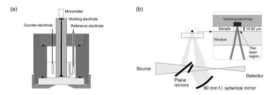
**FIGURE 13.43** Schematic diagrams of an IR-SEC cell (left) and how the cell fits into a commercial FTIR spectrometer (right). (From Best, S.P.; Borg, S.J.; Vincent, K. A. Infrared spectroelectrochemistry in *spectroelectrochemistry*, Kaim, W.; Klein, A., Eds., RSC Publishing: Cambridge, UK, 2008. Reproduced by permission of the Royal society of chemistry.)
