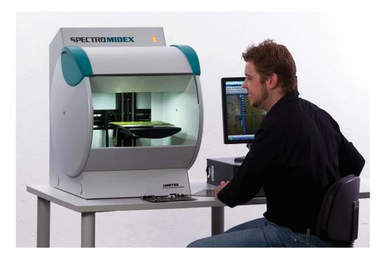
**FIGURE 8.46** A micro-XRF system with a large sample chamber, the SPECTRO MIDEX. This is used for analysis of large objects, such as the complete circuit board shown to the left of the analyst. (© SPECTRO analytical instruments, a unit of the materials analysis division, AMETEK, Inc. [www.ametek.com]. Used with permission.)
