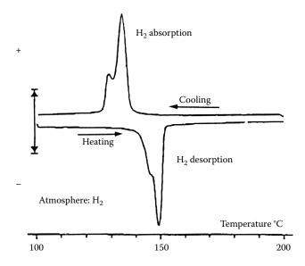
**FIGURE 14.26** DSC thermal curve of adsorption and desorption of hydrogen from a precious metal catalyst under constant pressure.
