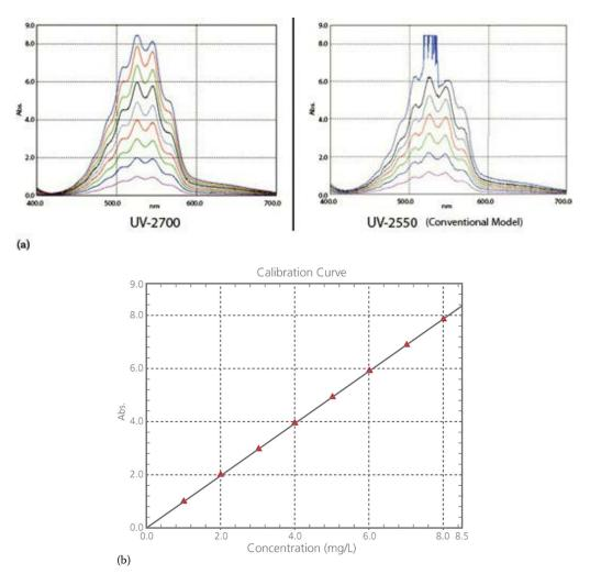
**FIGURE 3.16** (a) Left: Spectra obtained on a UV-2700 spectrometer equipped with a Lo-Ray-Ligh grating; right: the same spectra collected on a conventional spectrometer. Note that the signals on the conventional system go over the operating range. (b) Calibration curve from the UV-2700 showing linearity up to absorbance = 8.5. (© 2020 Shimadzu Scientific Instruments, [www.ssi.shimadzu.com]. Used with permission.)
