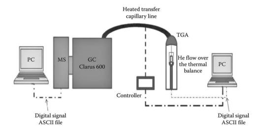
**FIGURE 14.29** Schematic of a TGA coupled to a GC-MS through a heated transfer capillary line. (© 2020 PerkinElmer, inc. All rights reserved. Printed with permission. www.perkinelmer.com.)
