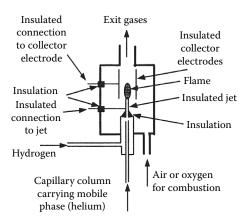
**FIGURE 11.20** Diagram of the flame ionization detector (FID). (Cazes, used with permission.)
