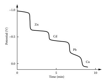
**FIGURE 13.36** Stripping voltammogram of metal-ion species at a TFME.
