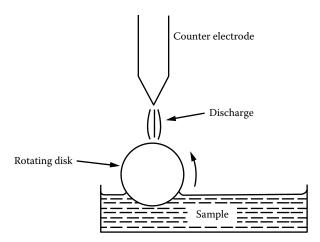
**FIGURE 7.11** A schematic rotating disk electrode (or rotrode) used for the introduction of liquid samples into an electrical discharge. The system is used primarily for the determination of metals in oils. The RDE is shown with an arc source and fiber optic lead to a Rowland circle polychromator with CCD detector. (Courtesy of Spectro Scientific, Chelmsford, MA. www.spectrosci. com. Used with permission.)
