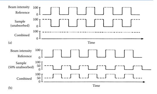
**FIGURE 2.29** Radiation intensity reaching the detector using double-beam optics and a rotating disk beam splitter. (a) No absorption by the sample; (b) 50 % absorption by the sample.
