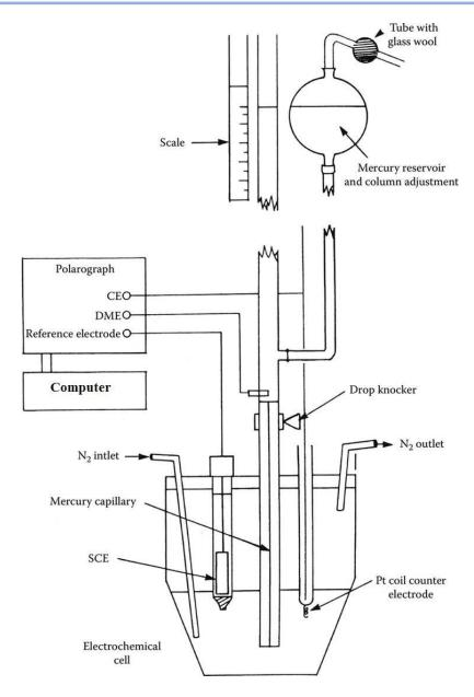
FIGURE 13.27 Modern polarographic cell and three-electrode circuit.
