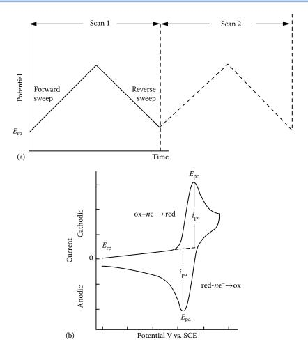
**FIGURE 13.35 (a)** Excitation waveform and **(b)** current response for a reversible couple obtained in cyclic voltammetry.
