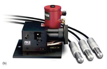
**FIGURE 4.22 (a)** Hollow wave guide schematic **(b)** Mid-IR FlexIR™ with remote probes **(c)** ATR spectra of human skin, skin treated with sunscreen and the result of spectral subtraction. (Courtesy of PIKE technologies, www.piketech.com. Used with permission.)
