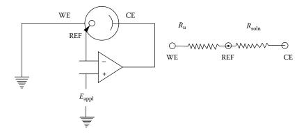
**FIGURE 13.14** Schematic of a simple potentiostat and representation of the cell as an electrical (equivalent) circuit.
