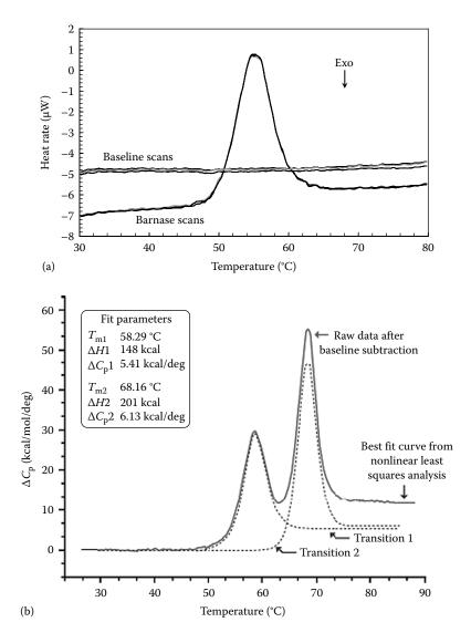
**FIGURE 14.36** (a) Three overlaid baseline temperature scans and three overlaid scans of 60 mg barnase in 0.3 mL 20 mM phosphate buffer, pH 5.5. (Courtesy of TA instruments, New Castle, DE. www.tainstruments.com.) (b) Stability assessment of two biomolecules using the MicroCal VP-DSC. (©2020 General electric company doing business as GE Healthcare [www.gelifesciences.com/microcal].)
