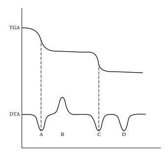
**FIGURE 14.28** The TGA and DTA curves of a hypothetical sample. The two steps in the TGA curve result from weight losses. They correspond to the endothermic peaks A and C in the DTA plot. The DTA thermal curve also shows an exothermic event, B, and an endothermic event, D, that do not involve a change in mass.
