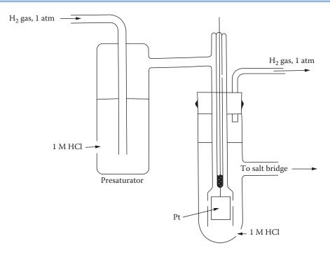
**FIGURE 13.4** The standard hydrogen electrode (SHE). This design is shown with a pre-saturator containing the same 1 M HCl solution as in the electrode to prevent concentration changes by evaporation. (Aikens et al., Waveland press inc., Long Grove, IL, 1984. All rights reserved.)
