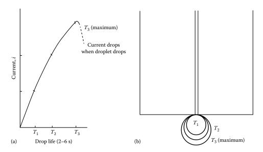
**FIGURE 13.28** (a) Current waveform and (b) time frame of an expanding drop.
