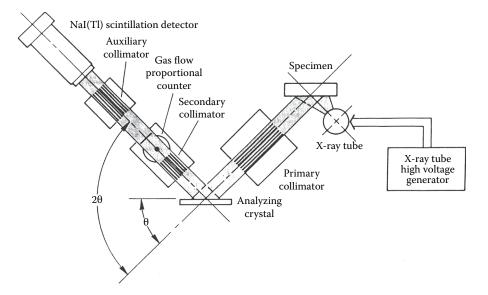
**FIGURE 8.31** A sequential spectrometer with two tandem detectors, showing the placement of the collimators in the optical path. (From Jenkins et al., 1981, Used with permission.)
