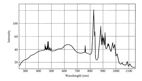
**FIGURE 3.49** Spectral output of a compact xenon arc lamp. (From Froelich and Guilbault, used with permission.)
