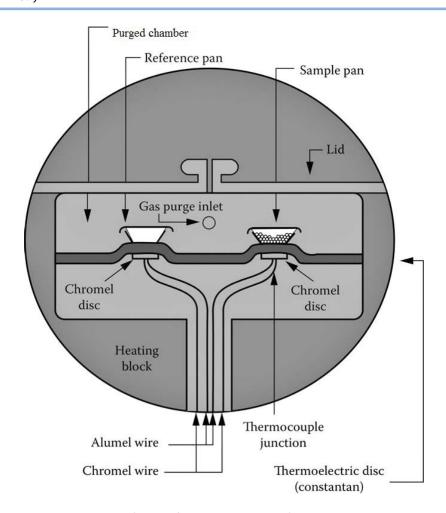
**FIGURE 14.19** Schematic of a heat-flux DSC. (Courtesy of TA instruments, New Castle, www. tainstruments.com.)
