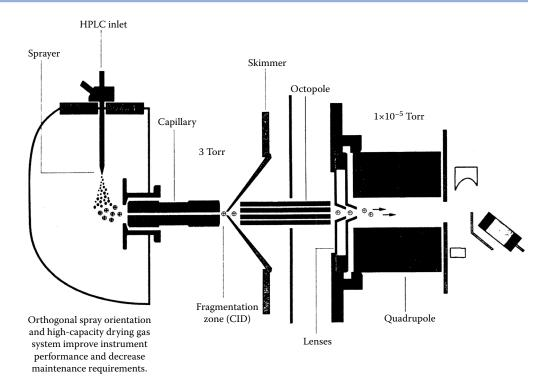
**FIGURE 12.23** Diagram of orthogonal electrospray LC-MS interface. (© 2020 Agilent Technologies [www.agilent.com/chem] All rights reserved. Used with permission.)
