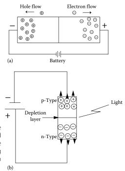
**FIGURE 3.23** (a) A p-n junction under reverse bias. The positive battery terminal is connected to the n side. A depletion layer forms along the junction. (b) Diagram of a photodiode showing light incident upon the depletion layer. (From Brown, used with permission.)
