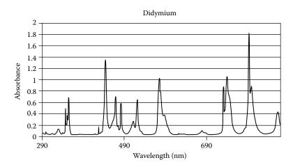
**FIGURE 2.20** Didymium oxide UV/VIS wavelength reference spectra, from a sealed quartz cell containing didymium oxide in perchloric acid solution. (Courtesy of Starna Cells, Inc., Atascadero, CA [www.starnacells.com].)
