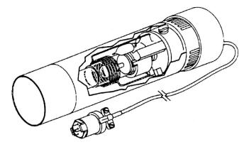
**FIGURE 6.7** Electrodeless discharge lamp. (© 1993-2020 PerkinElmer, inc. All rights reserved. Printed with permission. [www.perkinelmer.com].)
