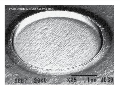
**FIGURE 7.44** A GD "sputter spot" in a steel sample showing the uniform removal of the surface. It is this uniform sputtering process that permits accurate depth profiling of layered materials by glow discharge OES. (Courtesy of Sandvik Materials Technology, Sandvikem, Sweden, [www.smt.sandvik.com].)
