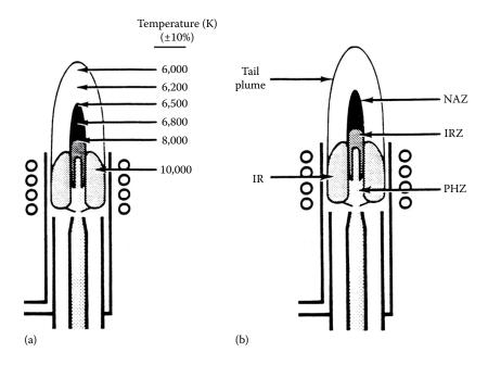
**FIGURE 7.24 (a)** Temperature regions in a typical argon ICP discharge. **(b)** Zones of the ICP discharge. IR, induction region; PHZ, preheating zone; IRZ, initial radiation zone; NAZ, normal analytical zone. (© 1999-2020 PerkinElmer, inc. All rights reserved. Printed with permission. [www.perkinelmer.com].)
