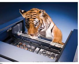
**FIGURE 8.44** (a) The S8 TIGER, a floor-mounted commercial WDXRF system. (b) The sample compartment of the S8 TIGER, showing the multi-position autosampler with typical samples such as polished metal flats on the left and pressed pellets on the right. (The namesake operator is not standard but is useful in providing scale!) (© 2020 Bruker, Inc. [www.bruker.com]. Used with permission.)
