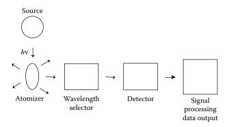
**FIGURE 7.50** Schematic AFS spectrometer system showing the typical 90° orientation between the source and the wavelength selector and detector to minimize scattered radiation.
