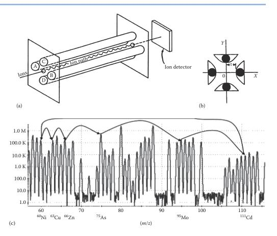
**FIGURE 9.31** (a) Transmission quadrupole mass spectrometer. Rods A and B are tied together electrically, as are rods C and D. The two pairs of rods, AB and CD, are connected both to a source of direct potential and a variable RF excitation such that the RF voltages are 180° out of phase. (b) The geometry of the rods. (c) Sequential detection of elements by peak hopping (ICP-MS).
