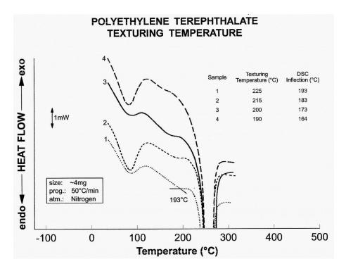
**FIGURE 14.24** PET heat-treatment and the resulting changes in the DSC thermogram. (Courtesy of TA instruments, New Castle. from thermal analysis applications brief TA-128. www.tainstruments.com.)
