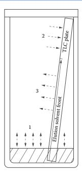
FIGURE 12.43 TLC plate in enclosed developing tank.
