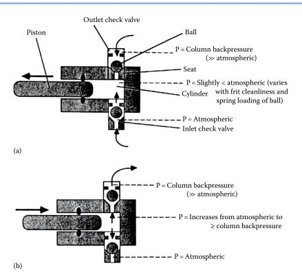
**FIGURE 12.9** Operation of piston and check valve reciprocating pump: **(a)** fill stroke and **(b)** exhaust stroke. (Katz et al., Used with permission.)
