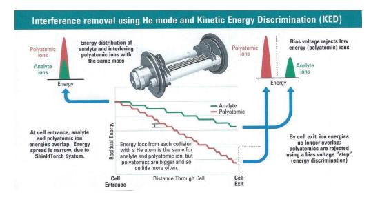
**FIGURE 9.56** The process of interference removal using He mode and kinetic energy discrimination in an octopole reaction cell. (© 2020 Agilent Technologies [www.agilent.com/chem]. All rights reserved. Used with permission.)
