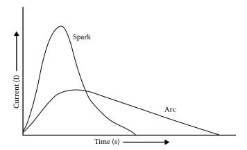
**FIGURE 7.9** Current-time relationship for a spark discharge and an arc discharge. (From Thomsen, used with permission from ASM International\*.)
