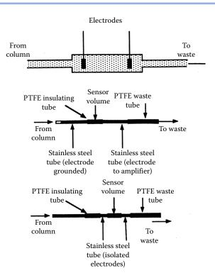
**FIGURE 12.19** Three conductometric detector designs. (Scott, used with permission.)
