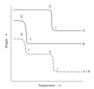
**FIGURE 14.7** TGA thermal curves for (top) pure A, (middle) pure B, and (bottom dotted line) a mixture of A and B. Because A and B have unique temperatures at which mass is lost, the composition of the mixture may be determined.
