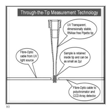
**FIGURE 3.34** (a) The AstraGene iCF UV/Vis spectrophotometer with the pipette being placed in the stand. (b) The pipette containing the sample in place for measurement. (c) Schematic of the "through the tip" technology. (©AstraNet systems, ltd., www.astranetsystems.com, www.norsci.ca. Used with permission.)
