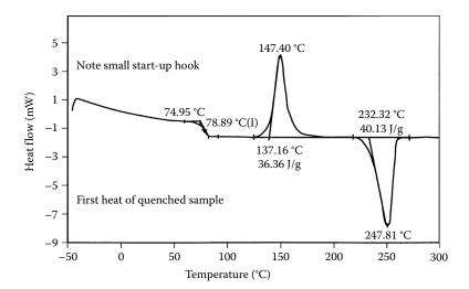
**FIGURE 14.22** DSC thermal curve for a sample of polyethylene terephthalate (PET).  $T_{\rm g}$  is observed at 78.9 °C. Crystallization begins at 137 °C and the area under the exothermic peak is equivalent to 36.36 J/g PET. Melting begins at about 323 °C; the area under the endothermic peak is equivalent to 40.13 J/g PET. (Courtesy of TA instruments, New Castle, DE, www.tainstruments.com.)
