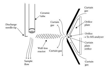
**FIGURE 12.24** Diagram of atmospheric pressure chemical ionization LC-MS interface. (Adapted with permission from applied biosystems, San Francisco, CA and MDS SCIEX, Vaughn, Ontario, Canada.)
