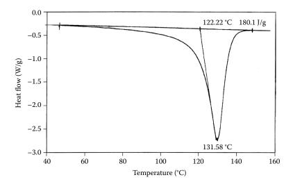
**FIGURE 14.25** Melting point of a polyethylene sample by DSC. (Courtesy of TA instruments, New Castle. From thermal analysis applications brief TA-123. www.tainstruments.com.)
