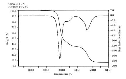
**FIGURE 14.14** TGA (solid line) and DTG (dotted line) thermal curves of polyvinylchloride polymer heated under nitrogen. The first mass loss at 280 °C is due to loss of HCl. (© 2020 PerkinElmer, inc. All rights reserved. Printed with permission. [www.perkinelmer.com].)
