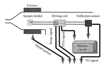
**FIGURE 14.27** A schematic simultaneous TGA-DTA instrument. A weight change on the sample side displaces the beam and a drive coil current returns the beam to zero. The current is proportional to the weight change and serves as the TGA signal. The temperature change between the sample and reference pans is measured by thermocouples attached to the pans. The temperature differential is the DTA signal.
