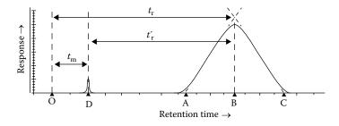
**FIGURE 10.9** Chromatogram with a single eluted peak; Peak position and shape terms.
