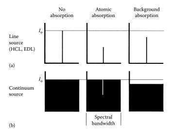
**FIGURE 6.25** (a) Atomic and background absorption with a line source (HCL, EDL). (b) Atomic and background absorption with a continuum source (deuterium lamp, tungsten-filament lamp). The width (x-axis) of each diagram is the spectral slit width. (© 1993-2020 PerkinElmer, inc. All rights reserved. Printed with permission. [www.perkinelmer.com].)
