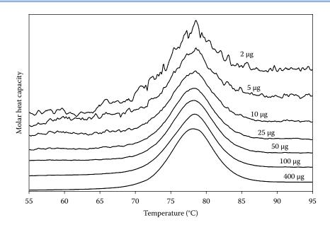
**FIGURE 14.37** A temperature scan, converted to molar heat capacity, for hen egg white lysozyme solution in 0.2 M glycine buffer, pH 4.0. Lysozyme concentrations ranged from 400  $\mu$ g to 2  $\mu$ g in the 300  $\mu$ L sample cell of the nano DSC. Curves are offset to see them clearly. (Courtesy of TA instruments, New Castle, DE. www.tainstruments.com.)
