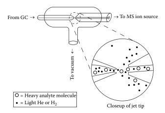
**FIGURE 11.25** Diagram of GC-MS jet separator interface operation.
