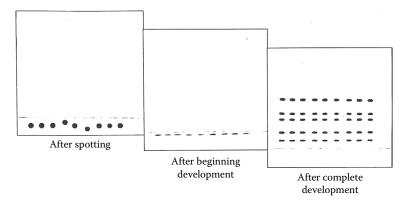
**FIGURE 12.44** Steps in development of a TLC chromatogram.
