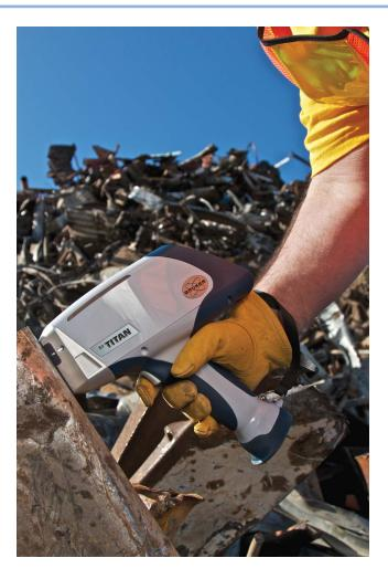
**FIGURE 8.54** Scrap metal sorting using the TITAN, a handheld XRF analyzer (HHXRF), to identify elemental composition. (Courtesy of Bruker Elemental, © 2020 Bruker, Inc. [www.bruker.com]. Used with permission.)
