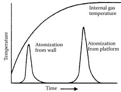
**FIGURE 6.22** Tube wall and platform temperature profiles. (© 1993-2020 PerkinElmer, inc. All rights reserved. Printed with permission. [www.perkinelmer.com.].)
