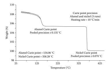
**FIGURE 14.5** The TGA curie point method records for each standard an apparent sharp weight change at a well-defined temperature, which corresponds to a known transformation in the standard's ferromagnetic properties at that temperature. The figure shows the relative temperature precision from three replicate calibration runs using alumel and nickel Curie point standards. (Courtesy of TA instruments, New Castle, DE, www.tainstruments.com.)
