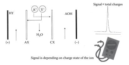
**FIGURE 12.20** Charge detector (QD) operation diagram. (© Thermo Fisher Scientific (www. thermofisher.com). Used with permission.)
