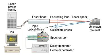
**FIGURE 7.51** LIBS schematic showing the major components. (Image reproduced courtesy of Applied Photonics Ltd., UK [www.appliedphotonics.co.uk].)
