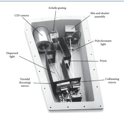
**FIGURE 7.15** Photograph of the interior of a commercial Echelle system with a CID detector. (© Thermo Fisher Scientific (www.thermofisher.com). Used with permission.)
