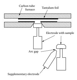
FIGURE 6.10 High-temperature furnace atomizer designed and used by L'vov.
