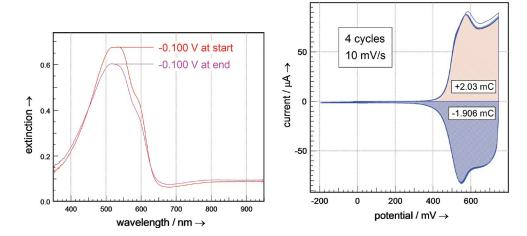
**FIGURE 13.41** Plots of stability (left) and electrochemical reversibility (right) of the model organic solar cell system. Note that the reversibility is shown as a plot of current versus potential and has the same form as a cyclic voltammogram. (Courtesy of C.-A. Schiller, ZAHNER-Elektrik GmbH & Co. KG. \*ZAHNER-Elektrik GmbH & Co. KG, Kronach, Germany [www.zahner.de].)
