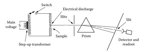
**FIGURE 7.5** Schematic diagram of an emission spectrometer with an electrical discharge excitation source. The prism is meant only to illustrate a dispersive device; a diffraction grating is used in all modern spectrometers with a single dispersive device. Echelle spectrometers use two dispersive devices, either a prism and a grating or two gratings.
