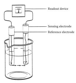
**FIGURE 13.6** An electrochemical measuring system for potentiometry. The indicator (sensing, working) electrode responds to the activity of the analyte of interest. The potential difference developed between the reference electrode and the indicator electrode is "readout" on the potentiometer (voltmeter). (© Thermo Fisher Scientific [www.thermofisher.com]. Used with permission.)
