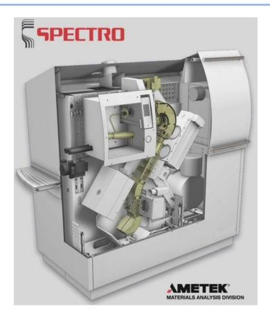
**FIGURE 9.24** Cutaway view of the SPECTRO MS, showing the ICP torch box upper left, the ion optic to the right of the torch box, leading to the mass spectrometer on the left under the torch box. (Courtesy of SPECTRO analytical instruments, inc., AMETEK® materials analysis division [www.spectro.com, www.ametek.com]. Used with permission.)
