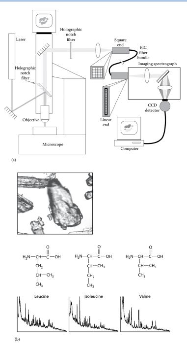
**FIGURE 4.56** (a) Schematic of the NIRIM. (b) Imaging and identification of three different amino acid crystals in a mixture using the NIRIM system. (Both reprinted from McLain et al., with permission from Advanstar Communications, Inc.)
