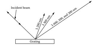
**FIGURE 2.17** The angle of diffraction of light from a grating depends not only on the wavelength but also on the *order of diffraction, n*. Wavelengths of 200, 300, and 600 nm are diffracted at different angles in first order (n = 1), but 200 nm light in third order (n = 3) and 300 nm light in second order (n = 2) diffract at the same angle as 600 nm light in first order. The three wavelengths overlap.
