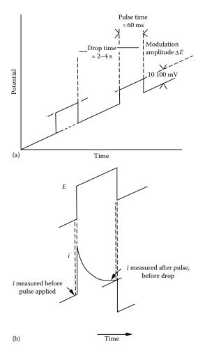
**FIGURE 13.32** Differential pulse polarography (not to scale). **(a)** Voltage vs. time sequence in DPP and **(b)** current response vs. time during DPP pulse.
