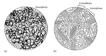
**FIGURE 14.17 (a)** Amorphous polymer structure **(b)** semicrystalline polymer structure with aligned chains in the crystalline regions and random structure in the amorphous region.
