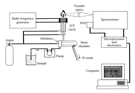
**FIGURE 7.21** Major components and layout of a typical ICP-OES instrument. (© 1999-2020 PerkinElmer, inc. All rights reserved. Printed with permission. [www.perkinelmer.com].)
