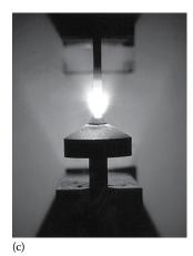
**FIGURE 7.7** (a) and (b) Photographs of the electrode assembly in commercial DC arc emission spectrometers. (c) Photograph of the plasma formed by the DC arc in operation. The discharge is established in the gap between the electrodes.
