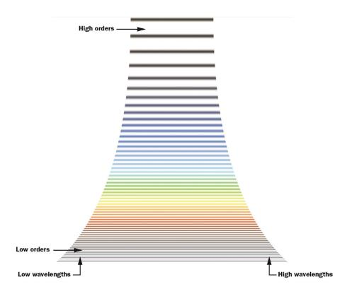
**FIGURE 7.16** Exit plane representing the 2D array of wavelengths produced by the Echelle configuration (an "Echellogram"). (Courtesy of SPECTRO, a unit of the materials analysis division of AMETEK, Inc., www.spectro.com, used with permission.)
