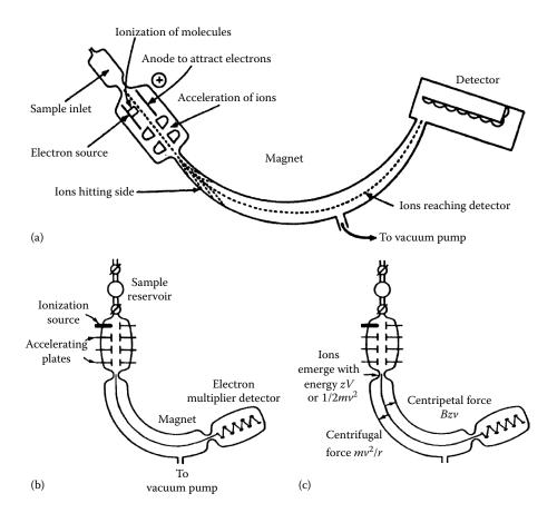
**FIGURE 9.1** (a) Schematic magnetic sector mass spectrometer. (b) Schematic magnetic sector mass spectrometer showing a gas sample reservoir with fill and inlet valves and an electron multiplier (EM) detector. (c) Forces and energies associated with ions traveling through a magnetic sector mass spectrometer. For an ion to reach the detector, Bzv must equal mv²/r.
