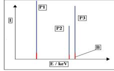
**FIGURE 8.9** Schematic comparison of EDXRF and WDXRF. The upper squares show the differences in instrument configuration, while the lower squares show the resulting spectra. B indicates the background radiation, while 1, 2, and 3 (P1, P2, P3) are photons of different energies.
