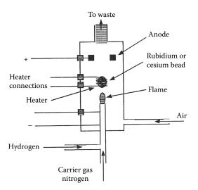
**FIGURE 11.22** Diagram of the nitrogen-phosphorus detector (NPD). (Cazes, used with permission.)
