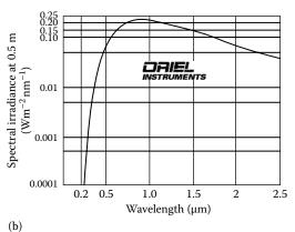
**FIGURE 4.8** (a) Commercial quartz tungsten-halogen lamps for use in the NIR region. The lamps are constructed of a doped tungsten coiled filament inside a quartz envelope. The envelope is filled with a rare gas and a small amount of halogen. (b) The spectral output of a model 6315 1000 W quartz tungsten-halogen lamp. The location and height of the peak depend on the model of lamp and the operating conditions. (Courtesy of Newport Corporation, Irvine, CA [www.newport.com].)
