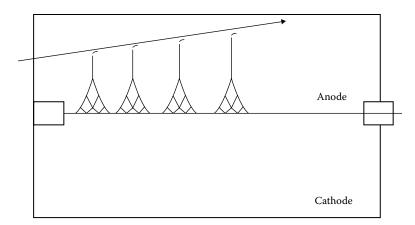
**FIGURE 8.39** Four primary ions pairs produce four "avalanches", all of which contribute to a single pulse. (Copyright Oak Ridge Associated Universities, www.orau.org.)
