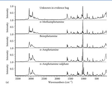
**FIGURE 4.48** (a) Raman spectra of an unknown material (top) and four related drug compounds. (b) The library search match numbers (second column) show that the unknown is very probably methamphetamine. Note that the entire analysis was performed in 30 seconds. (© Thermo Fisher Scientific [www.thermofisher.com]. Used with permission.)
