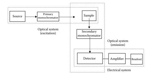
**FIGURE 3.46** Block diagram of the optical components of a typical fluorometer. (From Guilbault, used with permission.)
