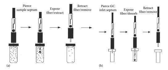
**FIGURE 11.6** Diagrams of SPME **(a)** Extraction sampling, and **(b)** GC desorption injection. (Used with permission from Sigma-Aldrich, a part of MilliporeSigma. www.sigmaaldritch.com. Copyright 2020 Sigma-Aldrich Co. LLC. All rights reserved.)
