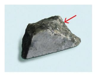
**FIGURE 4.60** A  $2 \times 2$  mm area at the indicated position was investigated on this inclined and rough rock sample while the sample was positioned under the microscope exactly as shown in the image. The height profile was measured by the integrated optical profilometer. (Courtesy of Frances Westall, CNRS Orleans, France and WITec GmbH, Ulm, Germany, www.WITec.de. Used with permission.)
