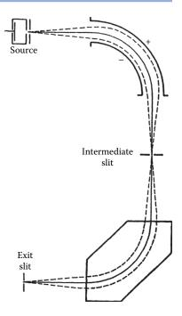
**FIGURE 9.20** A Nier-Johnson double focusing mass spectrometer. (From Ewing, used with permission.)
