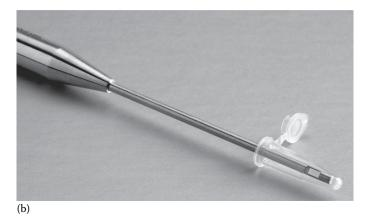
**FIGURE 3.29** (a) The evolution 300 with the rapid mixing accessory for fast kinetic studies in the UV/VIS region. (b) A fiber optic microprobe for UV/VIS determinations, shown in a PCR tube; 125  $\mu$ L of sample can be measured. (©Thermo fisher scientific inc., [www.thermofisher.com]. Used with permission.)
