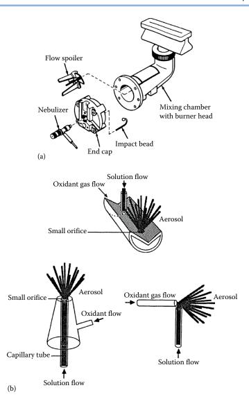
**FIGURE 6.8 (a)** Premix burner system. (© 1993-2020 PerkinElmer, inc. All rights reserved. Printed with permission. [www.perkinelmer.com].). **(b)** Schematic nebulizer designs. (Top): modified Babington type; (Left) concentric (the most common in FAAS); (Right) cross-flow type. (From Parsons, used with permission.)
