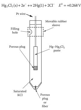
**FIGURE 13.5** The saturated calomel electrode (SCE). (Aikens et al., by permission, Waveland Press Inc., Long Grove, IL, 1984. All rights reserved.)
