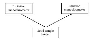
**FIGURE 3.47** Front surface fluorescence geometry for a solid sample. (From Froelich and Guilbault, used with permission.)
