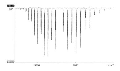
**FIGURE 14.31** Gas phase FTIR spectrum of HCl.
