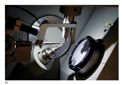
**FIGURE 8.67** (a) A benchtop single crystal XRD system, the Rigaku XtaLAB mini™. (b) Close-up of the goniometer, X-ray tube, and detector in the XtaLAB mini™. The single crystal sample is mounted at the tip of what looks like a sewing needle in the center of the photo. (Used by permission of Rigaku Corporation [www.rigaku.com].)
