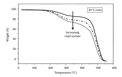
**FIGURE 14.9** TGA thermal curves of vinyl acetate copolymers. The weight loss at 340 °C is due to loss of acetic acid and gives a quantitative measure of the amount of vinyl acetate in the polymer. (Courtesy of TA instruments, New Castle, www.tainstruments.com.)
