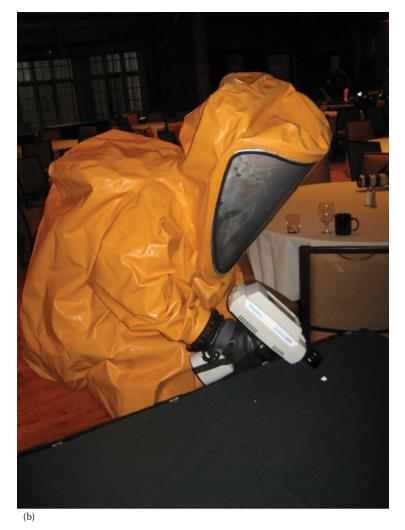
**FIGURE 4.45 (a)** Hand-held TruScan® Raman instrument collecting a spectrum from a powder sample directly through the plastic bag. (© Thermo Fisher Scientific [www.thermofisher.com]. Used with permission.) **(b)** Hazardous material identification by a first responder using the handheld FirstGuard™ 1064 nm advanced Raman system. (Used with permission of Rigaku Raman Technologies, Inc. [www.rigakuraman.Com].)
