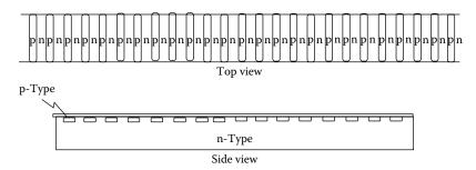
**FIGURE 3.24** A photodiode array. The top view shows the face that the light would fall on. The side view shows that the p-type elements are embedded in a continuous layer of n-type semiconductor. (From Brown, used with permission.)
