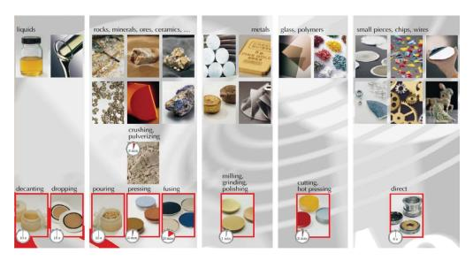
**FIGURE 8.49** Sample preparation techniques and sample holders for XRF analysis.
