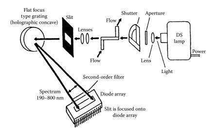
FIGURE 12.15 Schematic of diode array detector for HPLC. (Cazes, used with permission.)
