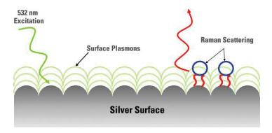
**FIGURE 4.50** The SERS process using 532 nm excitation of a silver substrate with adsorbed species (the circles). Surface plasmons interact with the adsorbed species to enhance the Raman emission, shown on the right side of the diagram. (© Thermo Fisher Scientific [www.thermo-fisher.com]. Used with permission.)
