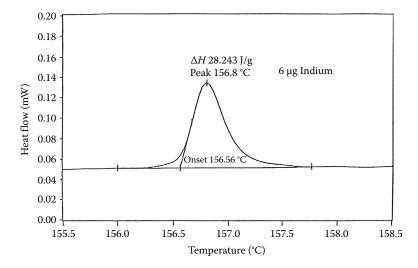
**FIGURE 14.21** DSC thermal curve showing the determination of the enthalpy of fusion of 6 μg of indium metal. (© 2020 PerkinElmer, inc. All rights reserved. Printed with permission. [www.perkinelmer.com].)
