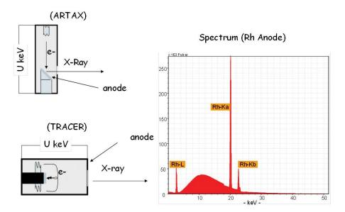
**FIGURE 8.12** Schematic diagrams of a Rh target side-window tube (ARTAX system) and a modern handheld transmission target design (TRACER system). (Courtesy of Roald Tagle, BRUKER NANO GmbH, Berlin. © 2020 Bruker, Inc. Used with permission.)
