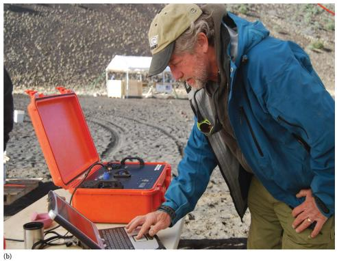
**FIGURE 8.74** (a) and (b) Two images of geologists using the terra Mobile XRF system in real mining applications in field conditions. (Courtesy of Olympus NDT [www.olympus-ims.com; www.inxitu.com].)
