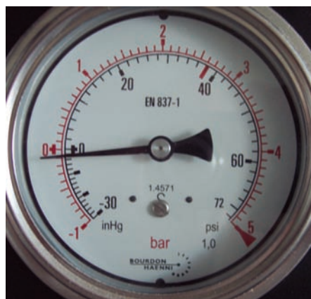
Figure 19.3 A pressure gauge on a modern vacuum-assisted autoclave. The red scale is in bar (see text) and the black scale above zero is calibrated in pounds per square inch. Note that the (black) vacuum scale (below zero) is in a third unit: inches of mercury.
