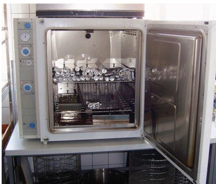
Figure 19.4 A laboratory-scale hot air sterilizer. Source: http://commons.wikimedia.org/wiki/File:Sterilisator_offen.jpg .
