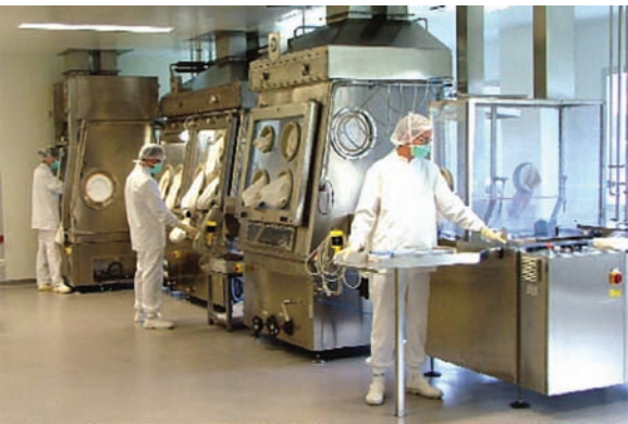
Figure 17.6 Three isolators used for filling cytotoxic injections. Pierre Fabre cytotoxic injectable filling line. Reproduced with kind permission from Pierre Fabre Médicament Production/Aquitaine Pharm International (API) ( www.aquitaine-pharm.com ).
