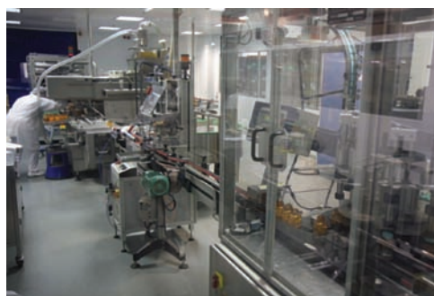
A medicines' filling line (largely enclosed to protect against contamination)
