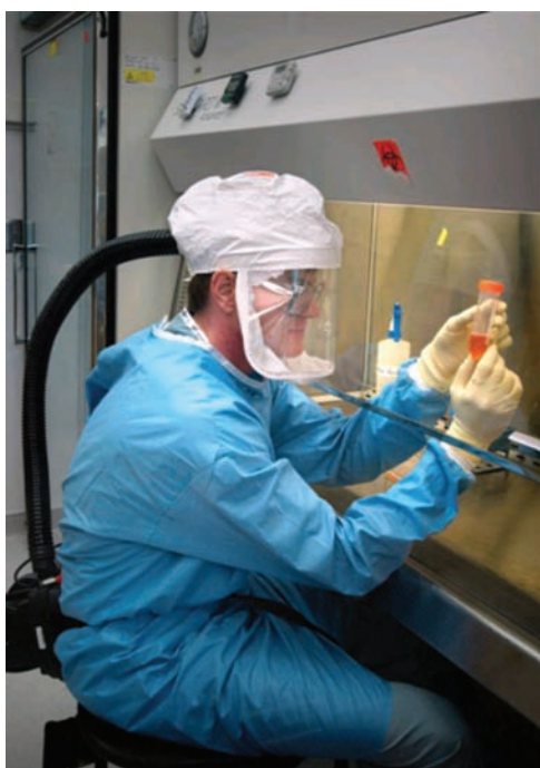
Figure 2.1 A microbiologist working with influenza virus using a class II safety cabinet in which the air is passed through filters to remove microorganisms. Source: PHIL ID #7988; Photo Credit: James Gathany, Centers for Disease Control and Prevention.
