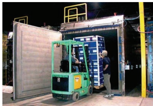
Figure 19.5 Loading an ethylene oxide sterilizer. Source: Image courtesy of Steris Corporation.
