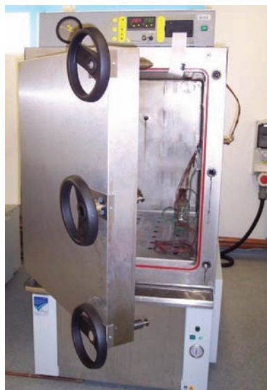
Figure 19.2 A front-loading laboratory autoclave having approximately four times the capacity of that in Figure 19.1. Note the thermocouple leads inside to record the temperature at different locations in the load.
