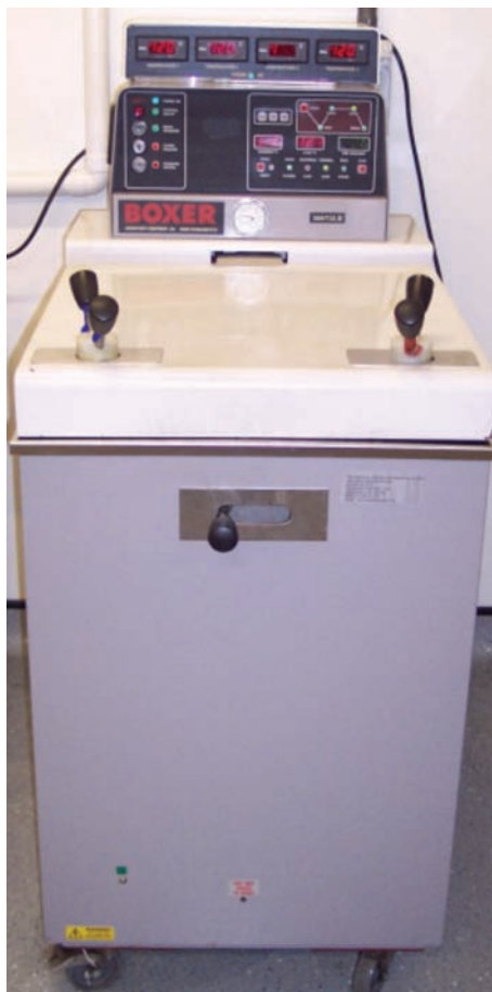
Figure 19.1 A small top-loading laboratory autoclave.
