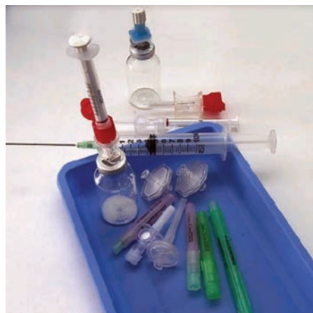
Figure 19.6 A selection of disposable units that fit onto syringes for sterilizing small volumes of liquid. Source: Image courtesy of Helapet Limited.
