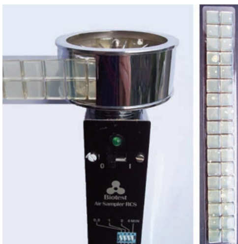
Figure 17.2 Biotest air sampler and (right, and not to scale) the agar strip after incubation on which bacterial colonies have grown. Before sampling, the strip is fed into the circular housing at the top of the instrument; this contains an impeller to suck in air which is blown against the moist agar surface of the strip. Dust and attached bacteria are caused to 'stick' to the agar and grow into visible colonies during incubation.
