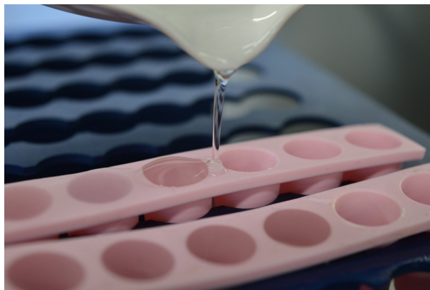
Figure 11 The suppository mold cavities are intentionally overfilled to account for contraction upon cooling.
