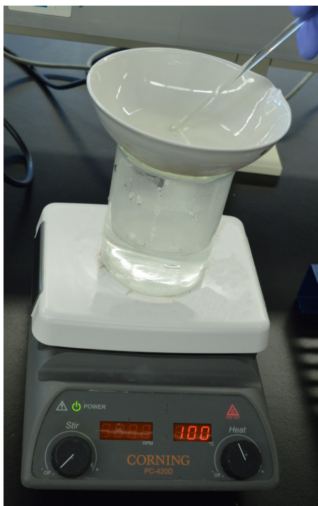
Figure 2 A steam bath is set up to limit direct exposure to heat from the hot plate. A ceramic dish is set on top of the steam bath to melt components of the formulation.
