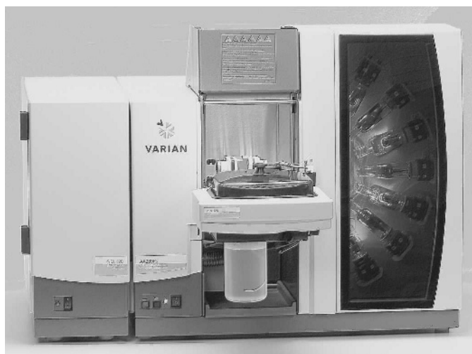
Figure 13.12 An AA spectrometer, Model AA 280 equipped with a graphite furnace and Zeeman device. A rotating turret holds height HCL (reproduced courtesy of Varian Inc.)
