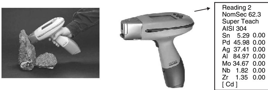
Figure 12.15 Portable field apparatus. This instrument represents a category of energy dispersive spectrometers equipped with an X-ray generator but no radioactive source (reproduced courtesy of Niton, USA). Type of information that can be obtained.
