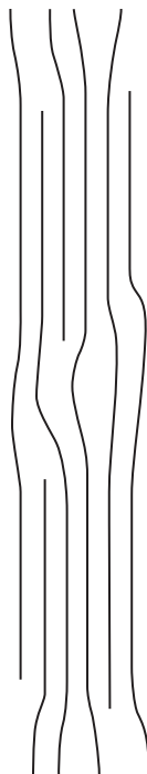
FIGURE 3.35 Crystalline regions in which the chains are parallel and ordered, separated by amorphous regions.
