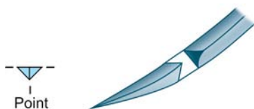
Figure 21.21: Reverse cutting needle
