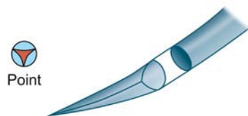
Figure 21.22: Taper cut needle
