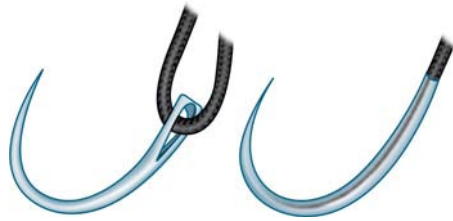
Figure 21.23: Eyed and eyeless needles
