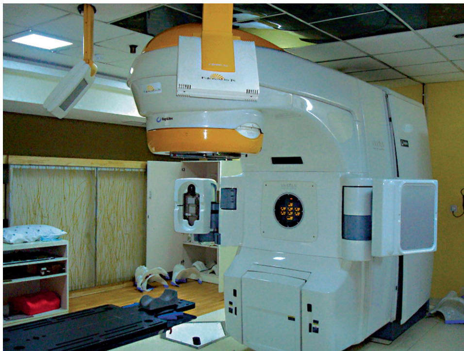
Figure 73.2. Novalis-Tx linear accelerator. Dual energy with photon and electron beam and 6D robotic couch. It is used for both cancerous and non-cancerous lesions. It generates photons (6 and 15 MV) and electrons (6, 9, 12, 15 and 18 MeV). It can be used for:
