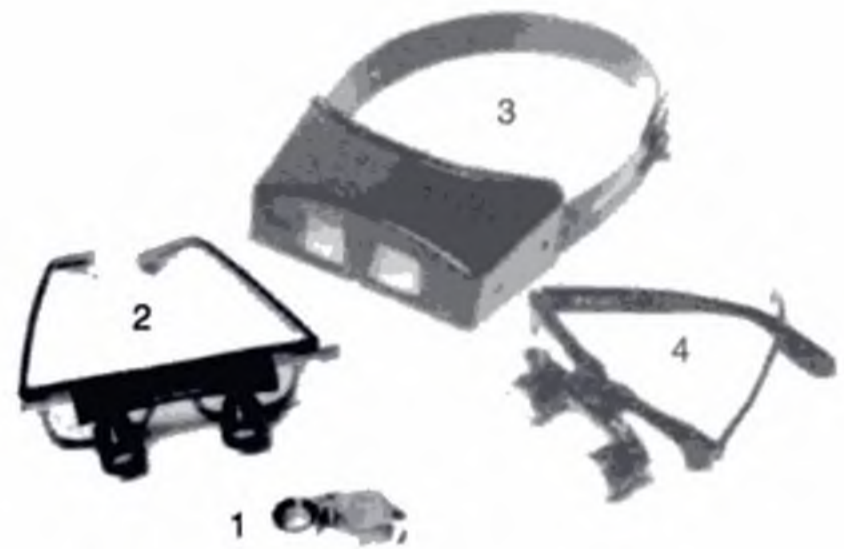
Fig. 33.1 Aids to produce magnification. 1, the 10x loupe used to examine the anterior segment of the eye; 2, inexpensive operating glasses (2x); 3, a simple magnifier with a head band; 4, the more sophisticated (and expensive) Keeler operating glasses (2x) (Galbraith).
