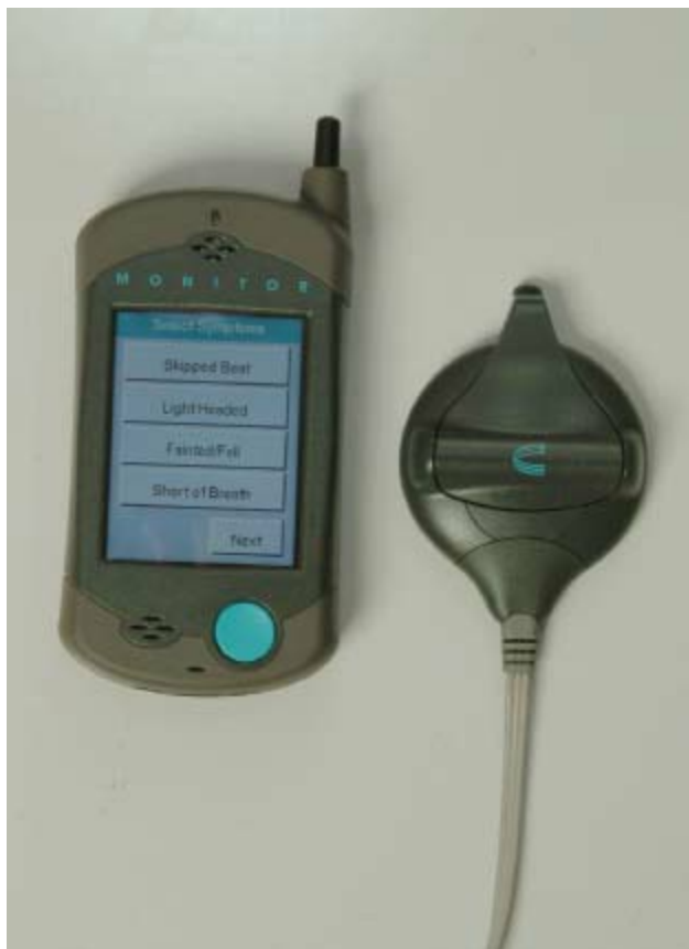
FIGURE 32.3 Cardionet ambulatory arrhythmia monitor.
