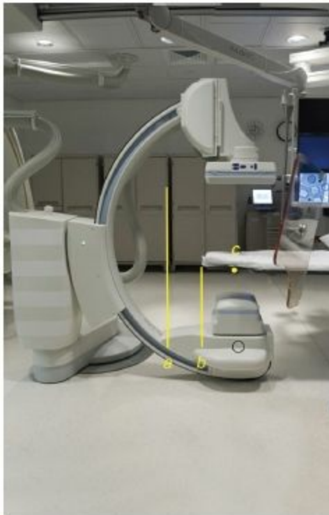
FIGURE 44.4 The x-ray focal spot is denoted on the fluoroscope by a small red dot on the x-ray tube housing (black circle). The source to image distance is the distance between the x-ray focal spot and the image receptor ( A ). The source to skin entrance distance is the distance between the x-ray focal spot and the table ( B ). The IRP is located at 15 cm below the isocenter of the C-arm, ( C ).
