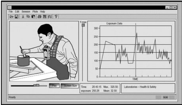
Fig 30.1 Video exposure monitoring. Combining a direct reading monitor with a video to examine the relationship between work practices and exposure.
