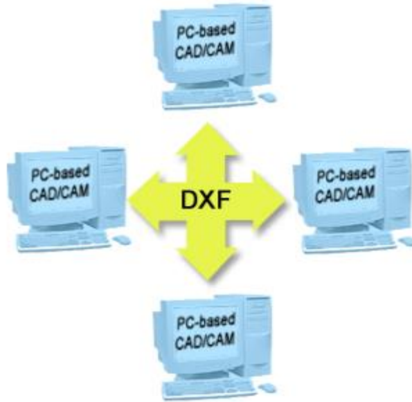
Figure 1. DXF allows the interchange of CAD data between different software packages.
