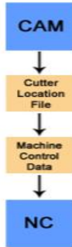
Figure 2. Post processing connects CAM and the CNC machine.
