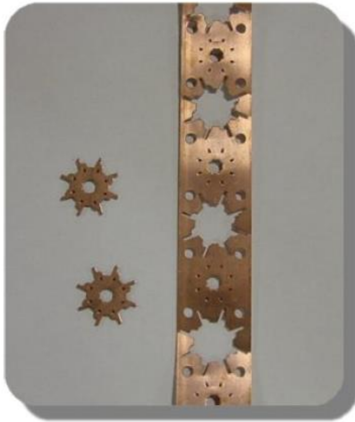
Figure 2. These parts were separated from the copper strip on a press.
