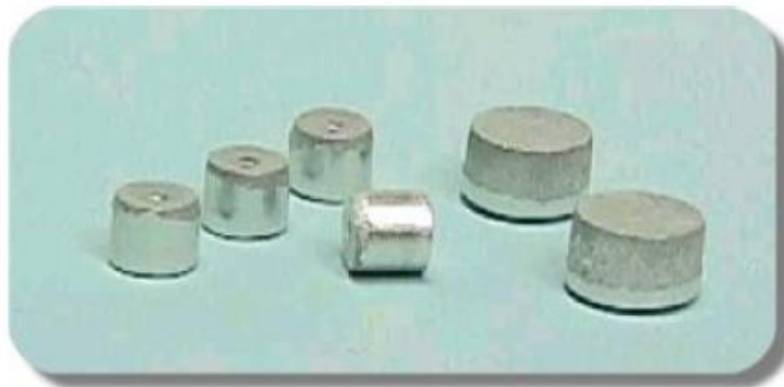
Figure 2. Metal slugs with visible deformation and tearing marks.
