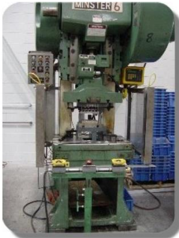
Figure 2. The C-shaped frame is very accessible.
