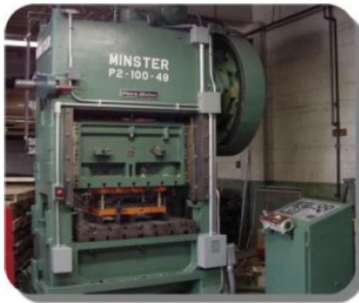
Figure 2. The straight-side press offers excellent rigidity.
