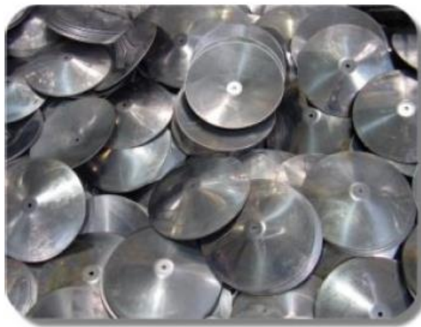
Figure 2. These parts were made by cold-working operations.
