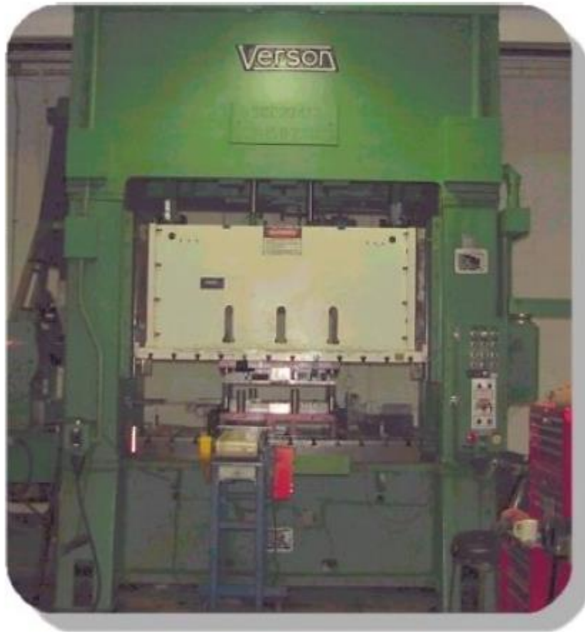
Figure 2. A 150-ton straight-side mechanical press.
