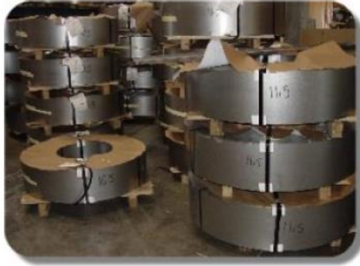
Figure 1. Sheet metal is sold in large coils.
