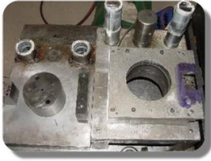
Figure 3. Disassembled upper and lower die shoes.
