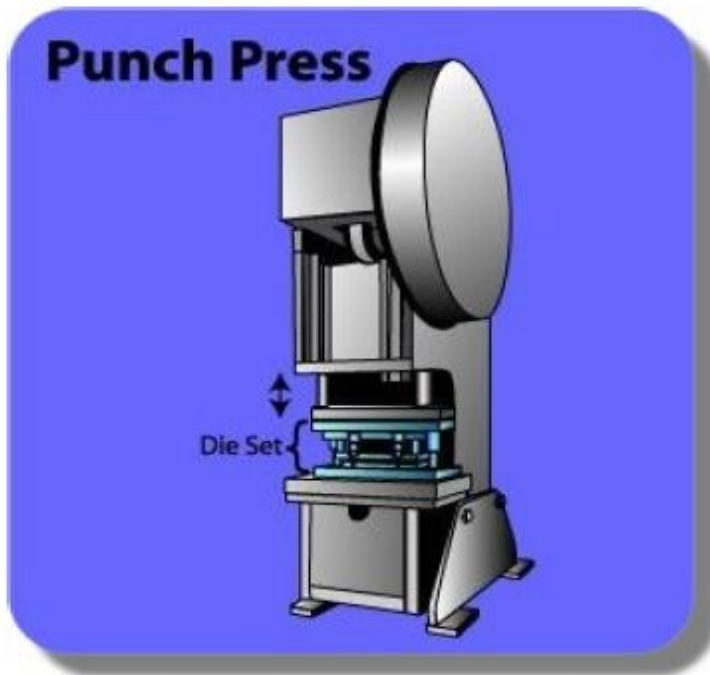
Figure 1. The die set is positioned between the ram and the bolster plate.
