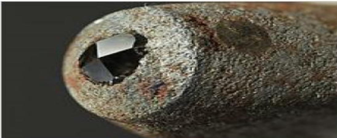
The pyramidal diamond indenter of a Vickers hardness tester.
