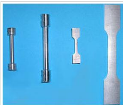
Tensile specimens made from an aluminum alloy. The left two specimens have a round cross-section and threaded shoulders. The right two are flat specimen designed to be used with serrated grips.
