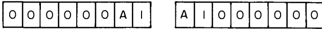
Figure 2.26 Identifier A1 right and left justified and zero filled (6 bits per character)
