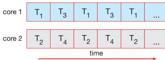
Figure 4.4 Parallel execution on a multicore system.
