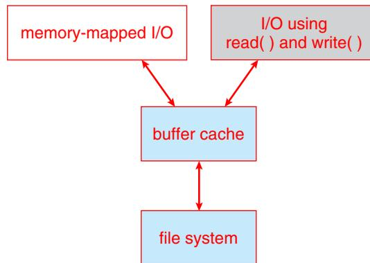
**Figure 14.11** I/O using a unified buffer cache.
