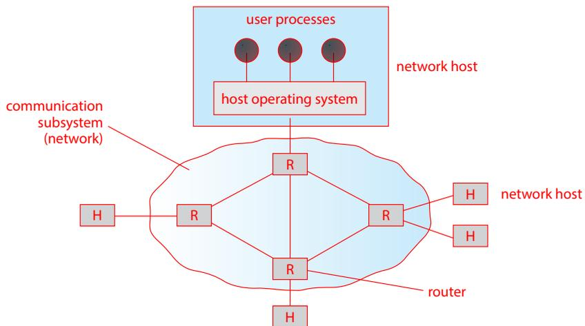
**Figure 19.3** Communication processors in a wide-area network.
