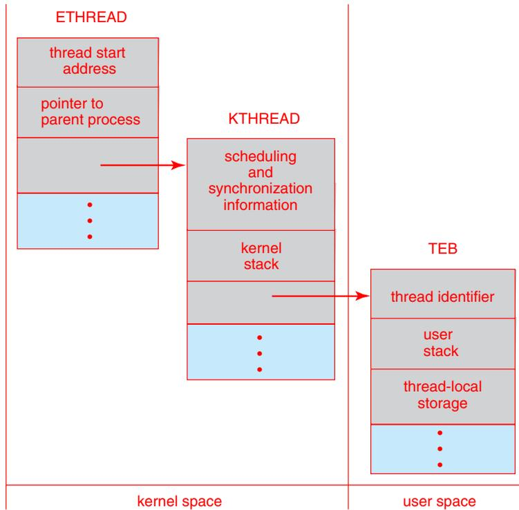
**Figure 4.21** Data structures of a Windows thread.
