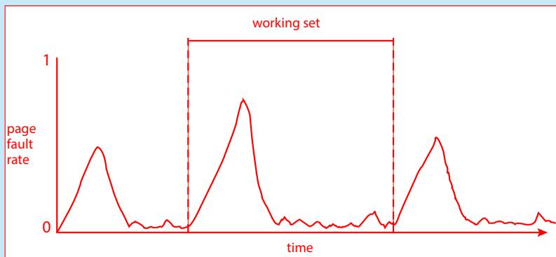
A peak in the page-fault rate occurs when we begin demand-paging a new locality. However, once the working set of this new locality is in memory, the page-fault rate falls. When the process moves to a new working set, the page-fault rate rises toward a peak once again, returning to a lower rate once the new working set is loaded into memory. The span of time between the start of one peak and the start of the next peak represents the transition from one working set to another.
