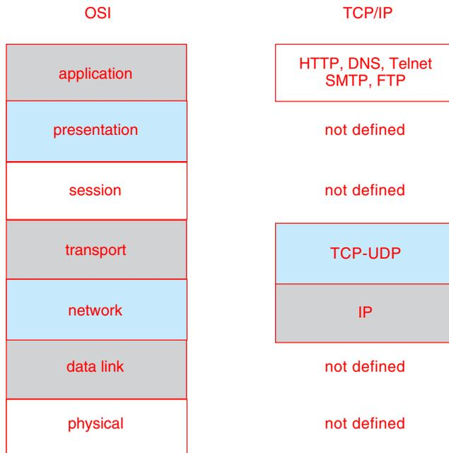
**Figure 19.8** The OSI and TCP/IP protocol stacks.
