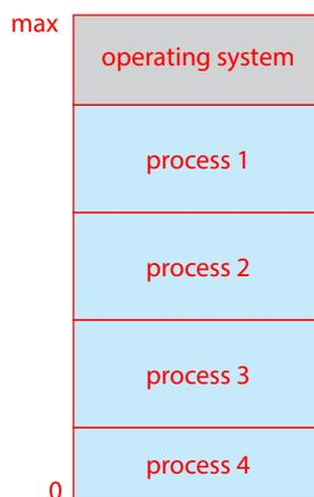
**Figure 1.12** Memory layout for a multiprogramming system.
