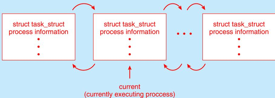
As an illustration of how the kernel might manipulate one of the fields in the `task_struct` for a specified process, let's assume the system would like to change the state of the process currently running to the value `new_state`. If `current` is a pointer to the process currently executing, its state is changed with the following:
