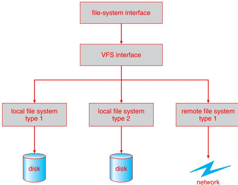
**Figure 15.5** Schematic view of a virtual file system.
