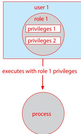
**Figure 17.10** Role-based access control in Solaris 10.
