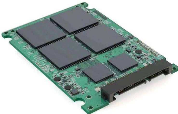
**Figure 11.3** A 3.5-inch SSD circuit board.
