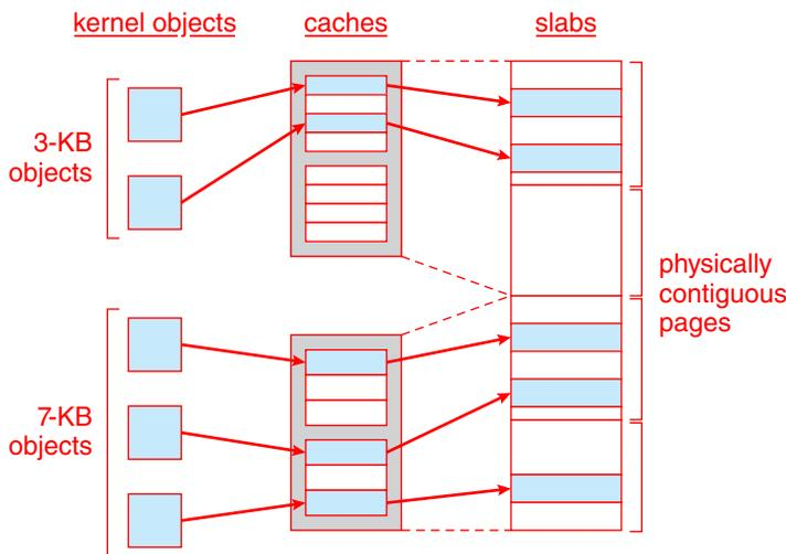
**Figure 10.27** Slab allocation.
