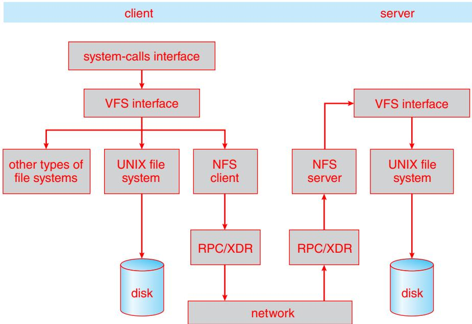
**Figure 15.8** Schematic view of the NFS architecture.
