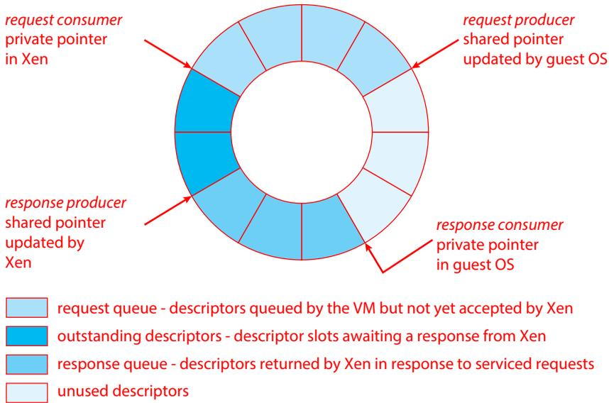
**Figure 18.6** Xen I/O via shared circular buffer.<sup>1</sup>
