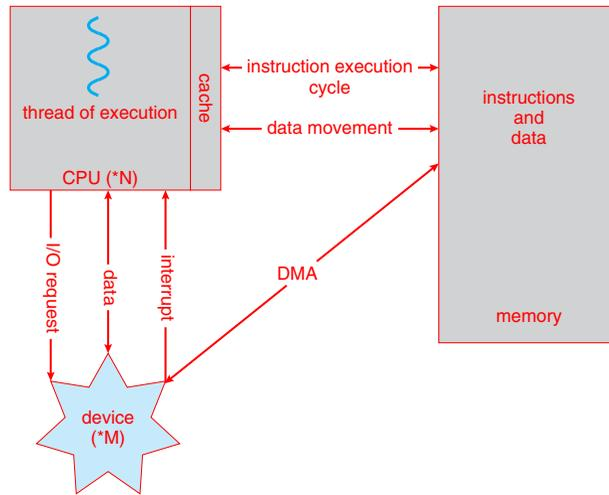
**Figure 1.7** How a modern computer system works.
