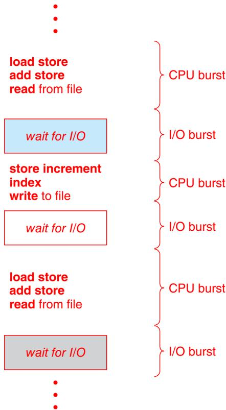
Figure 5.1 Alternating sequence of CPU and I/O bursts.
