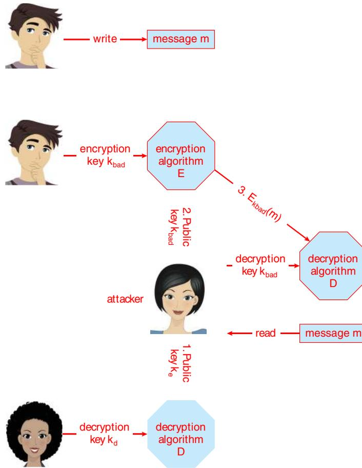
Figure 16.9 A man-in-the-middle attack on asymmetric cryptography.<sup>4</sup>
