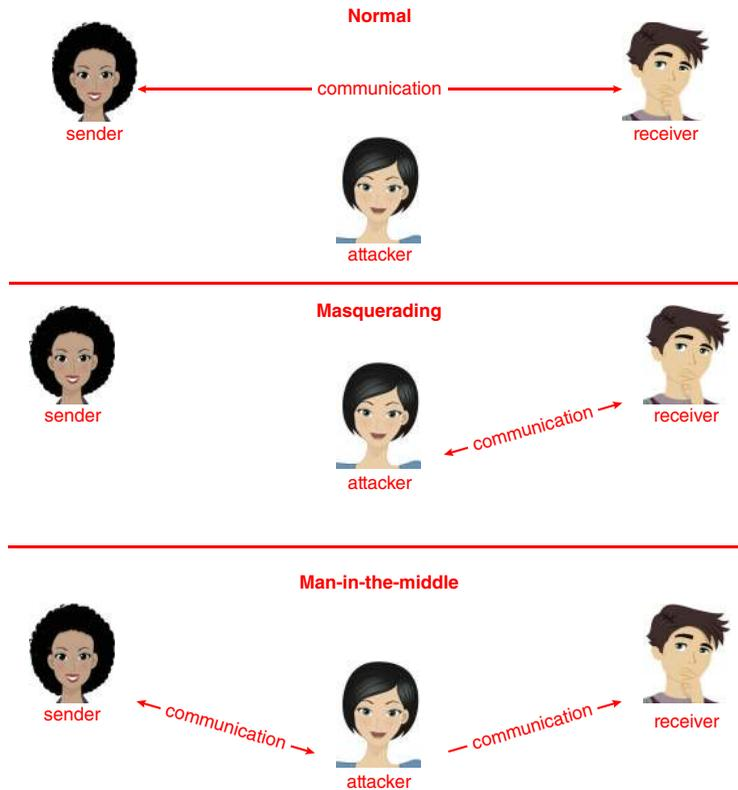
Figure 16.6 Standard security attacks.<sup>1</sup>
