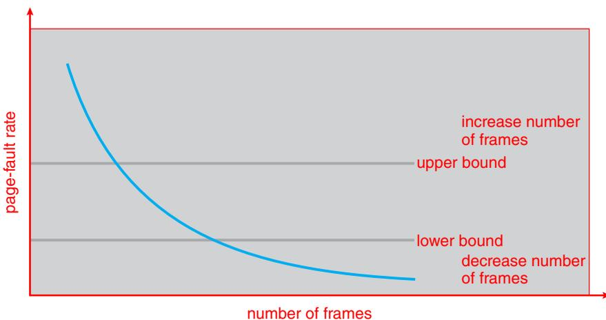
Figure 10.23 Page-fault frequency.
