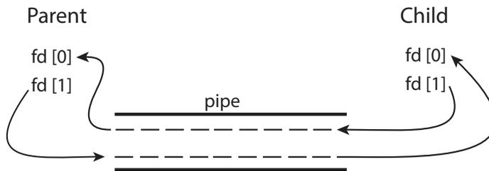
**Figure 3.20** File descriptors for an ordinary pipe.
