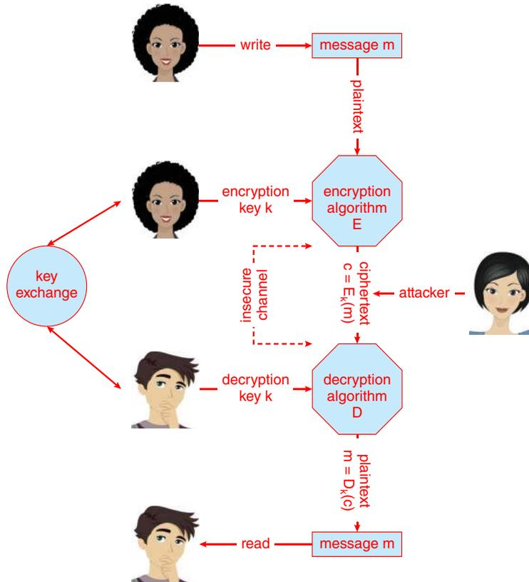
Figure 16.7 A secure communication over an insecure medium.<sup>2</sup>
