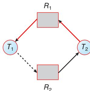
Figure 8.10 An unsafe state in a resource-allocation graph.
