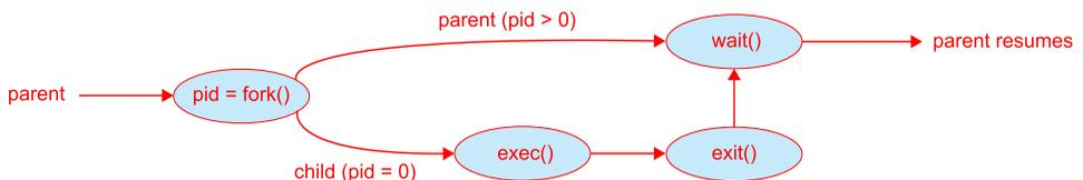
**Figure 3.9** Process creation using the `fork()` system call.
