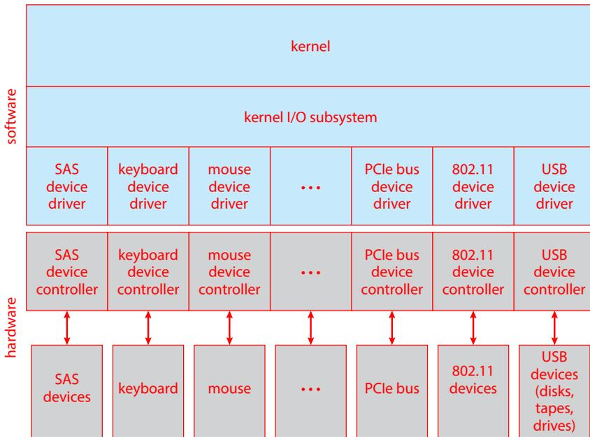
**Figure 12.7** A kernel I/O structure.
