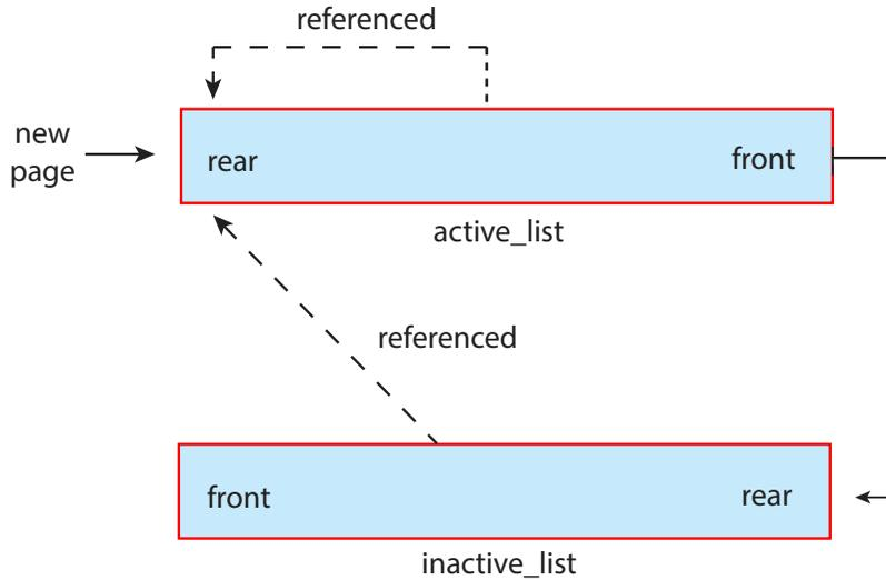
**Figure 10.29** The Linux `active_list` and `inactive_list` structures.
