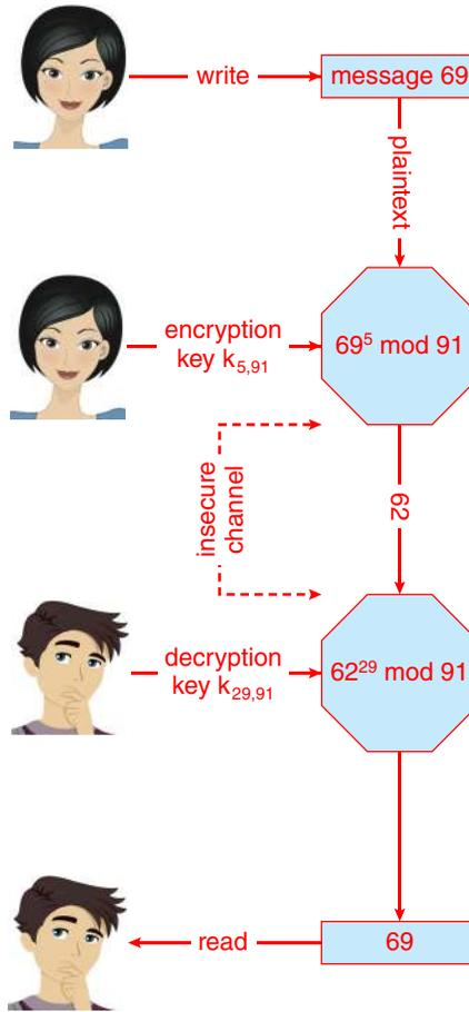
**Figure 16.8** Encryption and decryption using RSA asymmetric cryptography.<sup>3</sup>
