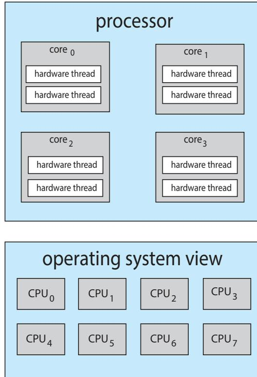
**Figure 5.14** Chip multithreading.
