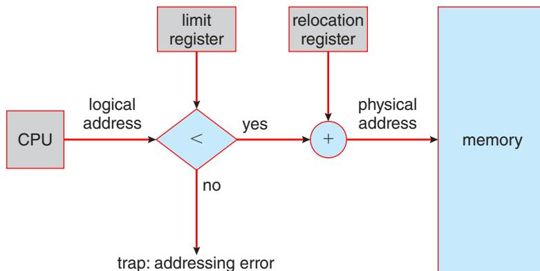
**Figure 9.6** Hardware support for relocation and limit registers.
