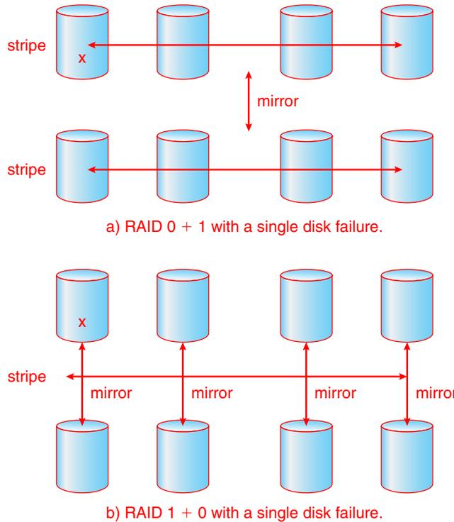
**Figure 11.16** RAID 0 + 1 and 1 + 0 with a single disk failure.
