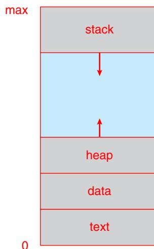
**Figure 3.1** Layout of a process in memory.
