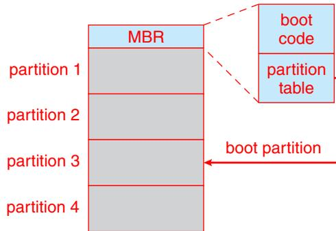
**Figure 11.10** Booting from a storage device in Windows.
