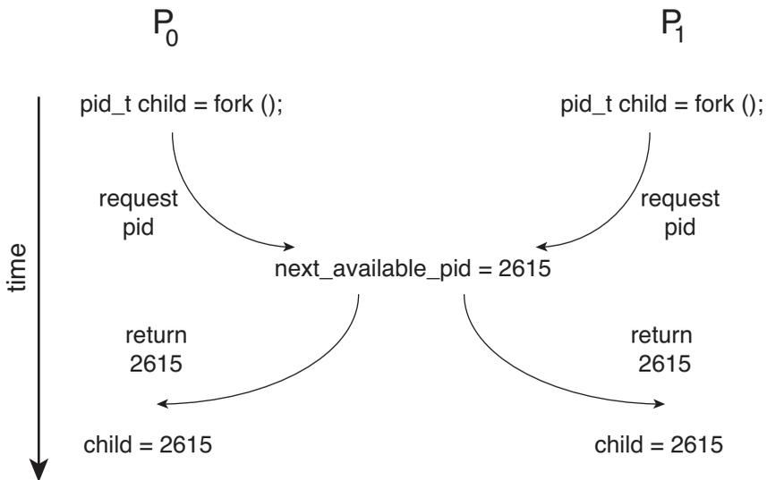
Figure 6.2 Race condition when assigning a pid.
