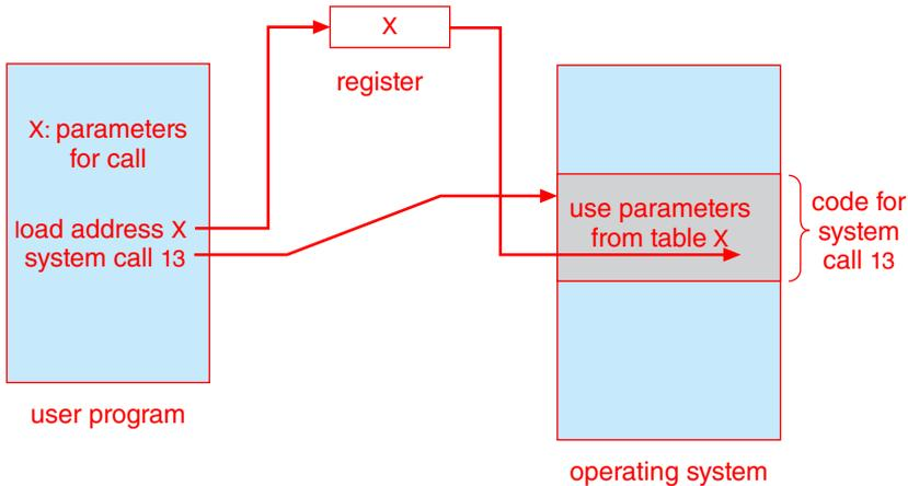
**Figure 2.7** Passing of parameters as a table.
