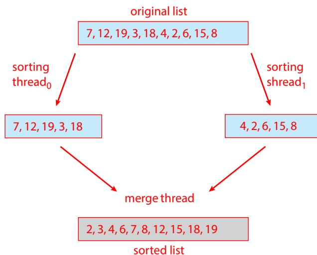
Figure 4.27 Multithreaded sorting.
