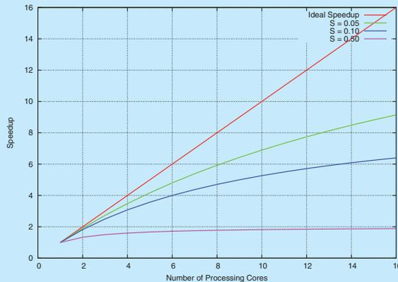
One interesting fact about Amdahl's Law is that as  $N$  approaches infinity, the speedup converges to  $1/S$ . For example, if 50 percent of an application is performed serially, the maximum speedup is 2.0 times, regardless of the number of processing cores we add. This is the fundamental principle behind Amdahl's Law: the serial portion of an application can have a disproportionate effect on the performance we gain by adding additional computing cores.
