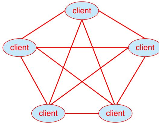
**Figure 1.23** Peer-to-peer system with no centralized service.
