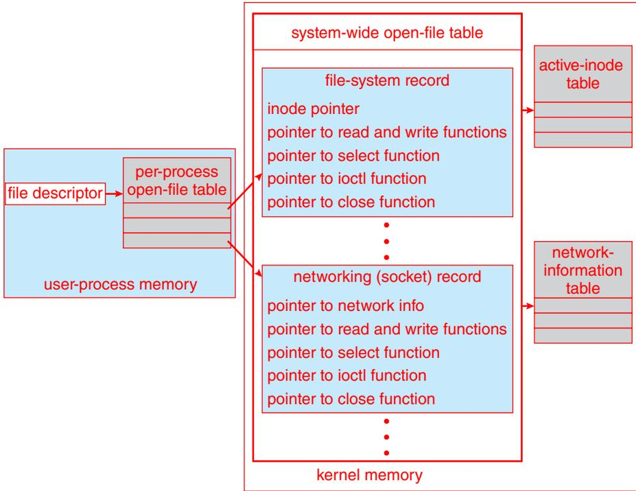
Figure 12.13 UNIX I/O kernel structure.
