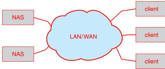
**Figure 11.12** Network-attached storage.
