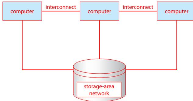
Figure 1.11 General structure of a clustered system.
