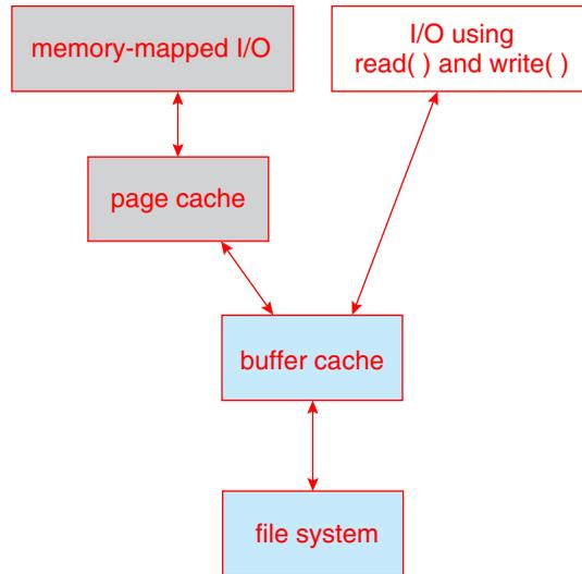
**Figure 14.10** I/O without a unified buffer cache.
