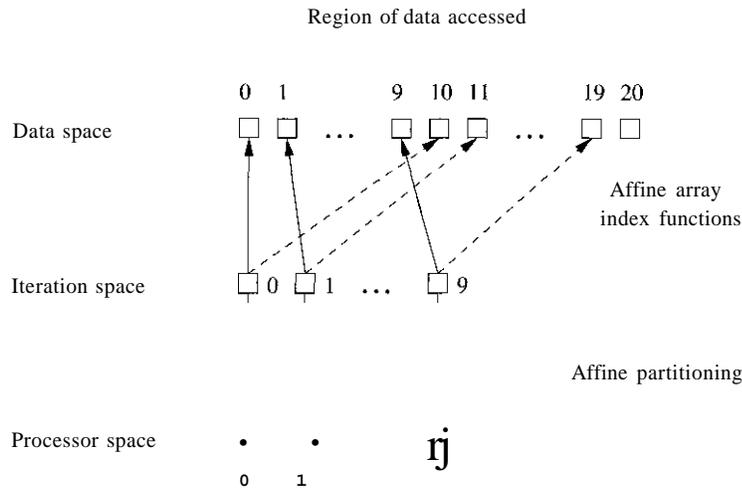
Figure 11.4: Iteration, data, and processor space for Example 11.4
