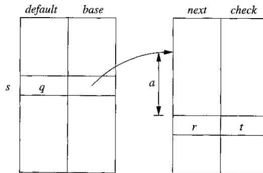
Figure 3.66: Data structure for representing transition tables
