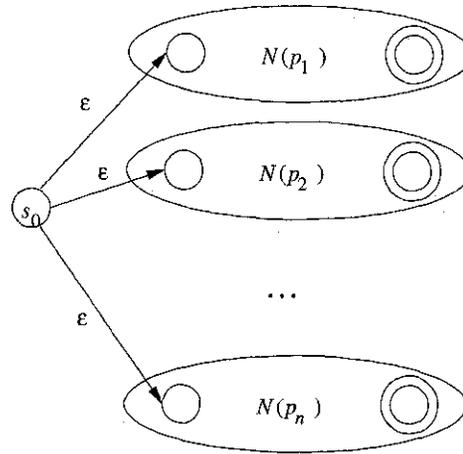
Figure 3.50: An NFA constructed from a **Lex** program
