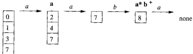
Figure 3.53: Sequence of sets of states entered when processing input **aaba**
