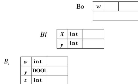
Figure 2.36: Chained symbol tables for Example 2.15
