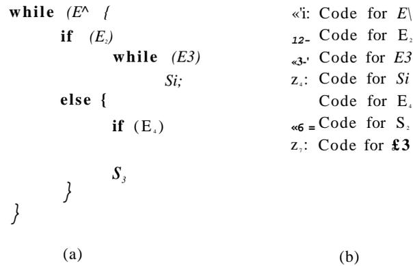
Figure 6.47: Control-flow structure of program for Exercise 6.7.2
