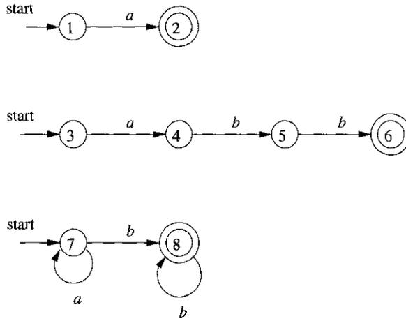
Figure 3.51: NFA's for **a**, **abb**, and **a\*b<sup>+</sup>**
