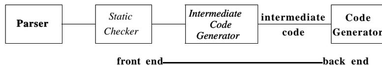
Figure 6.1: Logical structure of a compiler front end
