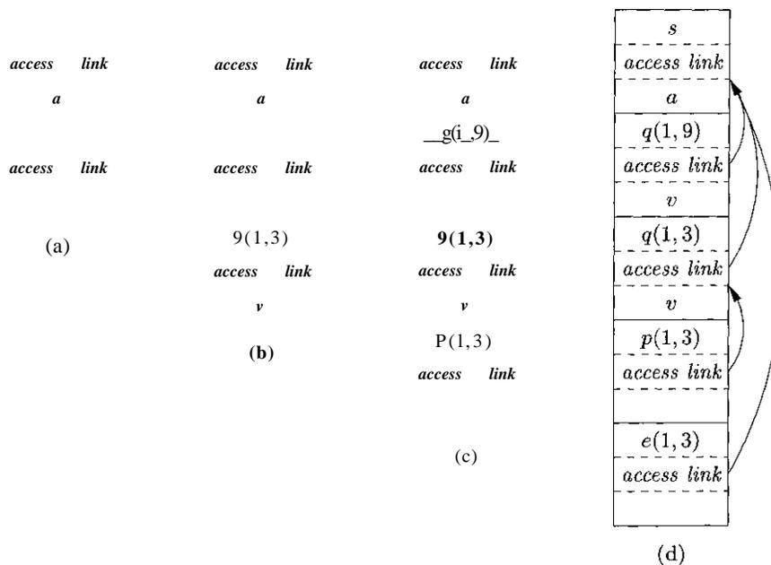
Figure 7.11: Access links for finding nonlocal data
