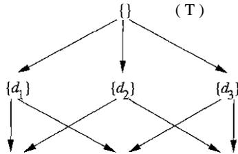
Figure 9.22: Lattice of subsets of definitions
