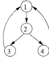
Figure 9.46: Two loops with the same header
