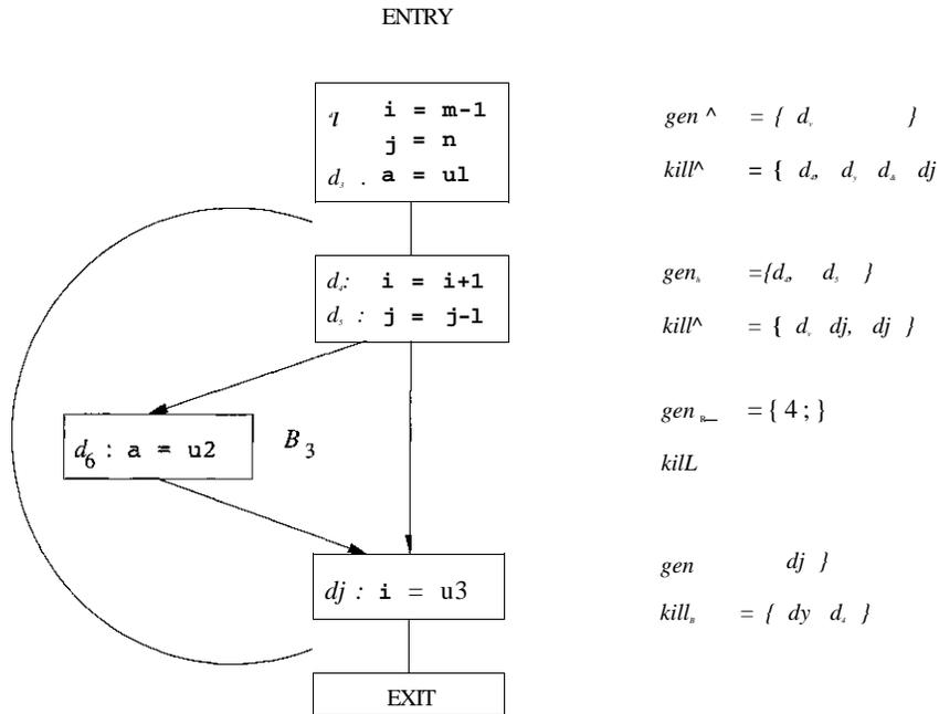
Figure 9.13: Flow graph for illustrating reaching definitions
