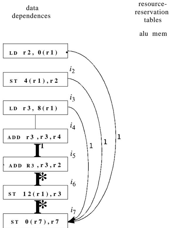
Figure 10.7: Data-dependence graph for Example 10.6
