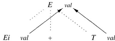
Figure 5.6:  $E.val$  is synthesized from  $Ei.val$  and  $Ei.val$
