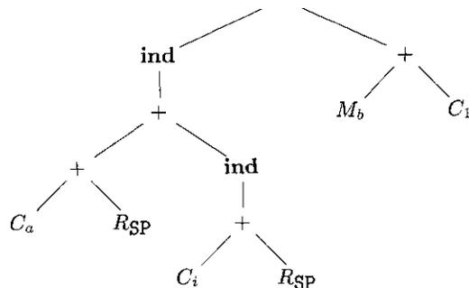
Figure 8.19: Intermediate-code tree for  $a[i] = b + 1$
