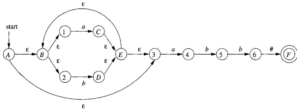
Figure 3.57: NFA constructed by Algorithm 3.23 for  $(a|b)^*abb\#$
