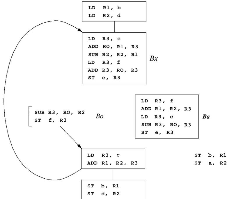
Figure 8.18: Code sequence using global register assignment
