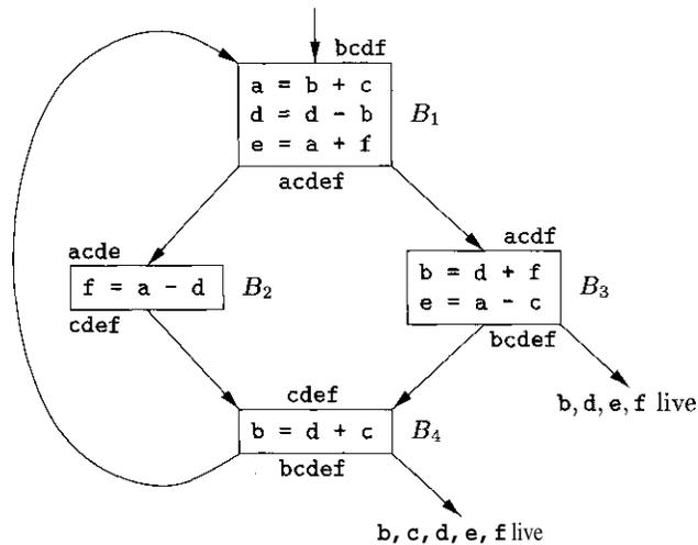
Figure 8.17: Flow graph of an inner loop
