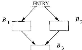
Figure 9.24: Flow graph illustrating the effect of early meet over paths
