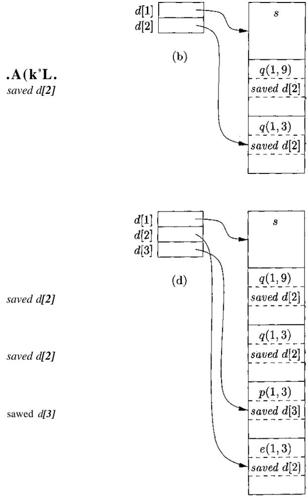
Figure 7.14: Maintaining the display
