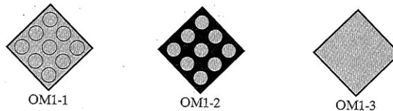
*Nine yellow retroreflectors with 3-in minimum diameter on a yellow or black diamond panel of 18 in or more on a side; or an all-yellow retro reflective diamond panel of the same size.*
