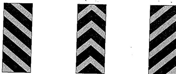
*A striped marker measuring 12 X 36 in with alternating black and yellow stripes sloping downward at an angle of 45° toward the side of the obstruction on which traffic is to pass.*
