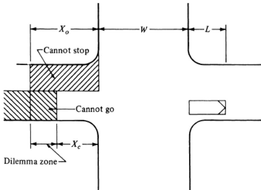
Figure 5.10 schematic of a dilemma zone.
