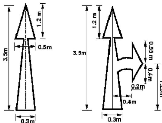
Figure 5.7 A typical example of a directional arrow
