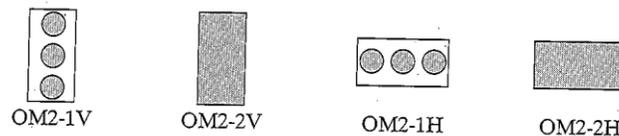
*Three yellow retroreflectors with 3-in minimum diameter arranged horizontally or vertically on white panel of at least 6 X 12 in; or an all- yellow retroreflective panel of the same size.*
