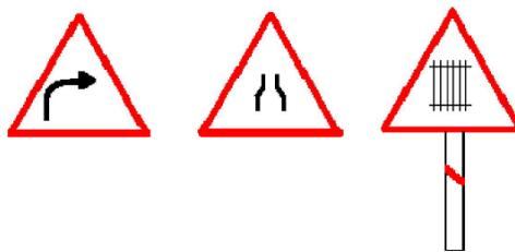
Figure 5.8: Examples of cautionary signs ( right hand curve sign board, signs for narrow road, sign indicating railway track ahead)
