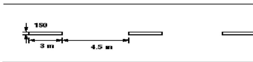
**Figure 5.1:** Centre line marking for a two lane road
