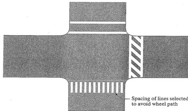
**Figure 5.5:** Pedestrian marking near an intersection
