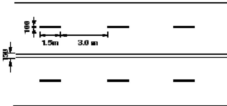
**Figure 5.3:** Double solid line for a two lane road
