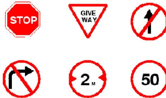
**Figure 5.7:** Examples of regulatory signs ( stop sign, give way sign, signs for no entry, sign indicating prohibition for right turn, vehicle width limit sign, speed limit sign)
