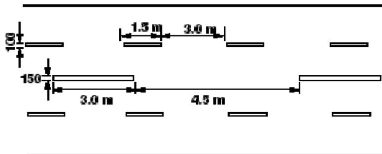
**Figure 5.2:** Centre line and lane marking for a four lane road
