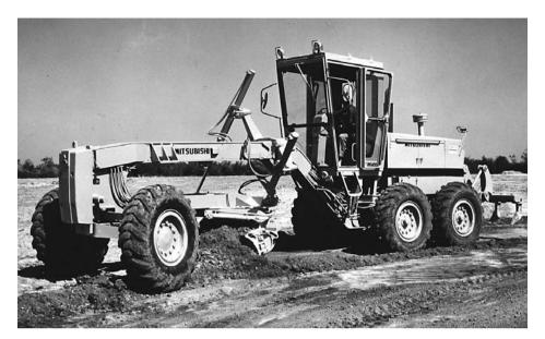
Figure 17.14 Typical Motor Grader
