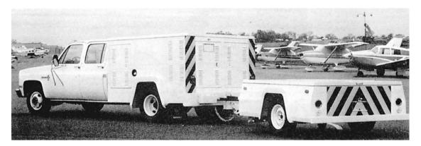
Figure 21.12 Locked-Wheel Skid Trailer
