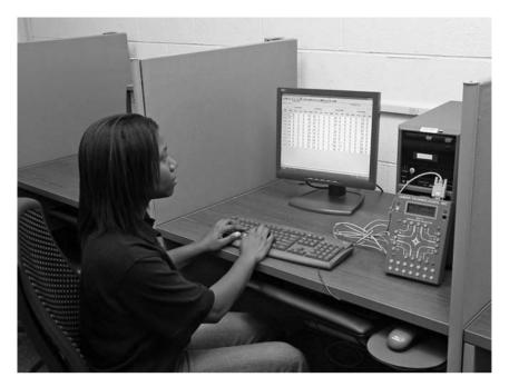
Figure 4.7 Jamar Traffic Data Collector TDC-12 Hooked to a Computer
