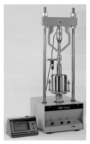
Figure 17.17 CBR Testing Equipment
