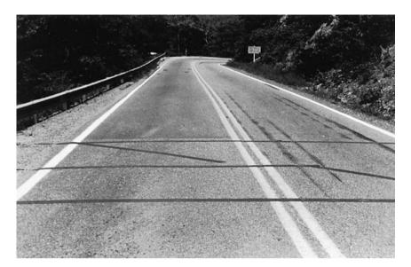
**Figure 4.8** An Example of a Sensor Setup of a Surface Detector Using Pneumatic Road Tubes SOURCE: Photograph by Lewis Woodson, Virginia Transportation Research Council, Charlottesville, VA.
