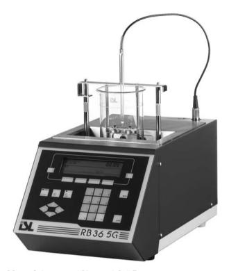
Figure 18.6 The RB36 5G Automated Ring-and-Ball Tester
