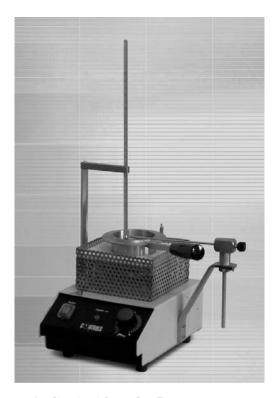
Figure 18.10 Apparatus for Cleveland Open-Cup Test
