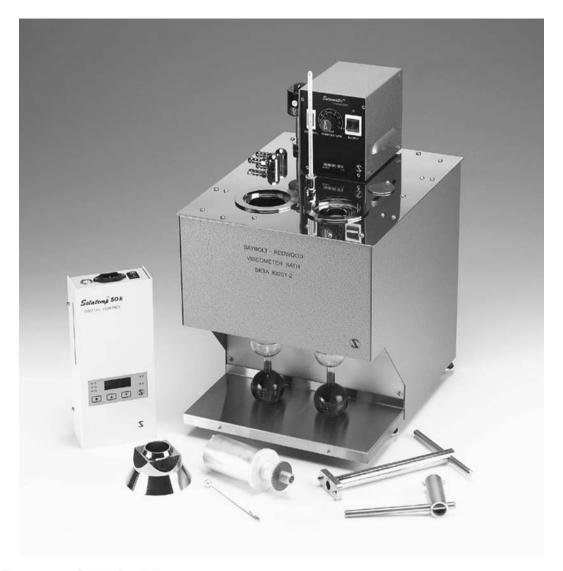
Figure 18.2 Saybolt Furol Viscometer
