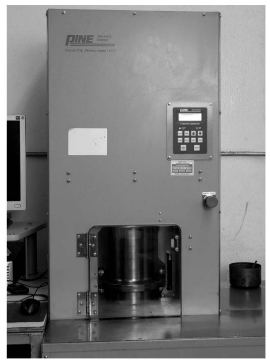
Figure 18.17 Superpave Gyratory Compactors
