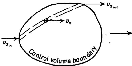
FIG. 3.17. Control volume for derivation of momentum equation.
