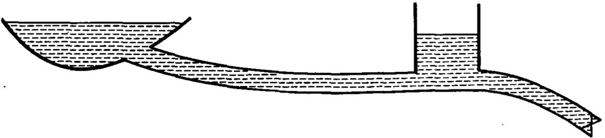
FIG. 10.18. Surge tank on a long pipeline.
