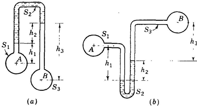
FIG. 2.9. Differential manometers.
