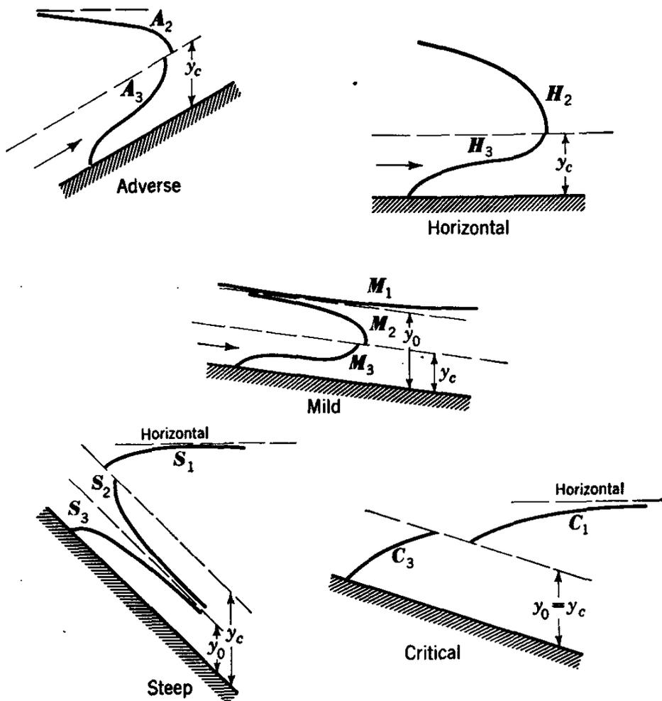
FIG. 11.11. The various typical liquid-surface profiles.
