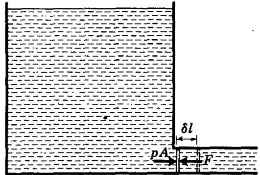
FIG. 3.9. Work done by sustained pressure force.
