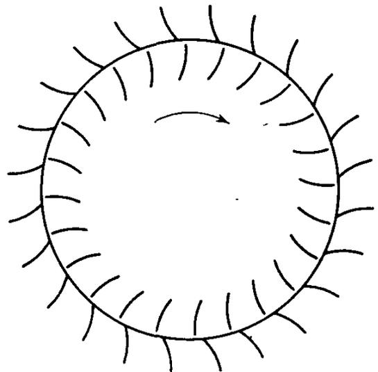
FIG. 8.4. Moving cascade within fixed cascade.
