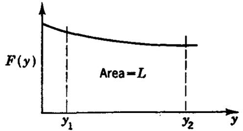
FIG. 11.10. Numerical integration of gradually varied flow equation.
