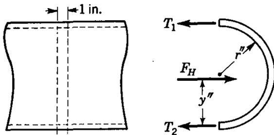
FIG. 2.32. Tensile stress in pipe.
