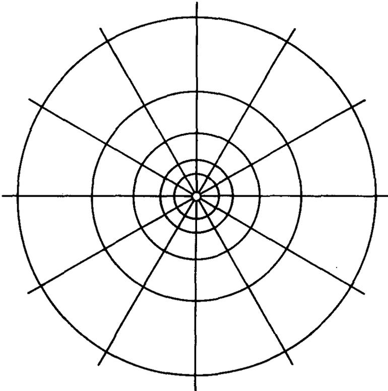
FIG. 7.26. Flow net for source or vortex.
