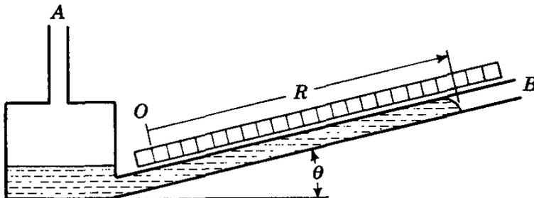
FIG. 2.13. Inclined manometer.
