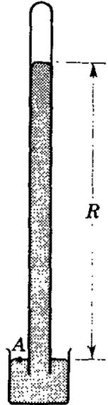
FIG. 2.7. Mercury barometer.
