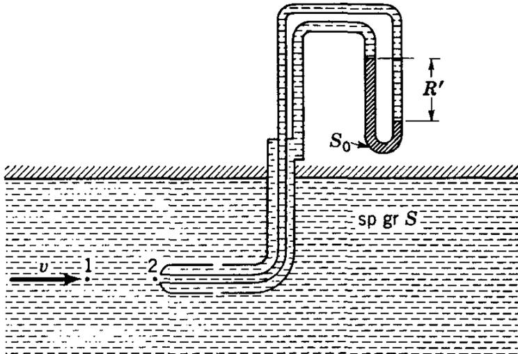
FIG. 9.7. Pitot-static tube.
