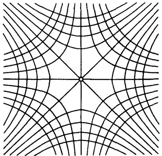
FIG. 7.24. Flow net for flow around  $90^\circ$  bend.
