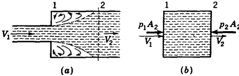
FIG. 3.33. Sudden expansion in a pipe.
