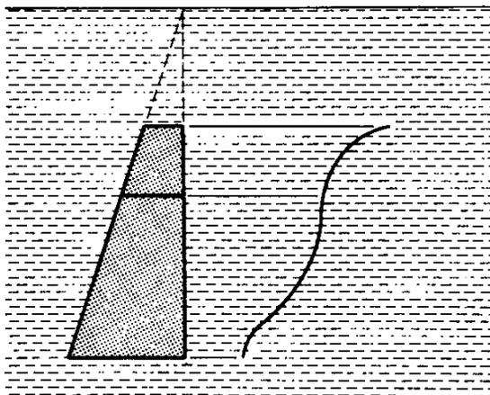
FIG. 2.28. Pressure prism for horizontal component of pressure
