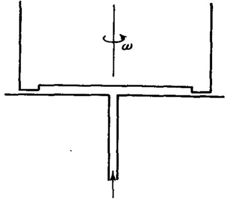
FIG. 5.40. Hydrostatic lubrication by high-pressure pumping of oil.
