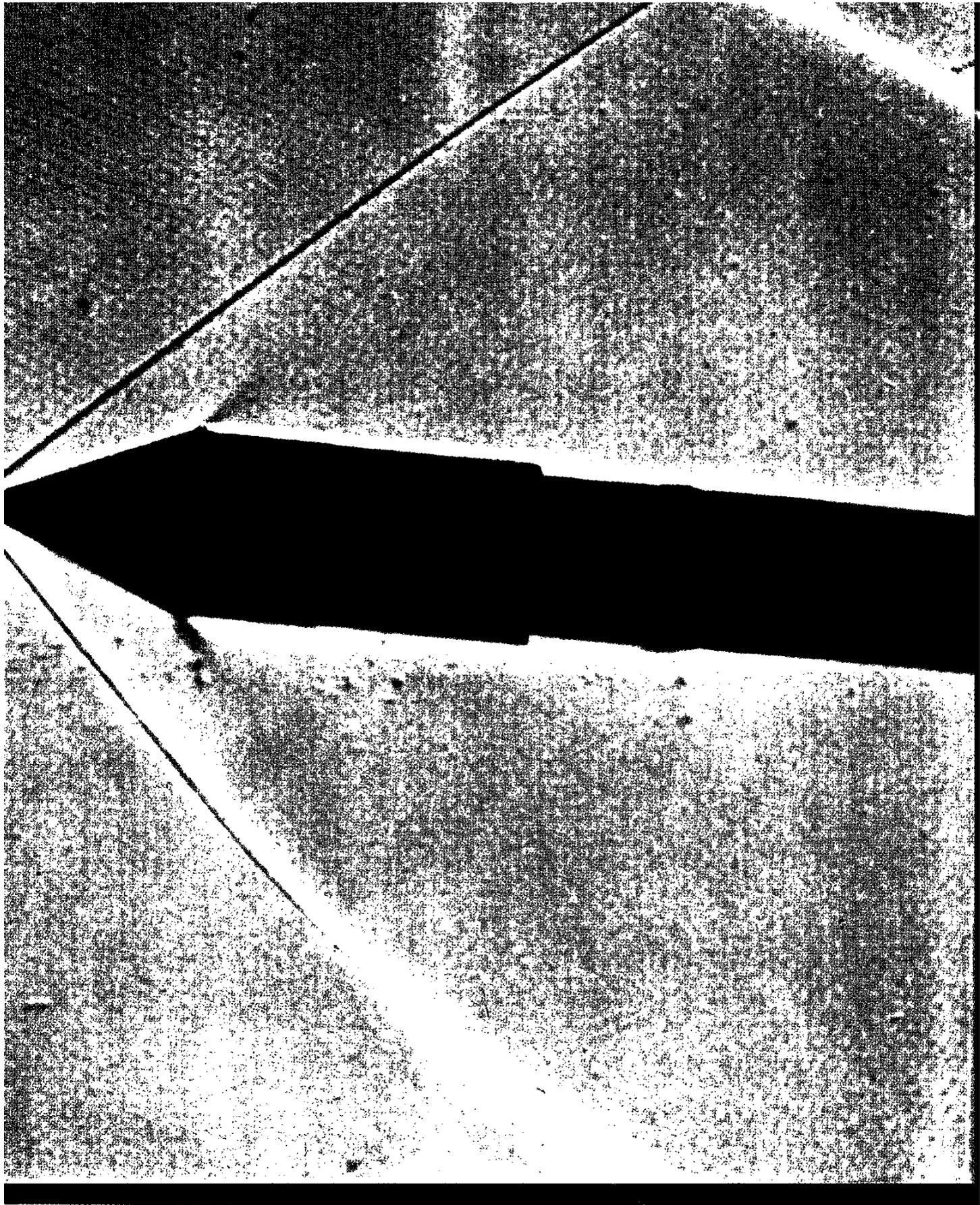
Colored Schlieren photograph of a  $22\frac{1}{2}^\circ$  half-angle wedge, Mach number 2.75, with angle of attack of  $5^\circ$ . Shock-wave interaction with wind-tunnel boundary layer shown at top. (*Aeronautical and Astronautical Engineering Laboratories, University of Michigan.*)
