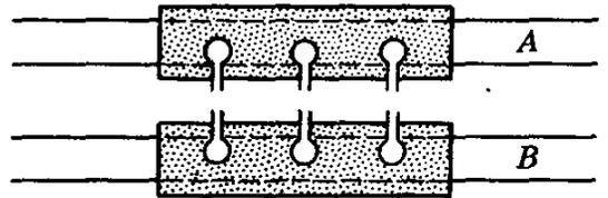
FIG. 1.3. Model for illustrating transfer of momentum.
