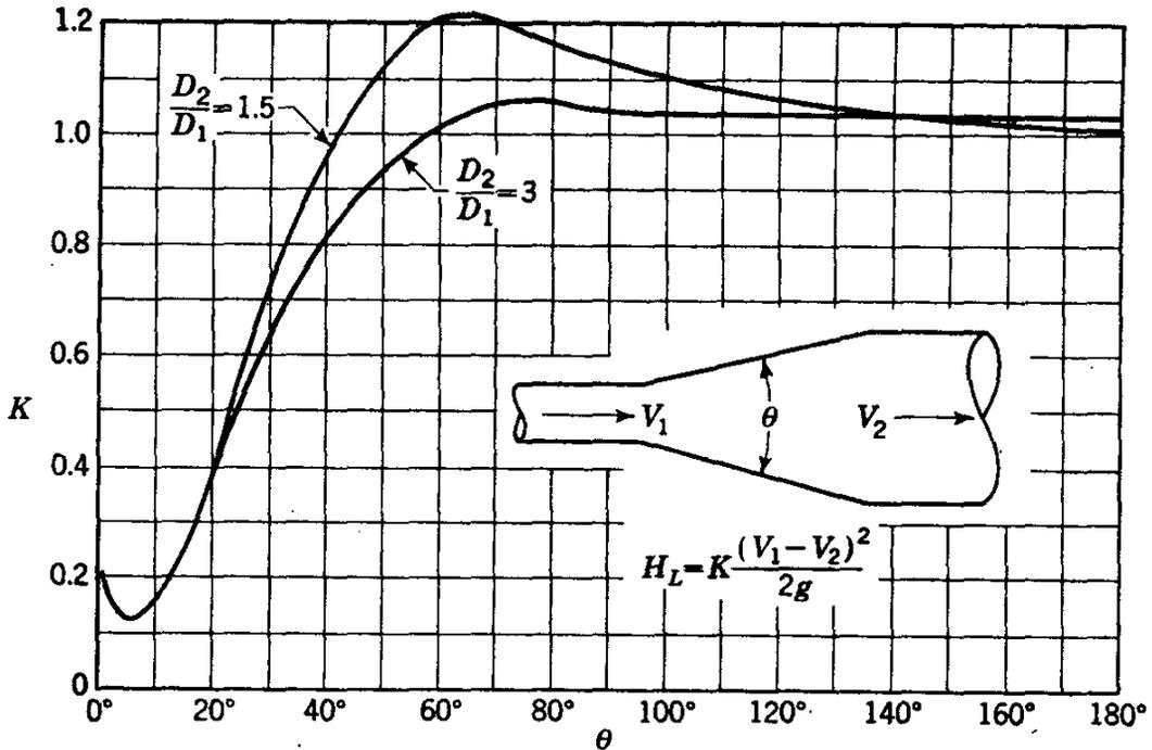
FIG. 5.36. Loss coefficients for gradual conical expansions.
