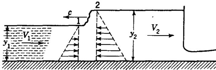
FIG. 11.16. Positive surge wave in a rectangular channel.
