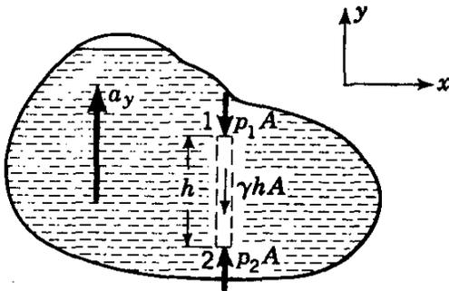
FIG. 2.16. Vertical acceleration.
