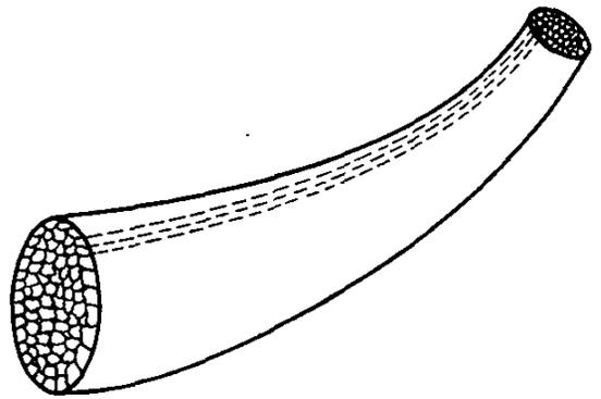
FIG. 3.5. Collection of stream tubes between fixed boundaries.
