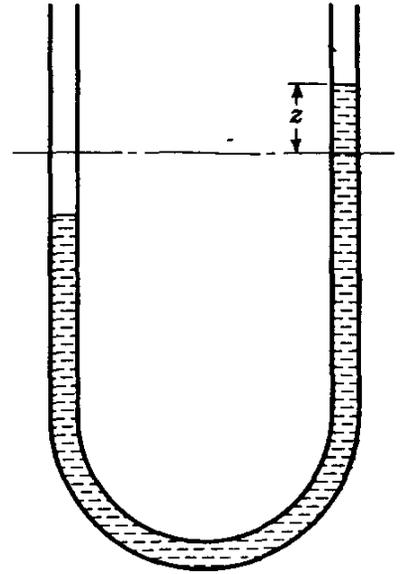
FIG. 10.13. Oscillation of liquid in a U-tube.
