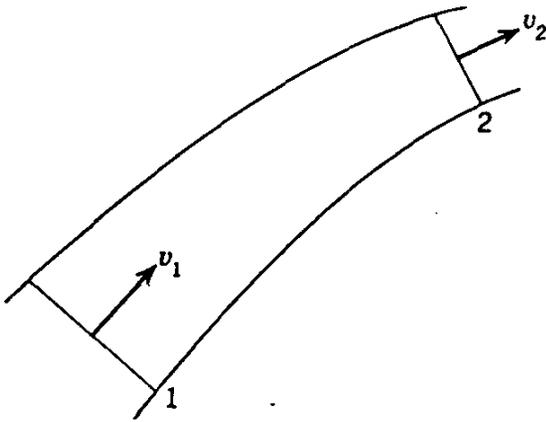
FIG. 3.4. Steady flow through a stream tube.
