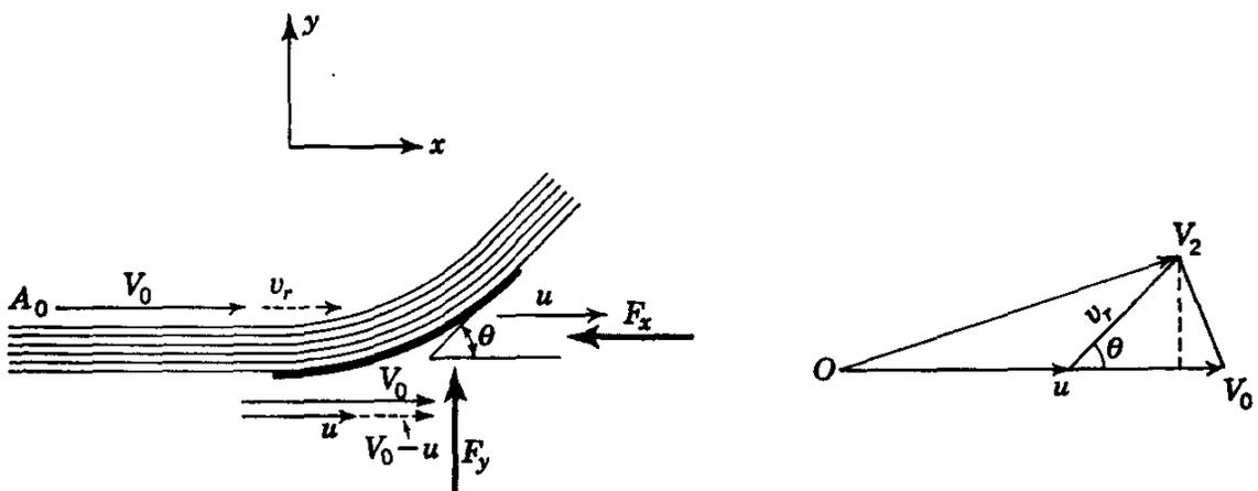
FIG. 3.28. Velocity relationships for a moving vane.
