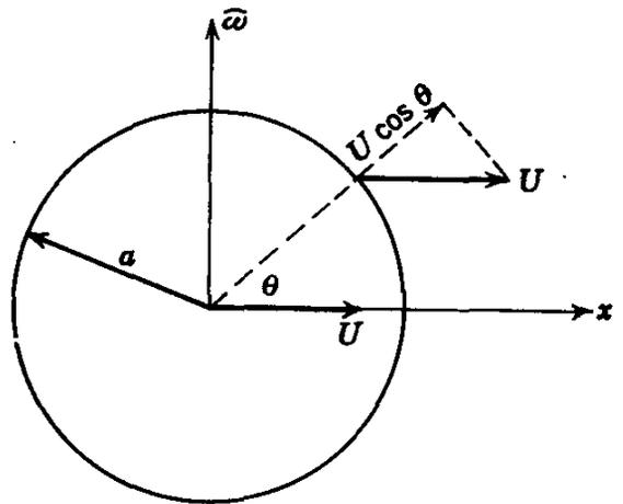
FIG. 7.21. Sphere translating in the positive  $x$ -direction.
