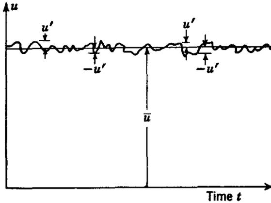
FIG. 9.36. Turbulent fluctuations in direction of flow.
