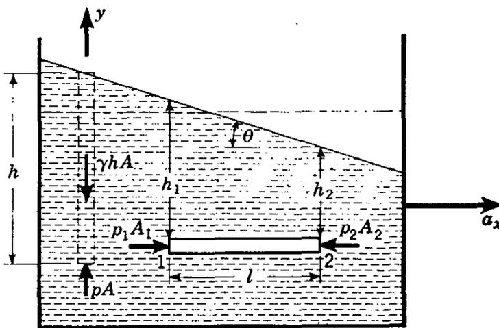
FIG. 2.14. Horizontal acceleration.
