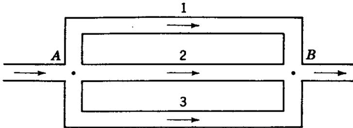
FIG. 10.7. Parallel-pipe system.
