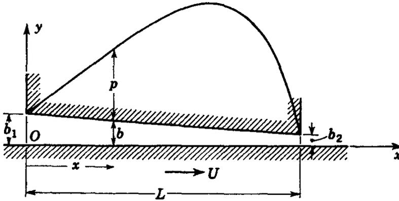
FIG. 5.38. Sliding bearing.
