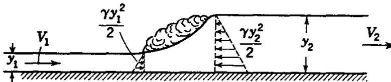
FIG. 3.34. Hydraulic jump in a rectangular channel.
