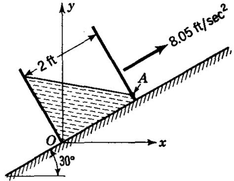
FIG. 2.17. Uniform acceleration along an inclined plane.
