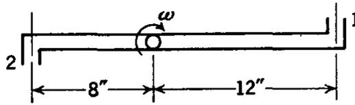
FIG. 3.39. Rotating jet system.
