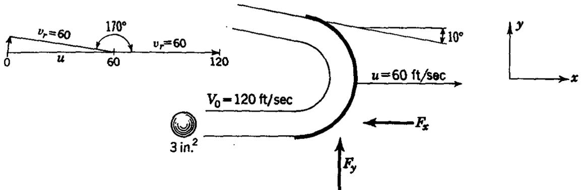
FIG. 3.30. Vector diagram for jet on moving vane.
