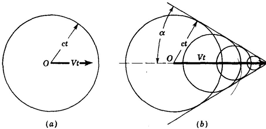
FIG. 5.26. Wave propagation produced by a particle moving at (a) subsonic velocity and (b) supersonic velocity.
