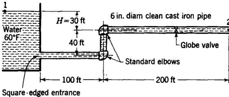
FIG. 5.37. Pipeline with minor losses.
