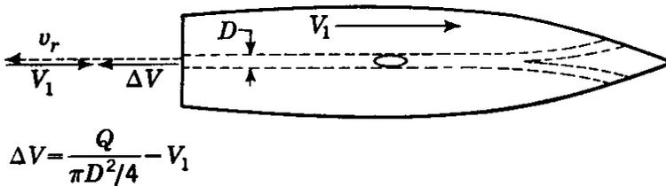
FIG. 3.23. Propulsion of boat with liquid jet.
