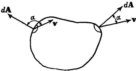
FIG. 3.3a. Notation for flow through a surface.
