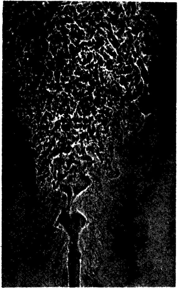
FIG. 9.15. Shadowgraph view of propane-air combustion. Flame is stabilized around  $\frac{1}{8}$ -in.-diameter spherical flame holder at bottom. Jet velocity 77 ft/sec. (Willow Run Research Center, The University of Michigan.)
