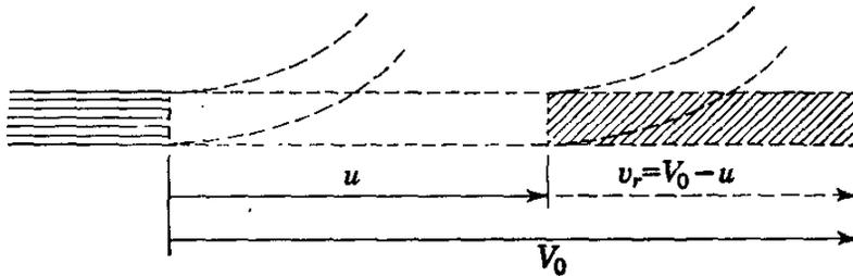
FIG. 3.29. Fluid overtaking vane in 1-sec period.
