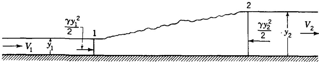
FIG. 11.4. Hydraulic jump in horizontal rectangular channel.
