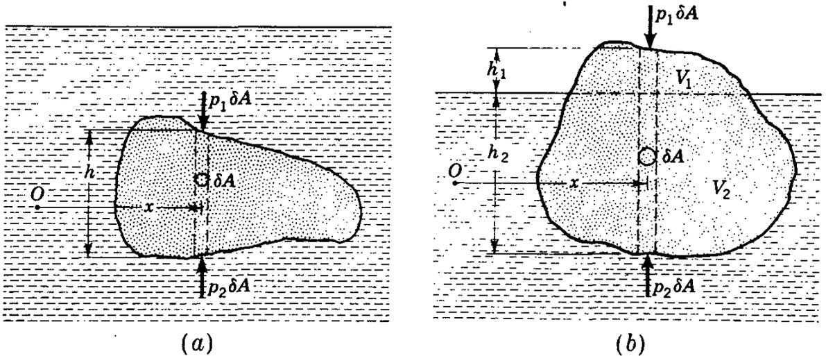
FIG. 2.34. Vertical force components on element of body.
