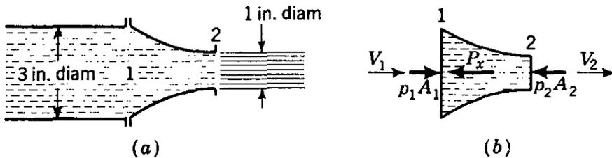
FIG. 3.20. Nozzle at the end of a pipe.
