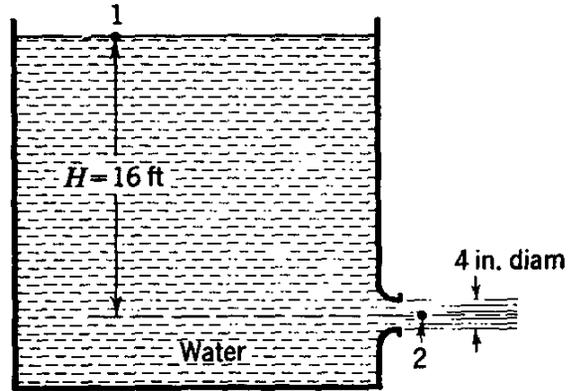
FIG. 3.12. Flow from a reservoir.
