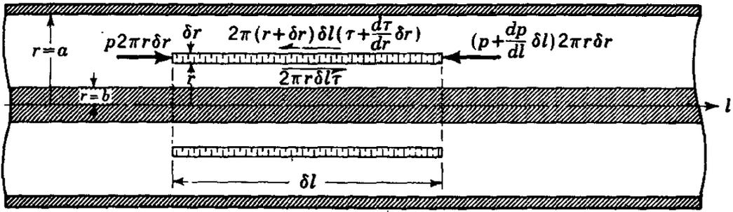
FIG. 5.11. Free-body diagram for flow through an annulus.
