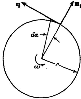
FIG. 7.4. Small fluid cylinder rotating as a solid.
