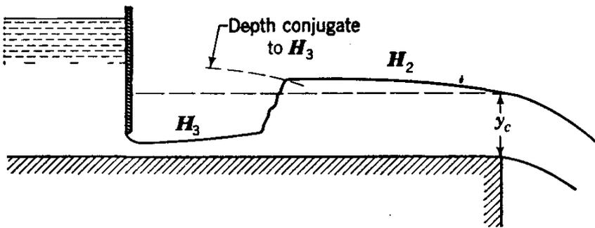
FIG. 11.13. Hydraulic jump between two control sections.
