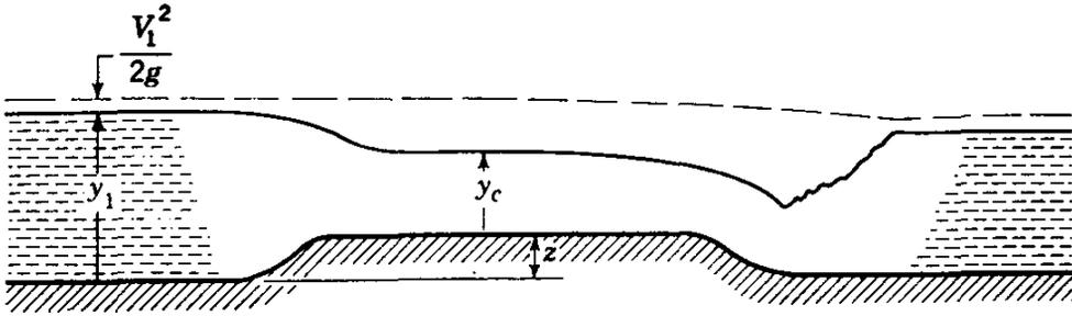
FIG. 11.15. Critical-depth meter.
