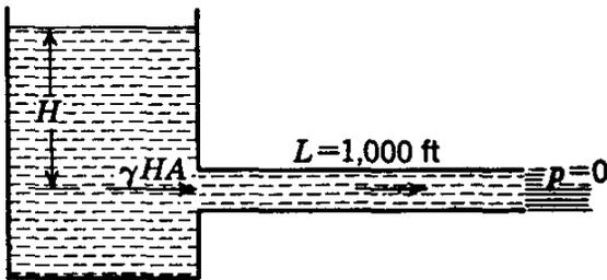
FIG. 3.36. Acceleration of liquid in a pipe.
