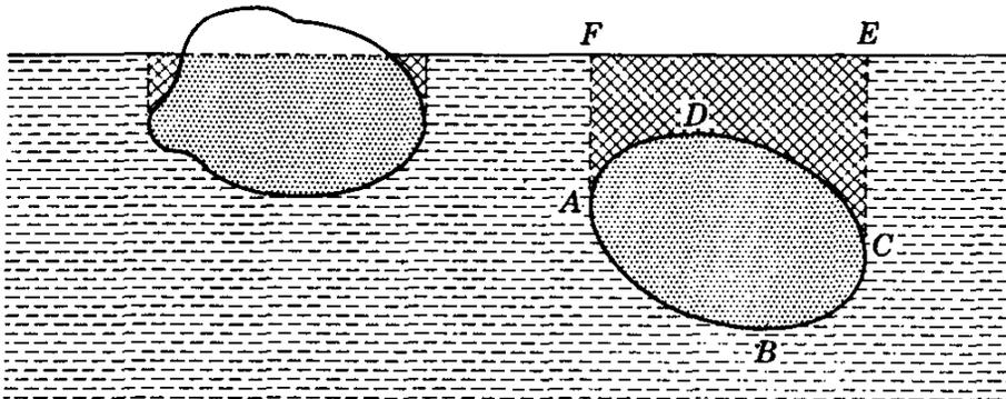
FIG. 2.33. Buoyant force on floating and submerged bodies.
