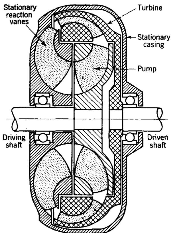
FIG. 8.33. Torque converter
