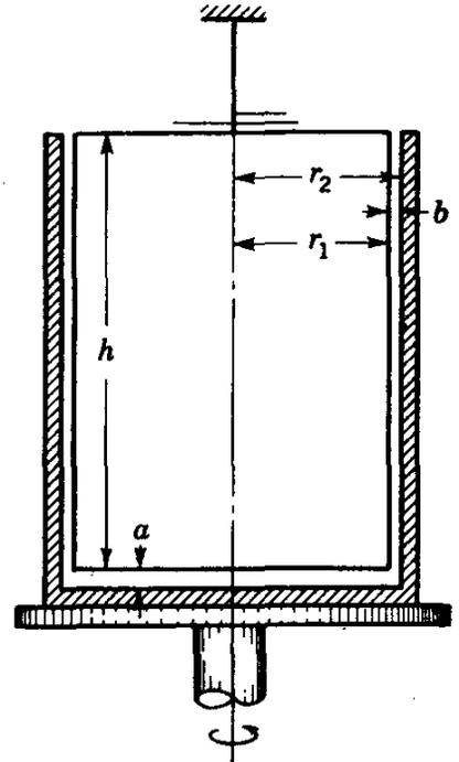
FIG. 9.37. Concentric-cylinder viscometer.
