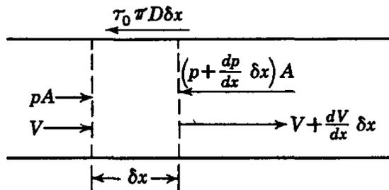
FIG. 6.4. Notation for application of momentum equation.
