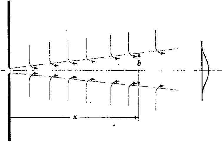
FIG. 5.15. Fluid jet issuing into same fluid medium.
