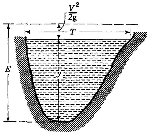
FIG. 11.8. Specific energy for a non-rectangular section.
