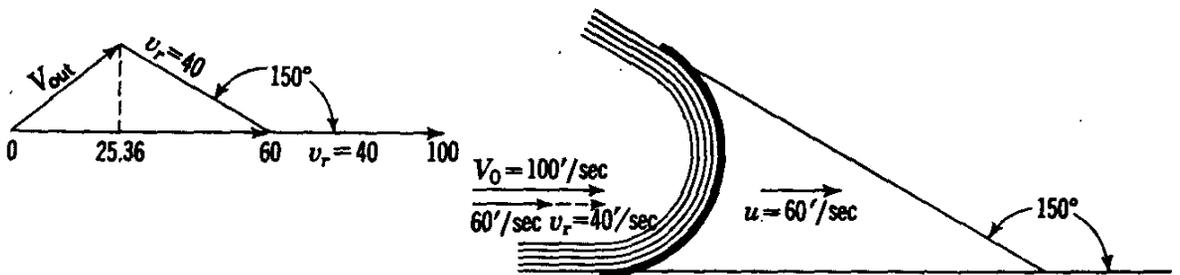
FIG. 3.31. Vector diagram for moving vane.
