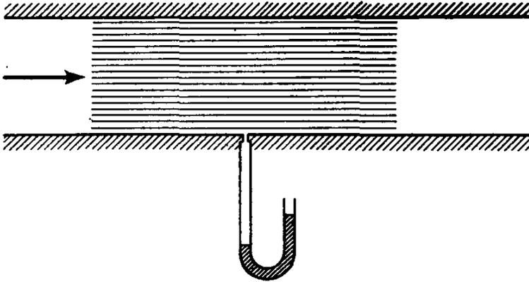
FIG. 9.1. Piezometer opening for measurement of static pressure.
