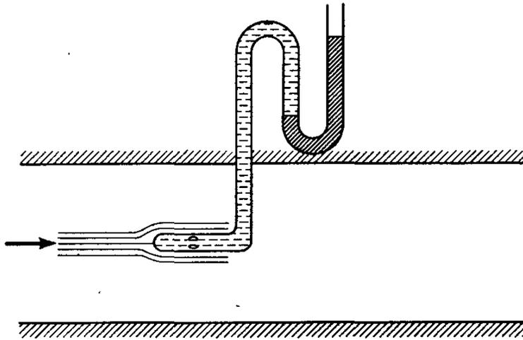
FIG. 9.2. Static tube.
