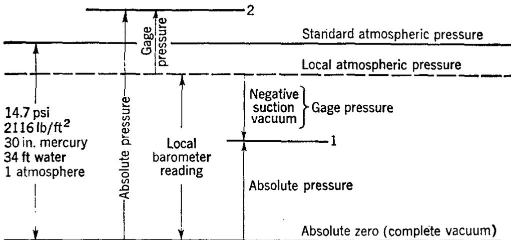
FIG. 2.6. Units and scales for pressure measurement.
