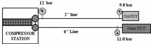
Figure 7-2: Compressed air system piping schematic
