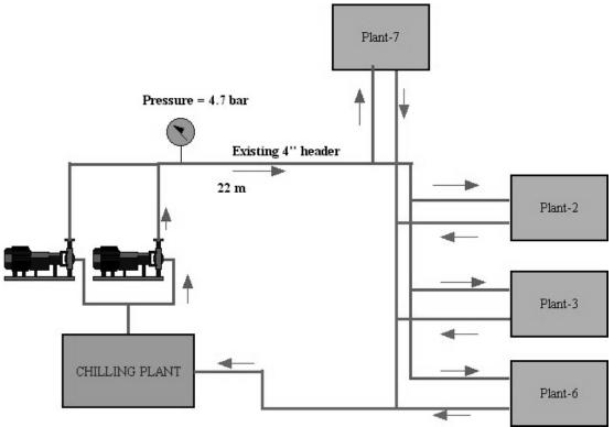
Figure 7-1: Chilled water system piping schematic
