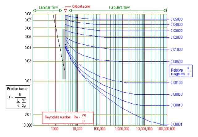
Figure 2-1: Estimation of friction factor
