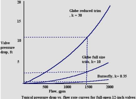
Figure 7-3: Pressure drop of Globe & Butterfly Valves
